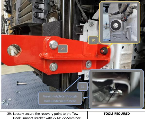
Hook Support Bracket with 2x M12x55mm hex bolts, flat washers and flange nuts.
