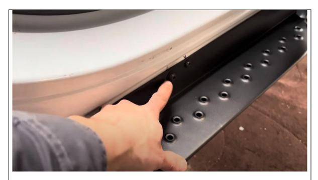
23. Fit all M6 bhcs and flat washers into the side of the slider into M6 nutserts
