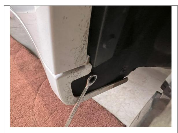
1. Remove 2 x per corner screws holding in felt liner. 8 screws in total
