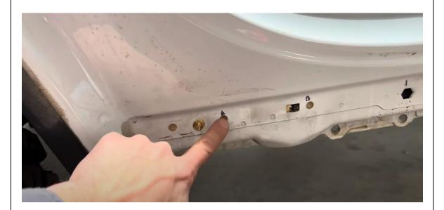
7. Starting from the rear skip the first two holes and then mark the next 2 and open the holes to 9mm or imperial equivalent to suit M6 nutserts, skip the hex hole and the open the next hole. Basically, you want the nutsert to just barely fit into the hole.
