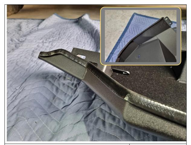
42. Fit the supplied lengths of pinch weld to the top flanges of the centre plate and both wings.
