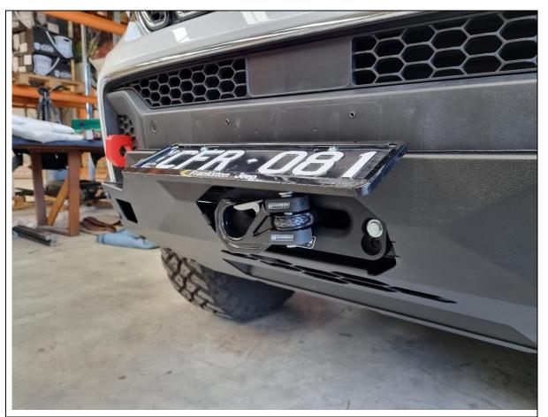
58. Fit the number plate onto the vehicle. You can either fit the number plate back on the original mounting location on the number, or to the holes on the centre plate of the Pre Runner.
