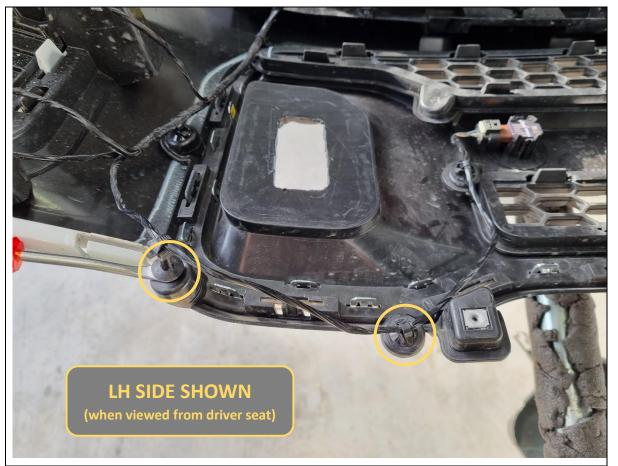
33. Unclip the wiring loom from the locations shown and tuck the loom up and out of the way.
