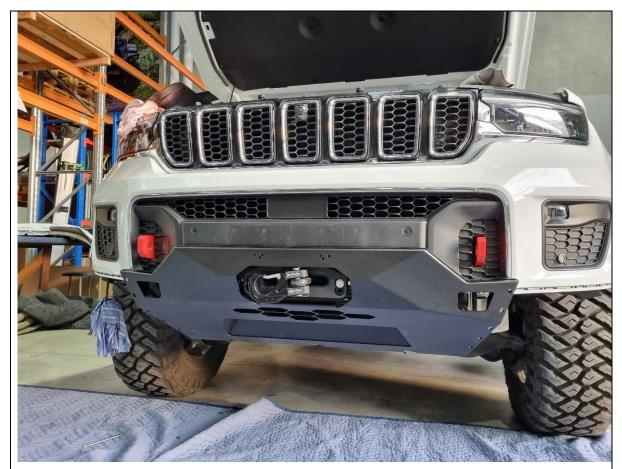
45. Hold the centre plate up to the vehicle, over on top of the bumper.
