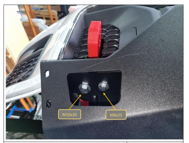
46. Loosely secure the top of the plate to the mount bracket using 1x M8x25 hex bolt and washer, and 1x M10x20 hex bolt, flat washer and flange nut. Repeat for other side.
