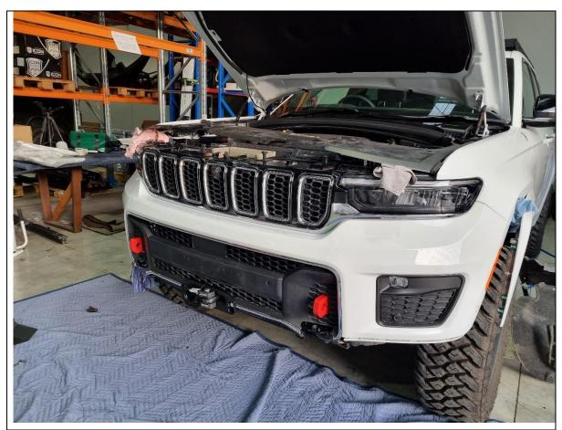
40. Fit the bumper back onto the vehicle. Reconnect all looms and washer hose lines.
