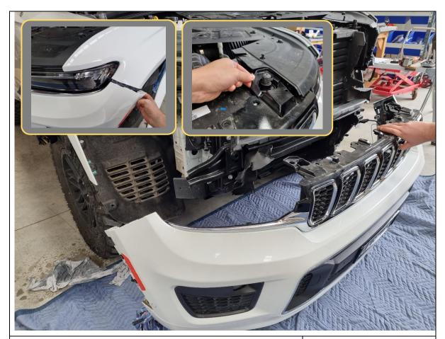
16. Remove the bumper by releasing the clips on either side and lifting the top flap of the grille over the bonnet rubber stops.
