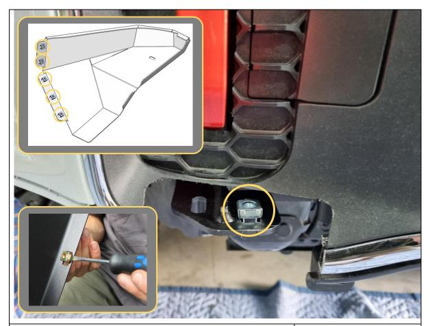
42. Install 1x M8 cage nut in the rectangular slot on the mount. Repeat for other side.
