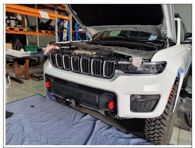
39. Fit the bumper back onto the vehicle. Reconnect all looms and washer hose lines.
