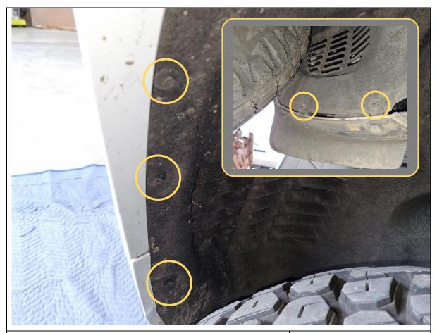
8. On each side, remove 5x 8mm hex head screws securing the wheel arch liner to the bumper.
