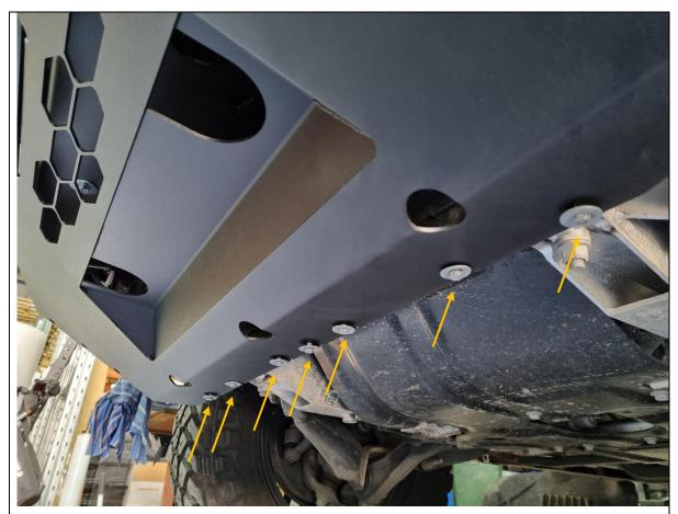
46. Loosely secure the bottom of the plate with 7x 10mm hex bolts retained from Step 6.
