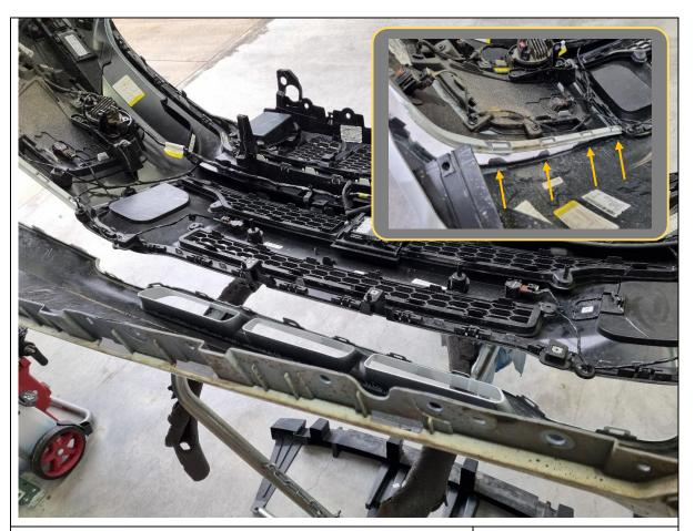
31. Unclip the lower half of the bumper from the main section.
