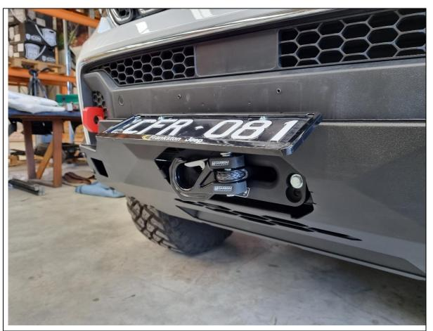
56. Fit the number plate onto the vehicle. You can either fit the number plate back on the original mounting location on the number, or to the holes on the centre plate of the Pre Runner.
