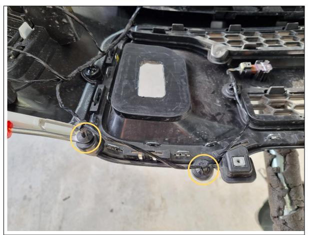
32. Unclip the wiring loom from the locations shown and tuck the loom up and out of the way.
