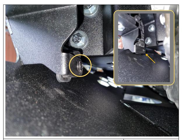
47. Secure the bumper to the centre plate by re-using the T20 torx screw from Step 29. Gain access from the opening on the side. Repeat for other side.
