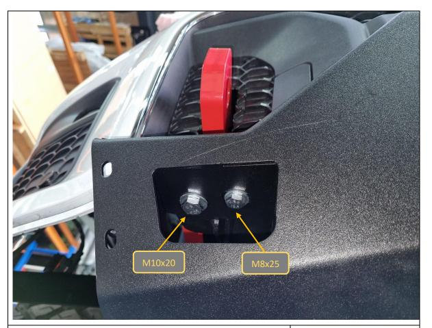
45. Loosely secure the top of the plate to the mount bracket using 1x M8x25 hex bolt and washer, and 1x M10x20 hex bolt, flat washer and flange nut. Repeat for other side.
