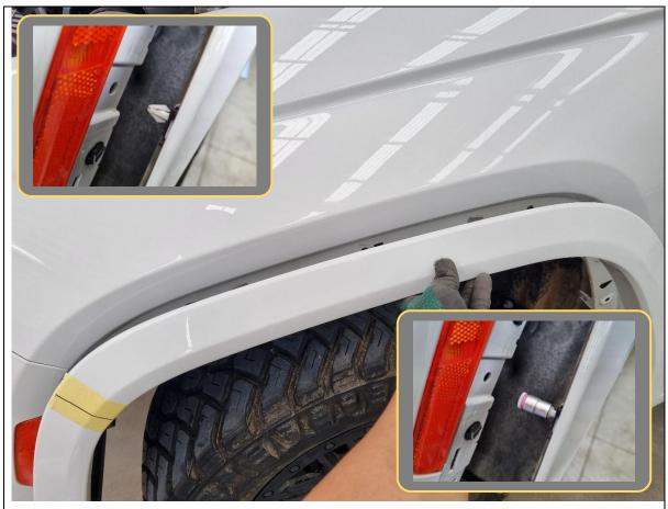
18. Pull and release the clips retaining the flare to the bumper + quarter panel.
