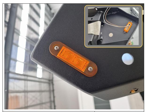
58. Bolt the supplied LED AutoLamps 7922 side marker light to the outer end of the bar using 2x M3x12 pan head screws, flat washers and hex nuts.
