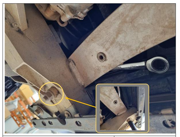
144. Additional reinforcement is required for the bash plate. Remove 2x 18mm hex nuts (1x per side) on the underside of the frame. Use an 18mm spanner to reach in access the bolt head on top of the frame member.
