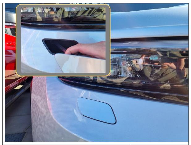
22. If headlight washers are equipped, pull out the plastic cover cap and unclip it from the plastic washer stem.
