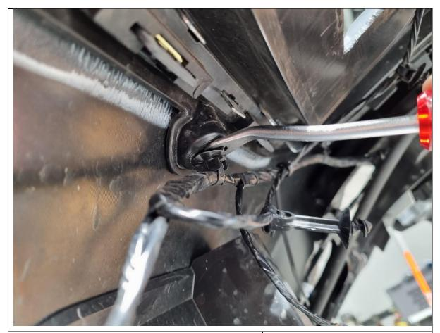
28. Unclip the loom behind the marked area and secure to the side and out of the way with cable ties.
