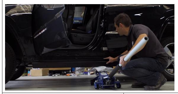
5. Using a jack lift the slider up to body of the Jeep. Line it up centrally front to back. See pull out picture above showing cut outs lined up with large oval holes in body. Make sure the laser cut arrow in slider faces forward
