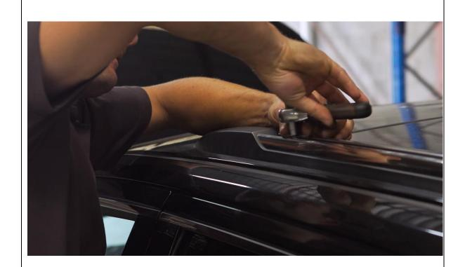
Remove factory rails on both sides. 4 screws in each.
