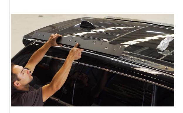
5. Lift steel rail onto roof ash shown. Repeat for other side TOOLS REQUIRED
