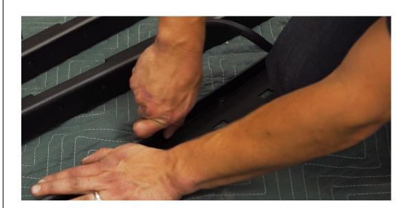
3. Fit Pinch weld to short edge of roof rails. Trim excess off with side cutters
