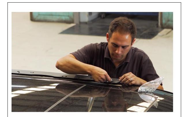
6. Fit Rails to roof with M6 Hex bolts and mud guard washers. 6 per side.
