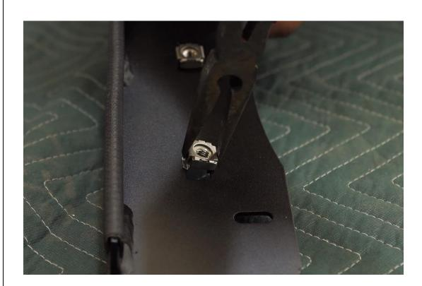
4. Fit nutserts as shown in both rails (6 per rail). You can use needle nose plyers or screwdriver to push one end of cage in from side
