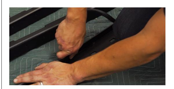
5. Fit Pinch weld to short edge of roof rails. Trim excess off with side cutters
