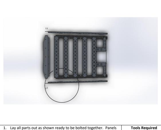
1. Lay all parts out as shown ready to be bolted together. Panels are labeled with numbers 1-5, with 1 being towards the front. As can be seen, the entire rack is dove tailed to suit Jeeps roof. Front is wider than back.
