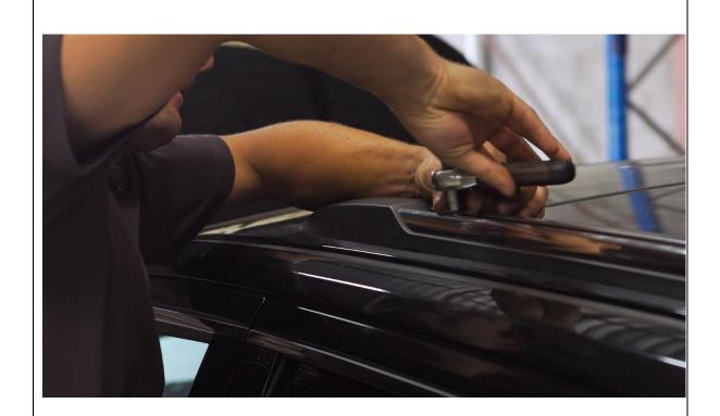
2. Remove factory rails on both sides. 4 screws in each. Once all screws have been removed pull forward then lift.
