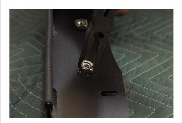
6. Fit nutserts as shown in both rails (6 per rail). You can use needle nose plyers or screwdriver to push one end of cage in from side
