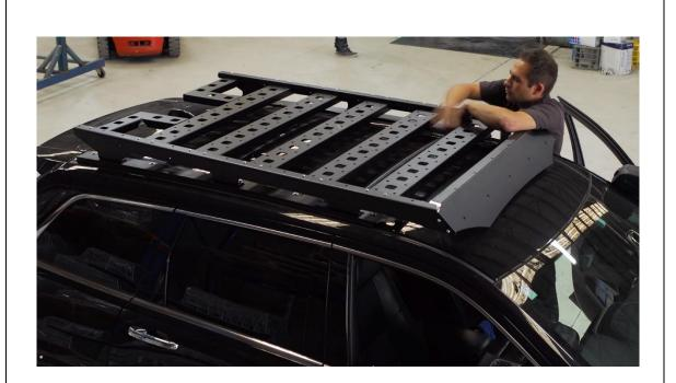
16. Loosely fit M8 bolts spring washers and washers through rack into nutserts fitted to steel rail
