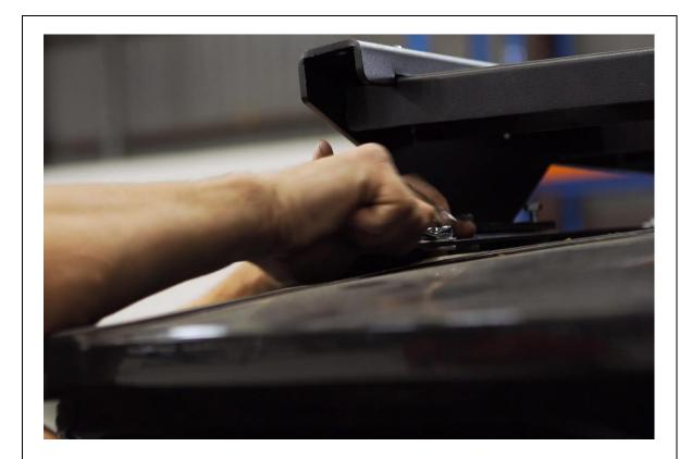
17. Position rack, and ensure all fasteners are threaded in, then torque down each M8 and M6 fastener
