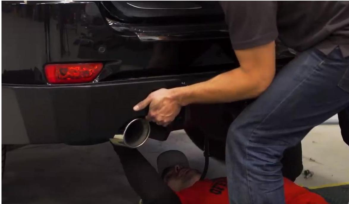
17. With the help of that friend of yours, lift the bar onto the vehicle while one lies underneath and starts all the bolts. Here you will also put the nut plates into the chassis and secure with M16 fasteners.
