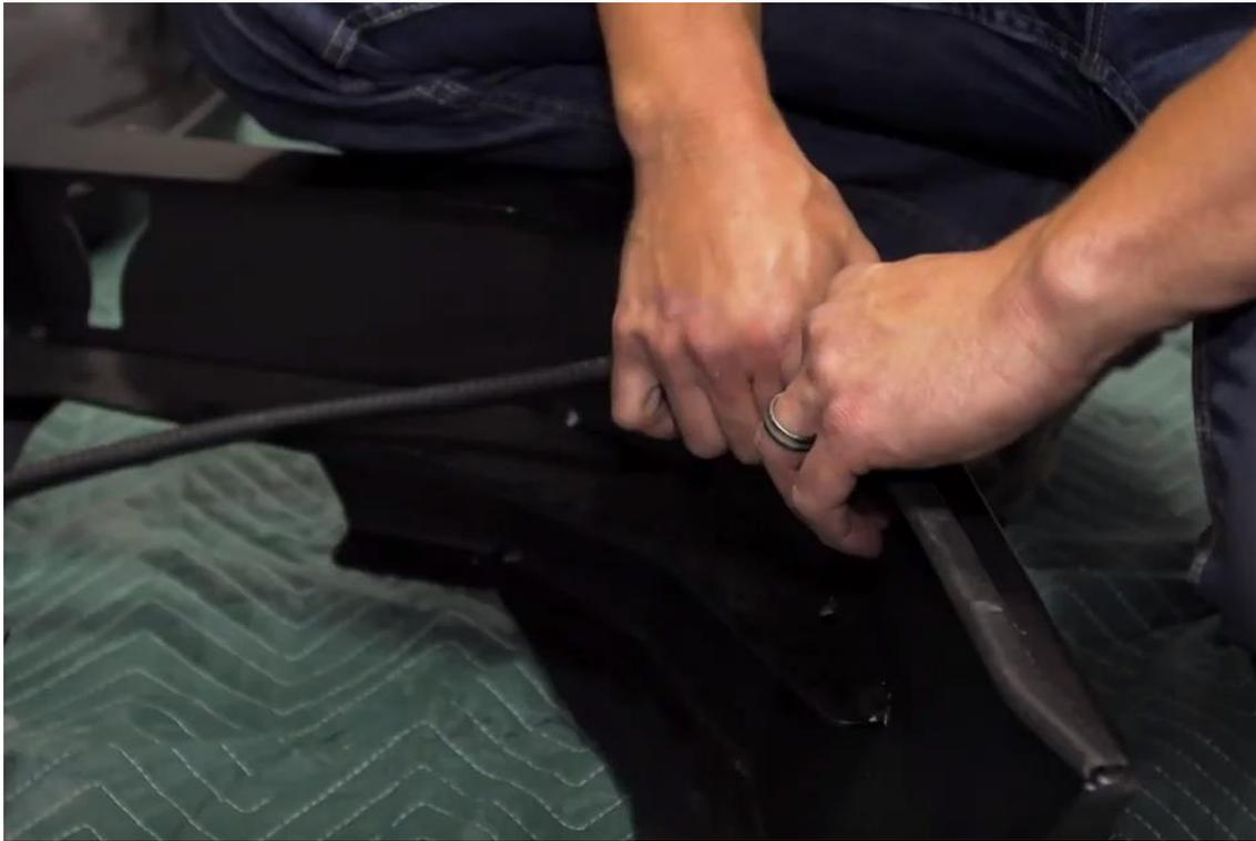
16. Install pinch weld on top and side edges of steel rear bar. Trim extra length off with side cutters
