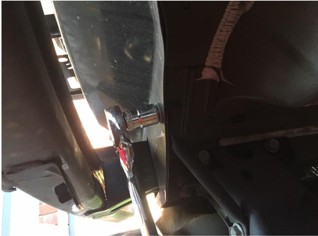
10. Remove Tow point on LHS of Jeep using 18mm and 23mm spanners or sockets
