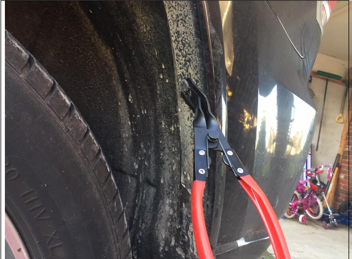
3. Pry off plastic rivets on both sides
