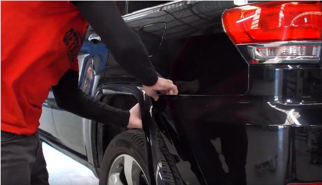
7. Pull flare aside with use of flat screw driver on each clip to release from body. Repeat for other side
