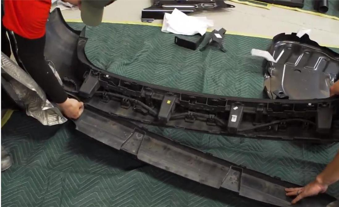
14. Split lower section of bumper from upper section. Use pry tool, flat head screw driver and T20 Torx bit
