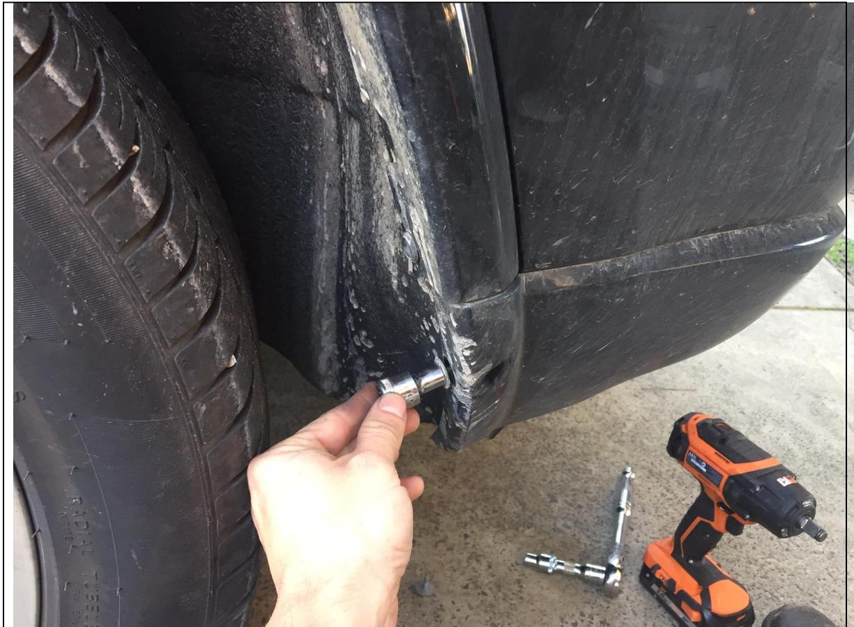
2. Remove lower bolt on both sides with 10mm spanner or socket
