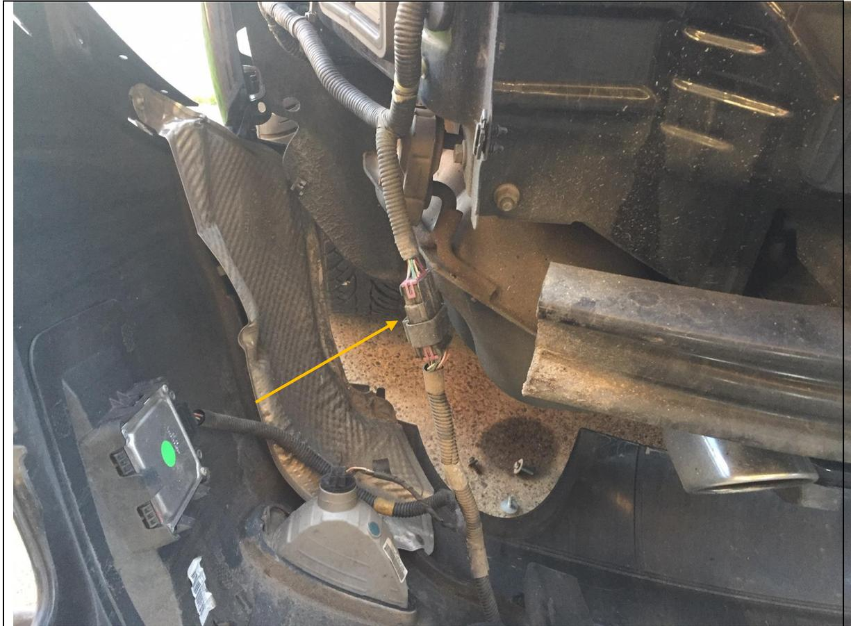
9. Unplug loom for rear fog lights and rear parking sensors if fitted
