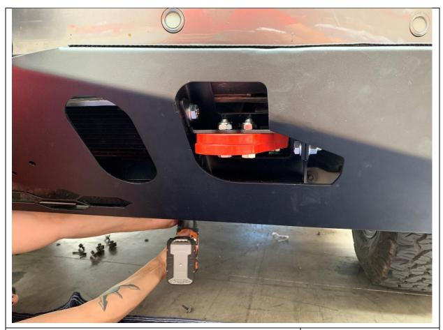
17. Using the factory M6 bolts secure through the bottom of the Pre runner centre plate
