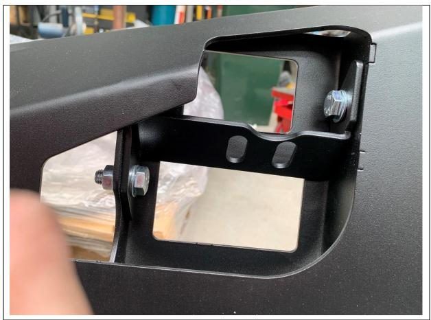
13. Fit Pre runner mounts as shown with M10 x 30 bolts, washers and flange nuts
