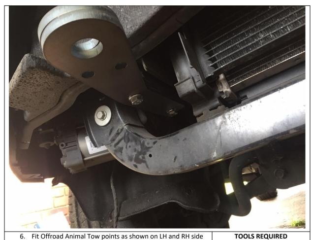
6. Fit Offroad Animal Tow points as shown on LH and RH side with M10x80 bolts directly into frame of Jeep. Torque down bolts. Be aware if fitting a nudge bar you may need to later loosen these bolts to realign these tow points to suit the nudge bar.
