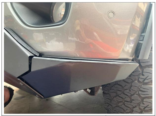
20. Position the wings to have the smallest gap possible between wings and centre. Torque up bolts
