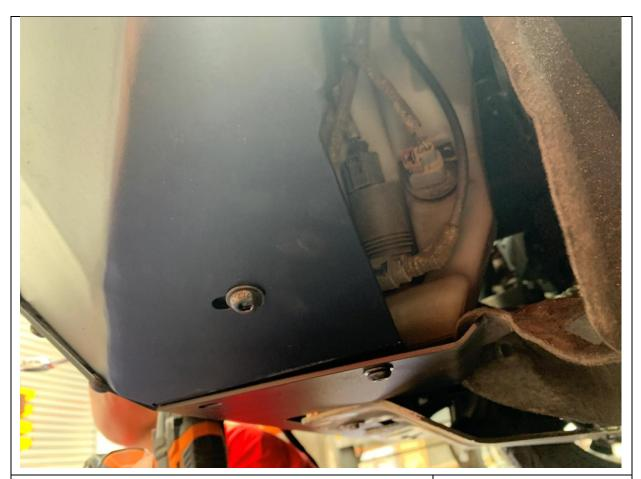
21. Fit Bolt through wing into support bracket
