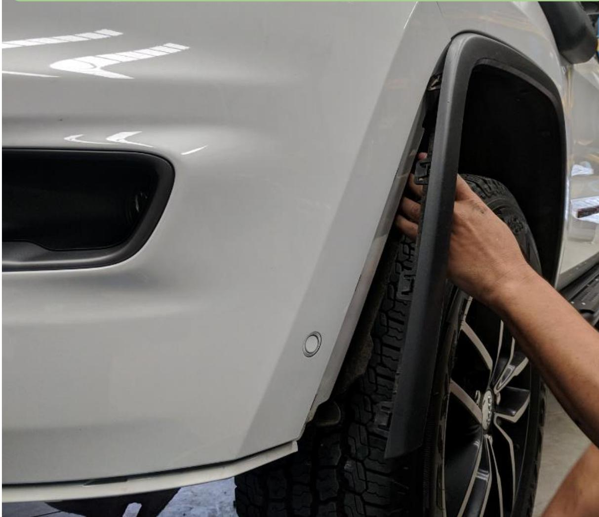
17. Pull factory flare away from bumper, using a flat head screwdriver release at least 2 of the push in clips on top edge being careful not to break them as you pull the flare away from the body
