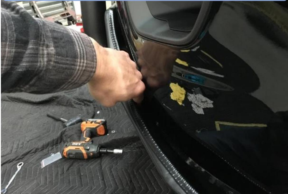
53. Fit wings to center panel, as shown. Fit top bolt first by putting bolt through front face and using your fingers behind to hold the flange nut.
