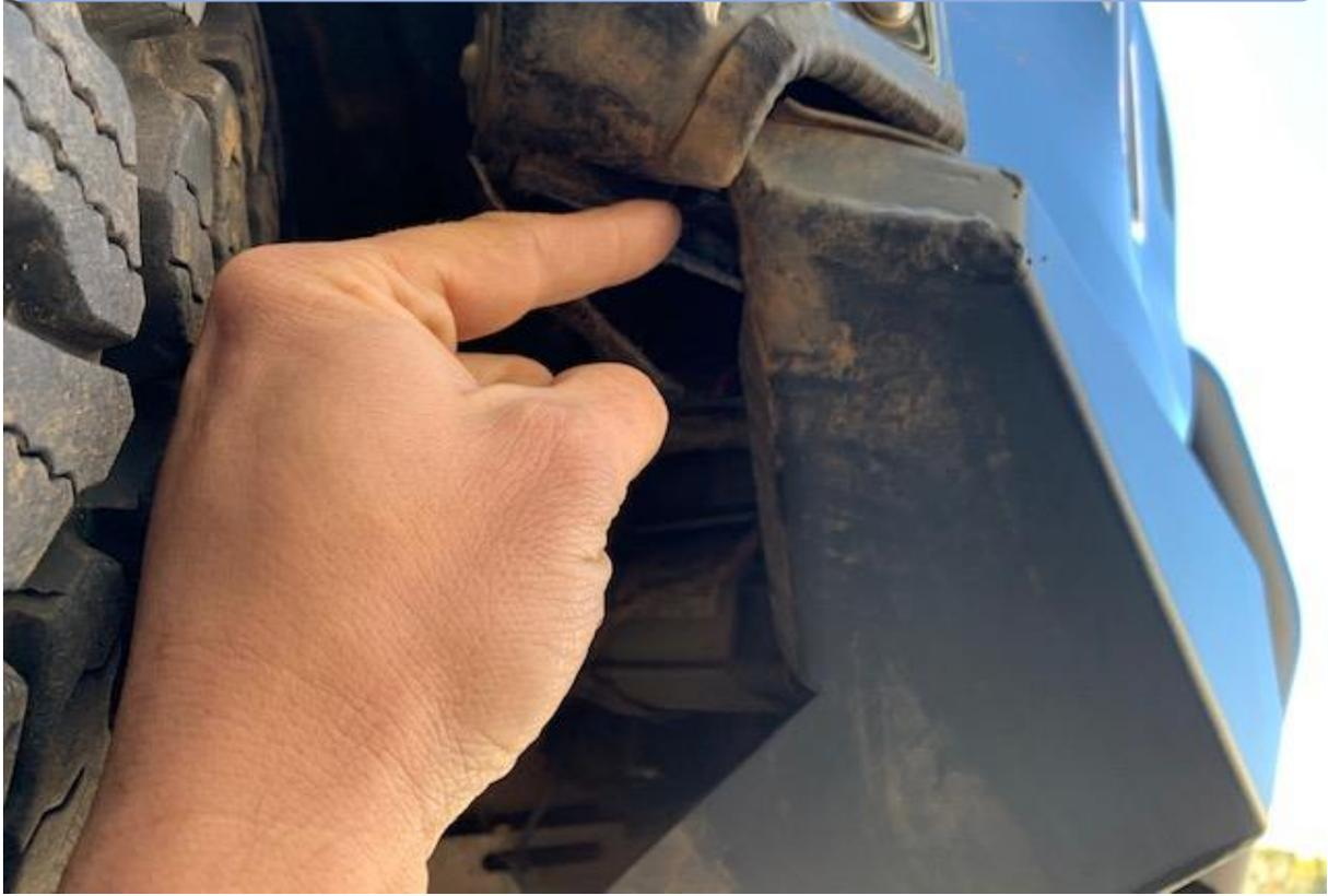
69. If your Jeep is equipped with parking sensors and they are going off as they see the new bumper you can fix this by adding a cable tie to the slot that originally holds the lower air dam being pointed to in the picture.
