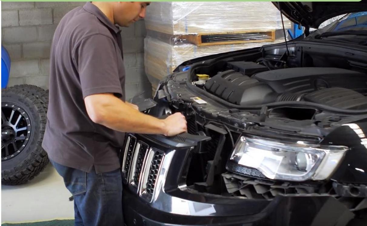
20. Lifting the top section ever so slightly you can release clips holding in the top section and pull the remainder of the bumper away
