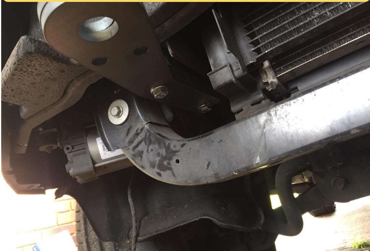
7. Fit Offroad Animal Tow points as shown on LH and RH side with M10x80 bolts directly into frame of Jeep.
