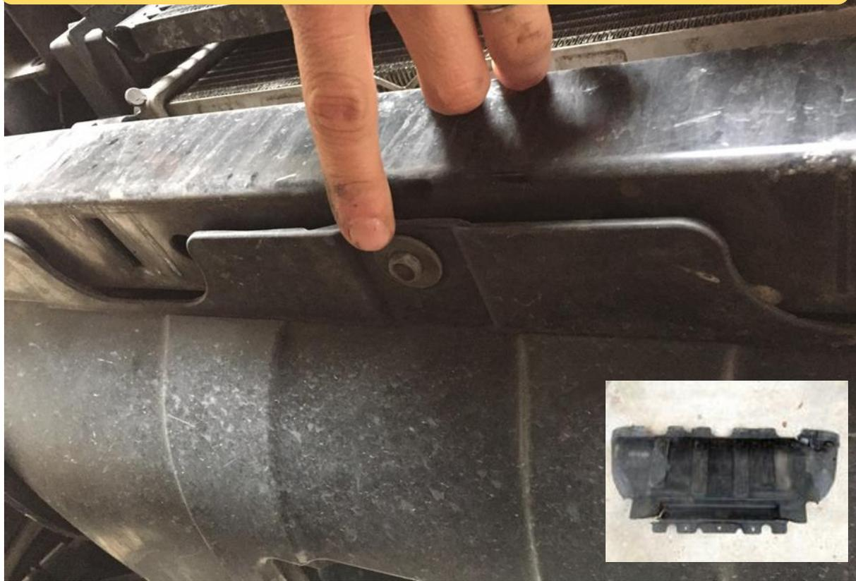
3. Remove factory Lower Radiator Cover. 3x M6 bolts on front and 2x M8 bolts on back. Use 10mm socket or spanner for front and 13mm for rear
