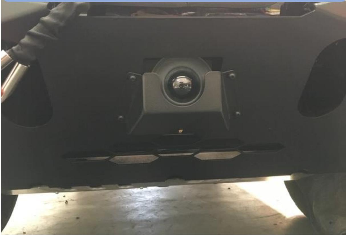
64. Secure ACC cover to main plate with M6 x 16 button head cap screws washers and flange nuts
