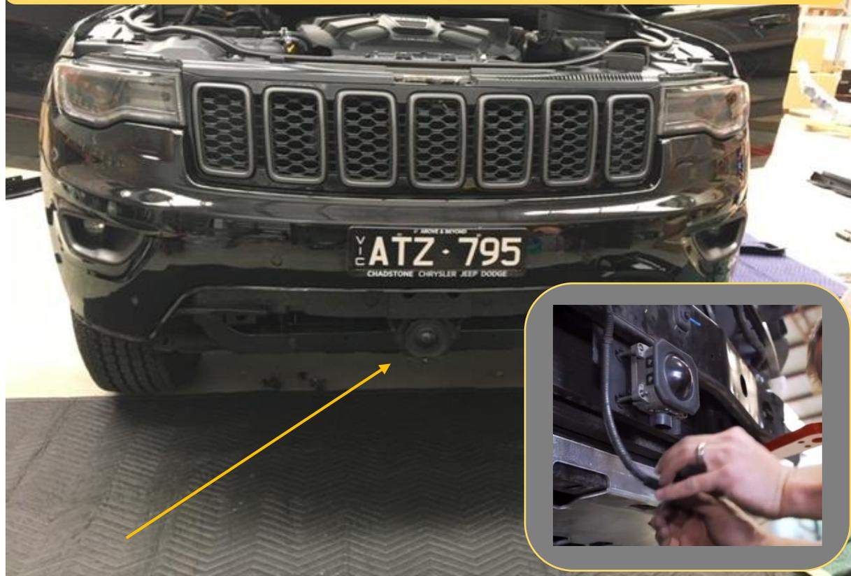
9. If Adaptive cruise control is fitted, unplug loom and pull sensor off the mounting posts.
