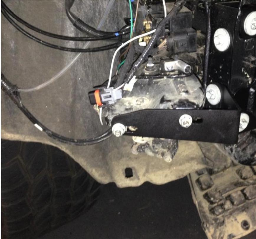
27. If vehicle is fitted with Air Suspension, fit Air suspension bracket B-0087 as shown to secure the suspension compressor.
