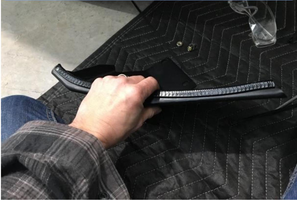
52. Fit pinch weld to top edge of wings like shown
