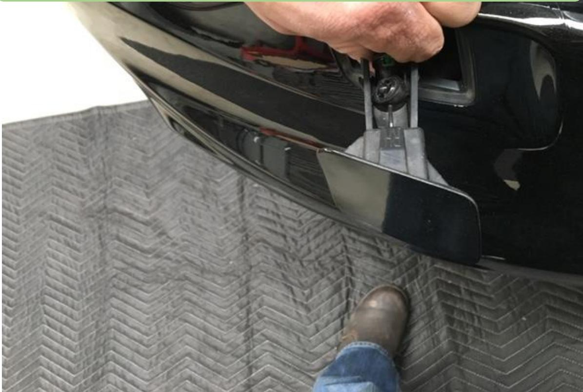
18. Pull headlight washer out by hand, and detach retaining clips allowing mechanism to retract and remove outside panel
