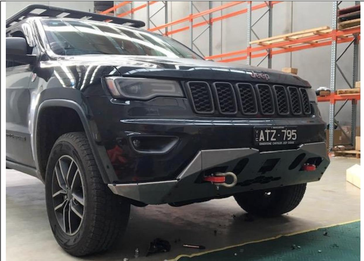
70. Fit logo plate to bumper. If fitting nudge bar hold off until that is on before doing this step.
