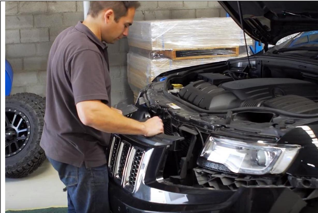
12. Lifting the top section ever so slightly you can release clips holding in the top section and pull the remainder of the bumper away
