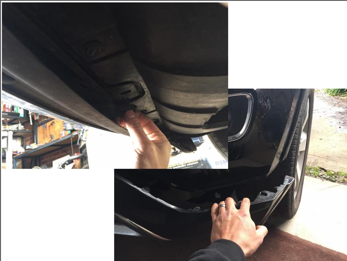
1. First step is to remove the lower air damn fascia. To do this climb under your Jeep and remove all 5 quarter turn clips by hand. Two are tucked up high in each corner and 3 in the middle
