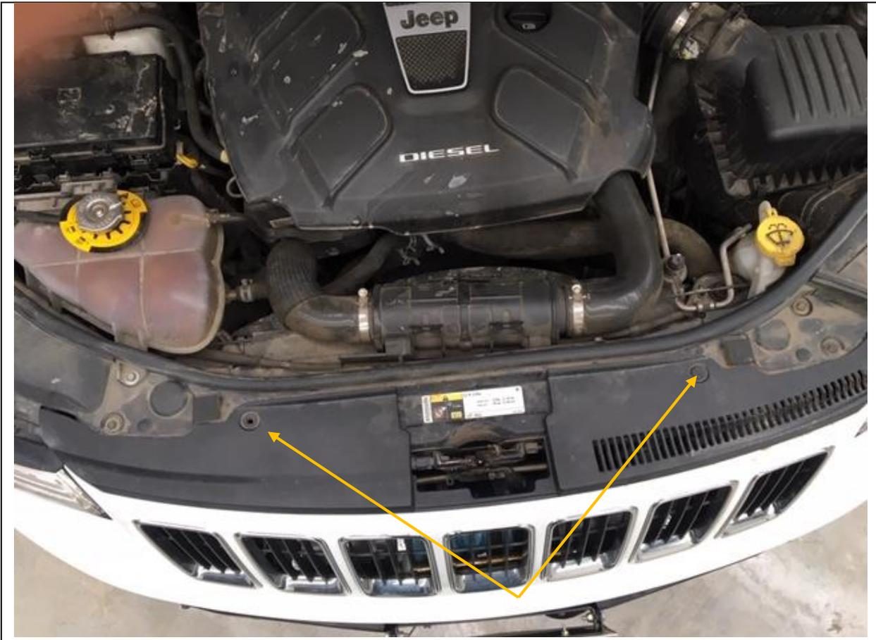
7. Next step is to remove the rest of the front bumper. Start with bonnet/hood open and pry out two clips shown with trim tool or flat head screw driver
