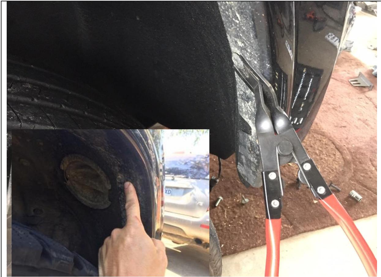
8. At the wheel arch on both sides you will need to pry out 2 plastic rivets. You can also drill out the centre of the rivet if you're struggling to pry it out.
