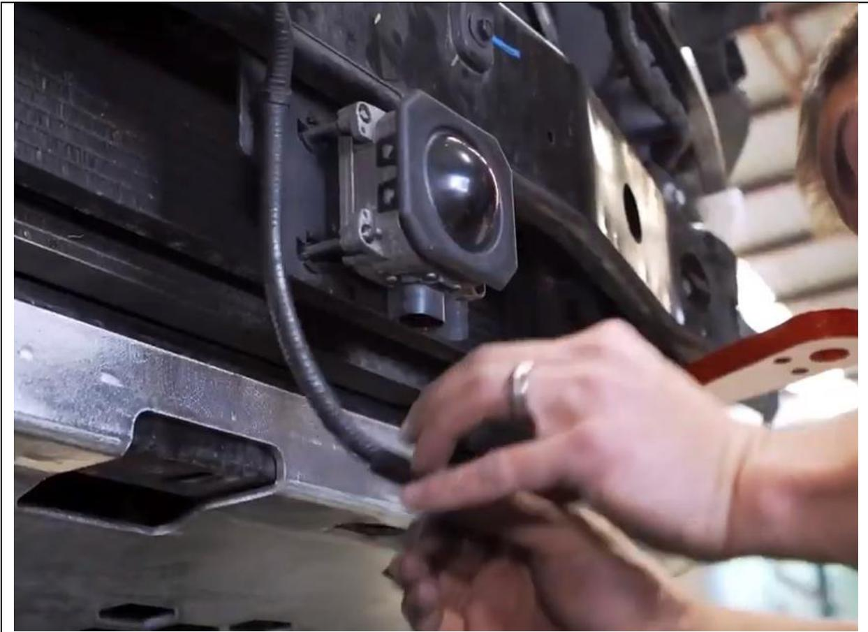
18. If Adaptive cruise control is fitted, unplug loom and pull sensor off posts
