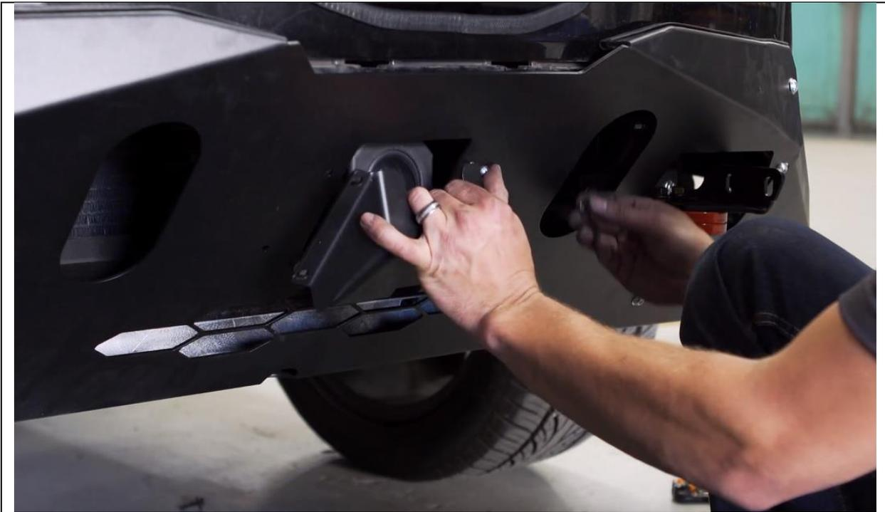
36. Secure ACC cover to main plate with M6 x 16 button head cap screws washers and flange nuts
