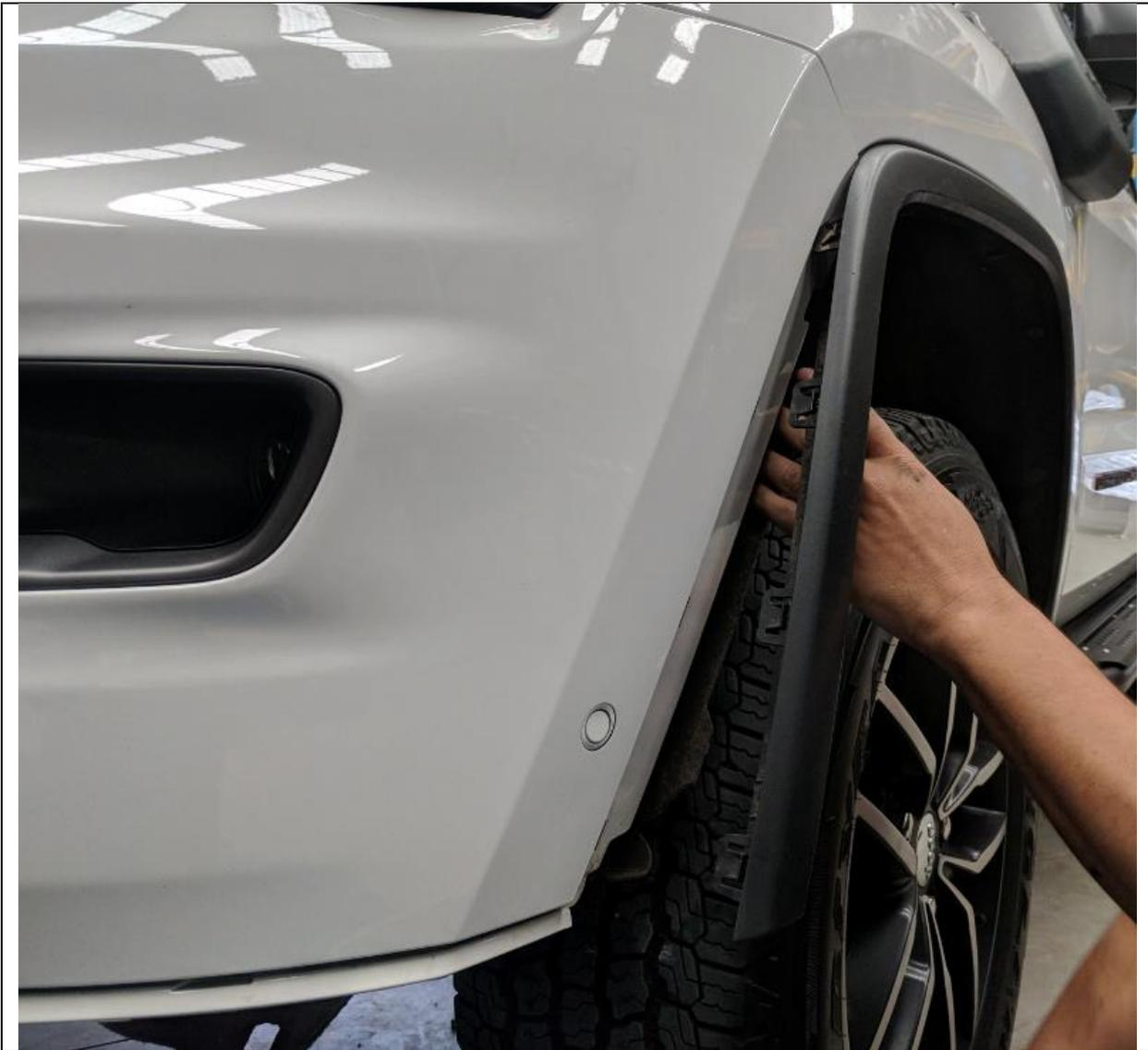
10. Pull factory flare away from bumper, using a flat head screw driver release at least 2 of the push in clips on top edge being careful not to break them as you pull the flare away from the body
