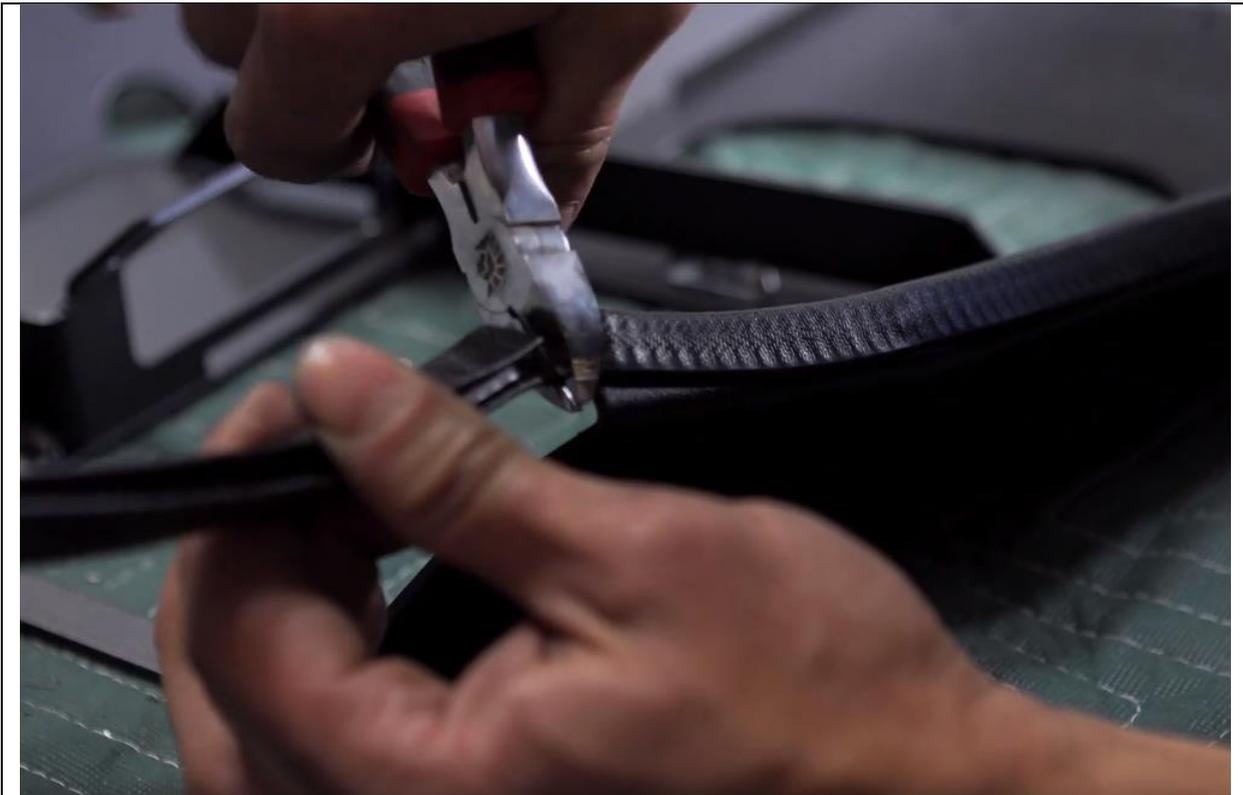
23. Trim edges of pinch weld at edge of plate
