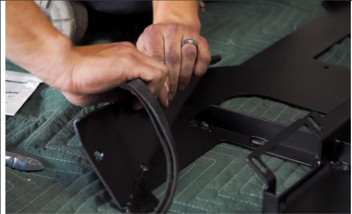
22. Fit pinch weld to top edge of main plate and wings
