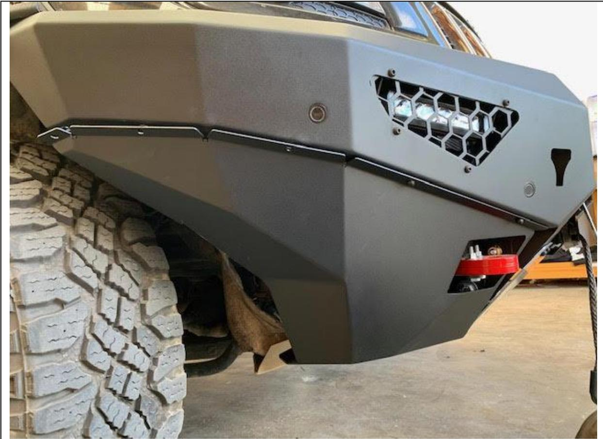
122. Fit under panels as shown with M6 along top edge and M8x 30 bolts. Trim Felt wheel well liner with razor blade so it tucks neatly behind the under panel which will hold it in place.
