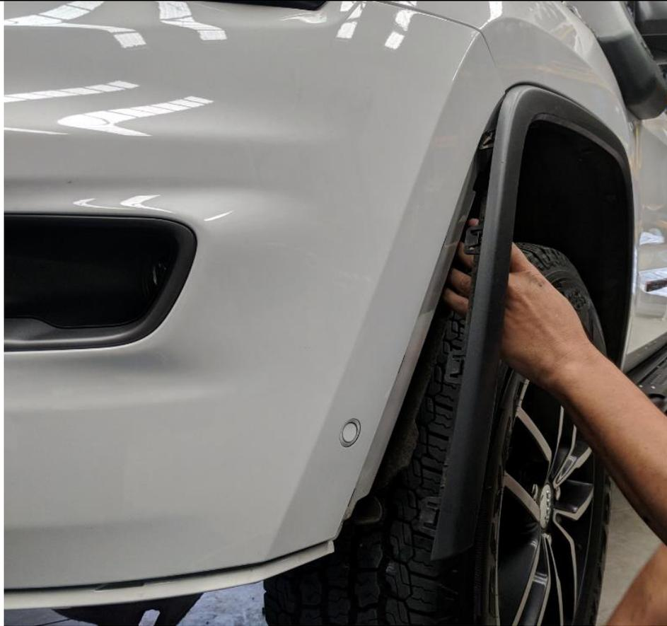
63. Pull factory flare away from bumper, using a flat head screw driver release at least 2 of the push in clips on top edge being careful not to break them as you pull the flare away from the body
