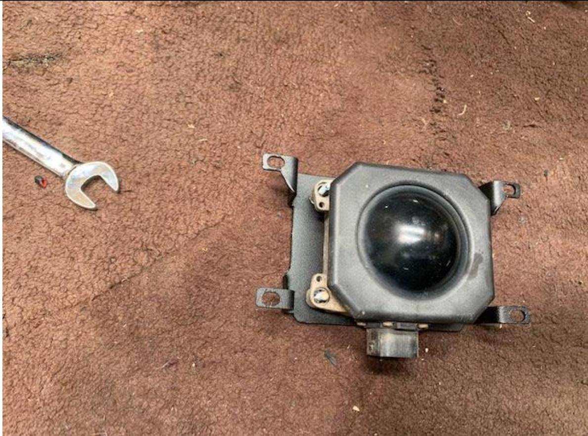
101. Fit Radar to ACC bracket as shown MY 14-MY16 with supplied M5 screws.
