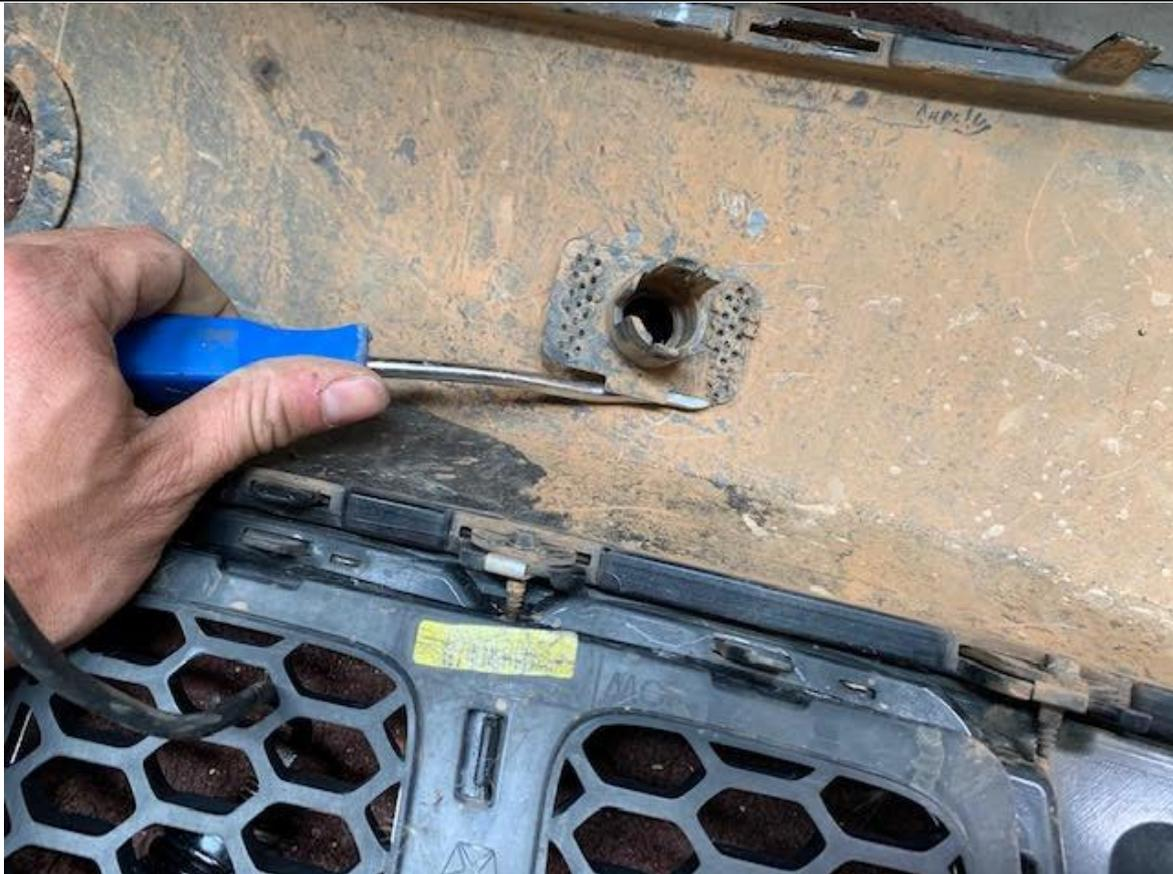
77. If factory parking sensors are present on the vehicle you'll need to remove the sensor from each housing and pry the housing off the bumper with a trim tool or flat head screw driver
