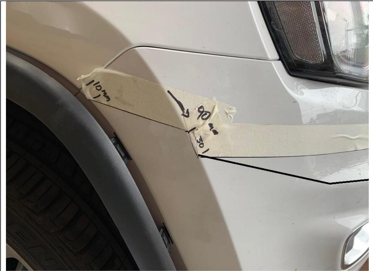
36. Use masking tape above the cut line to protect the bumper section you're going to keep
