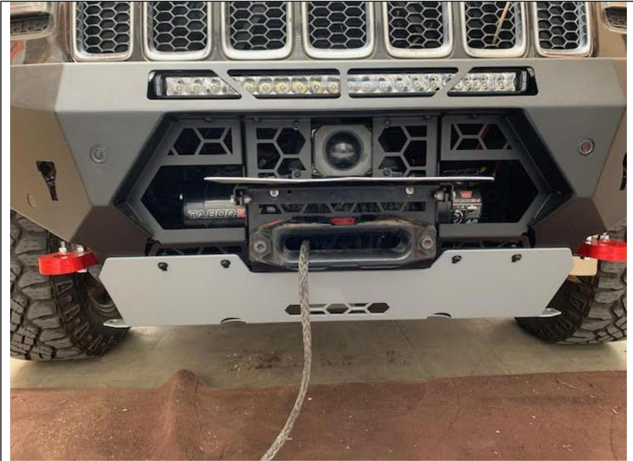
118. Fit bash plate as shown with M8 hardware through bash plate, mesh panel and into winch cradle.
