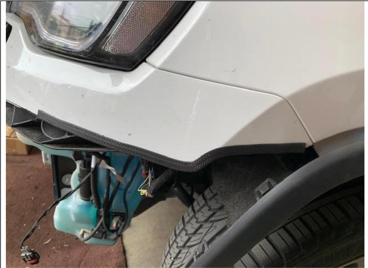
87. Fit a small section of pinch weld as shown
