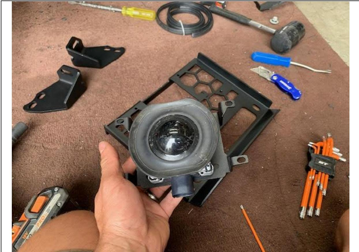
109. Fit ACC mount with Radar to centre mesh panel with M6 hardware
