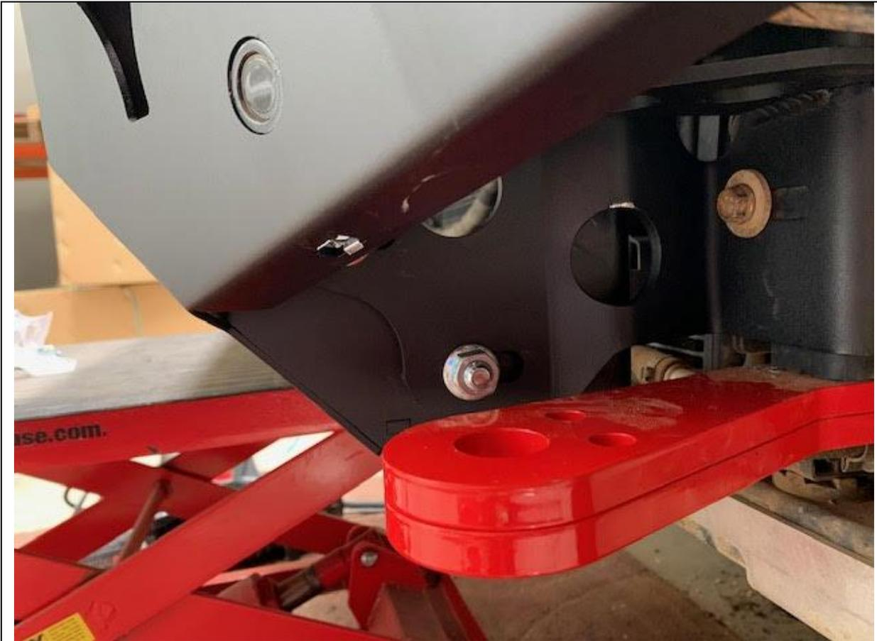
93. Fit the rest of the M12 x 30 bolts, flat washers and Nyloc nuts, leave loose for now.
