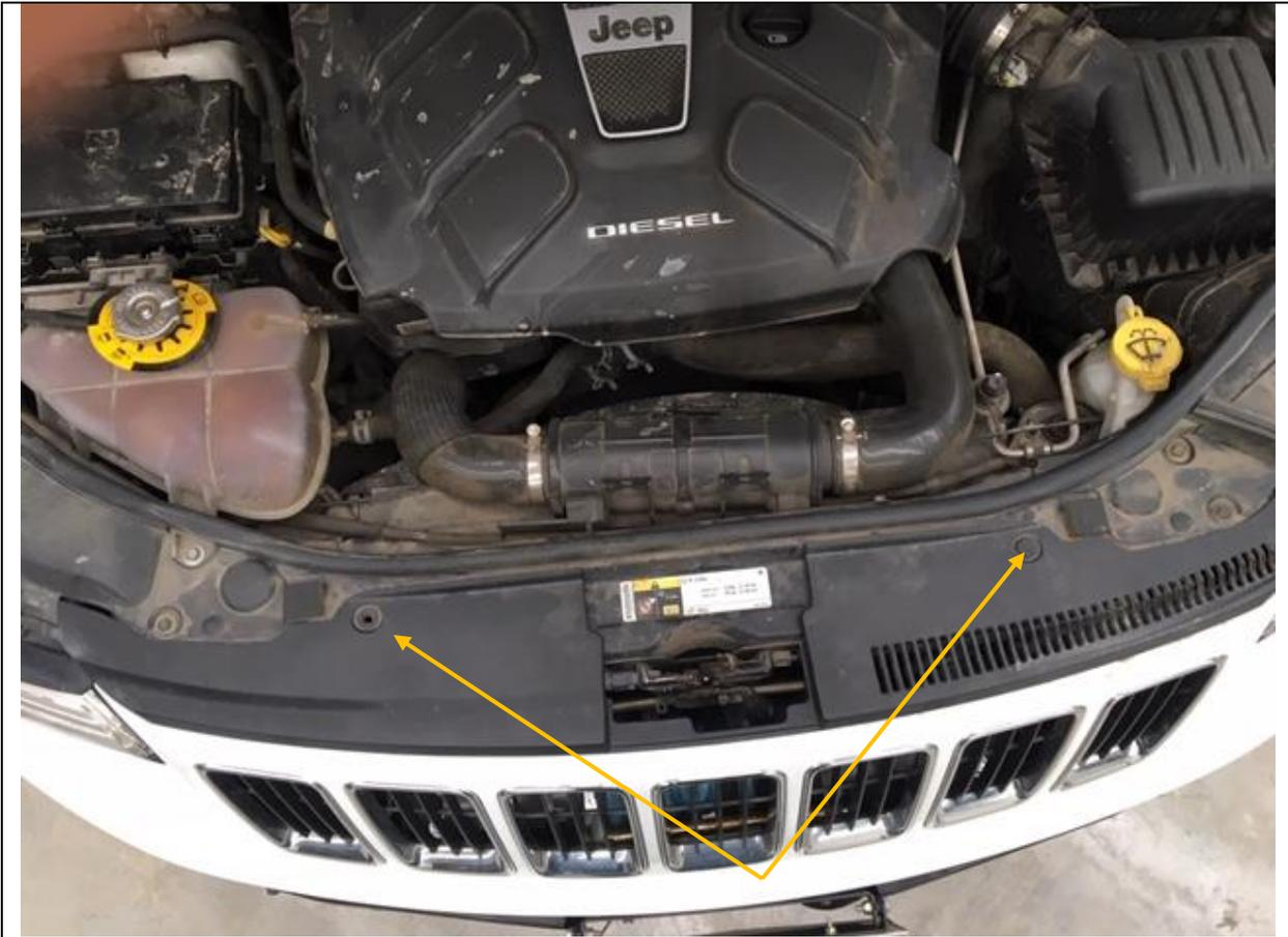
60. Next step is to remove the rest of the front bumper. Start with bonnet/hood open and pry out two clips shown with trim tool or flat head screw driver
