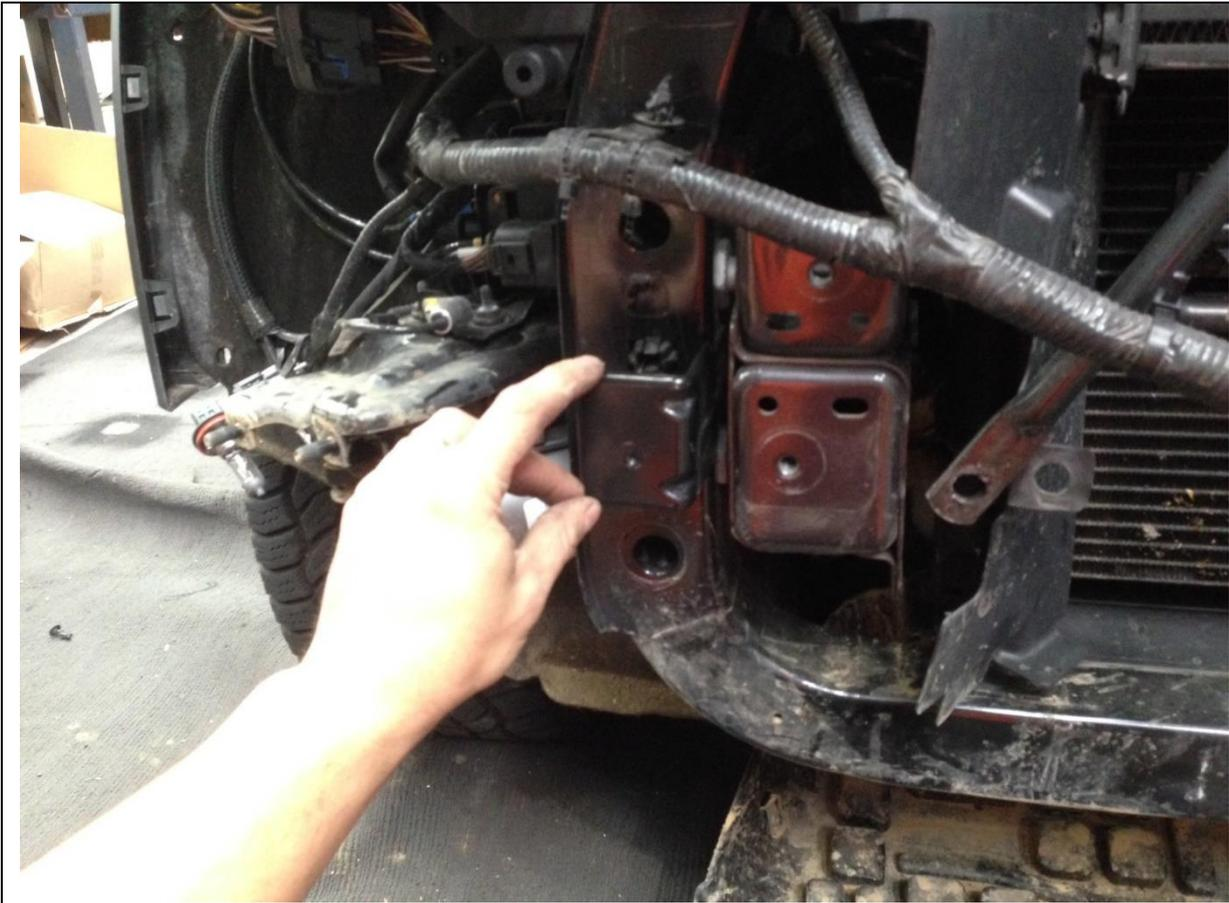
73. Cut tab off shown in picture from both sides, you can bend it back and forth a few times and remove by hand
