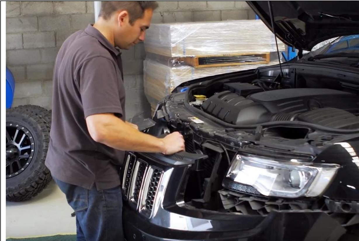
65. Lifting the top section ever so slightly you can release clips holding in the top section and pull the remainder of the bumper away
