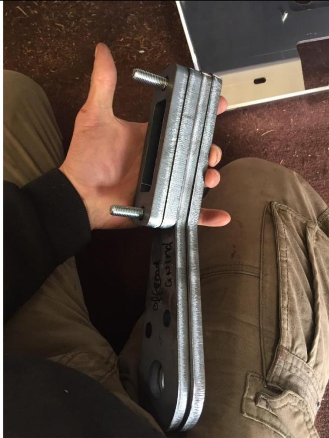
5. Stack Offroad Animal Tow points together as shown with M10 bolts and M10 flat washers.
