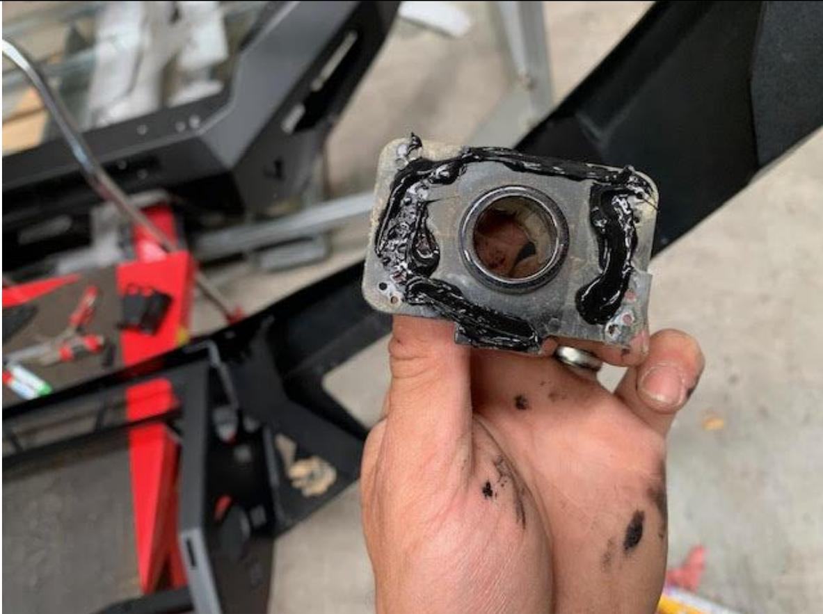
78. Clean the front face of the sensor mount and when dry apply a healthy amount of adhesive silicone to the front face of each sensor mount
