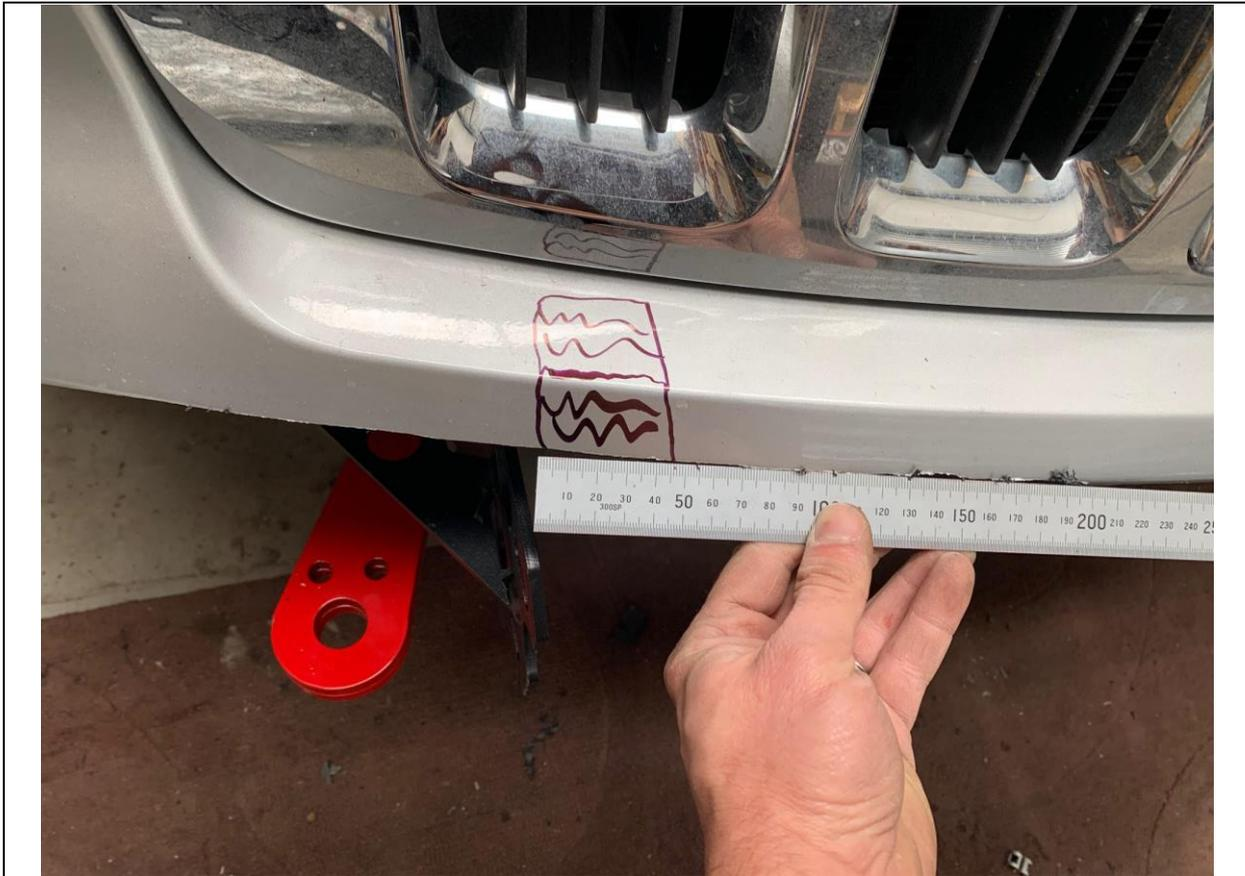
58. With the bumper back on, and the mounts installed, mark a point directly above the flat face of the mount then 45mm toward the centre of the car. Then 40mm up towards the car. Shade this area and cut it out
