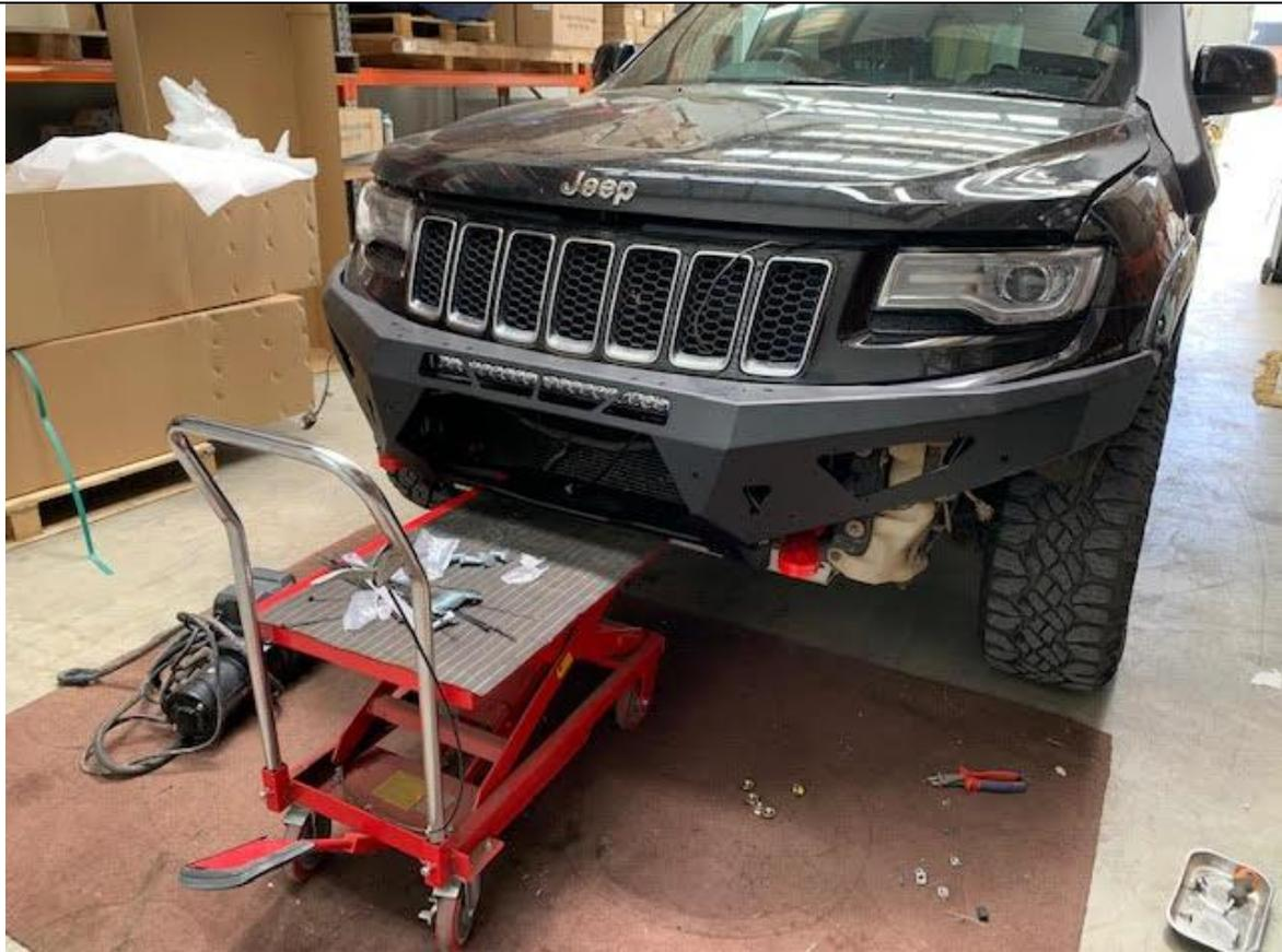
92. With the help of a friend or lifting table (guess which one is easier, no it's not with your friend) lift the bar on top the mounts and hold up with M12x 30 hex bolts, flat washers and nuts
