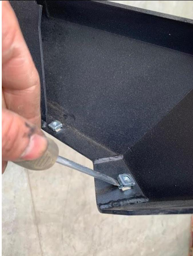
84. Fit cage nuts to the bar as shown. You can often just push them in by hand, otherwise use a flat head screwdriver. You may need to use the screwdriver to open the legs of each nut from underneath
