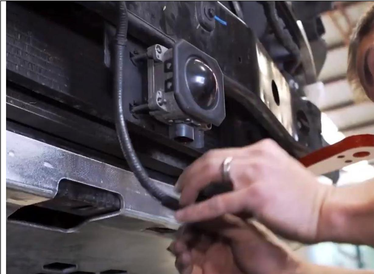
71. If Adaptive cruise control is fitted, unplug loom and pull sensor off posts
