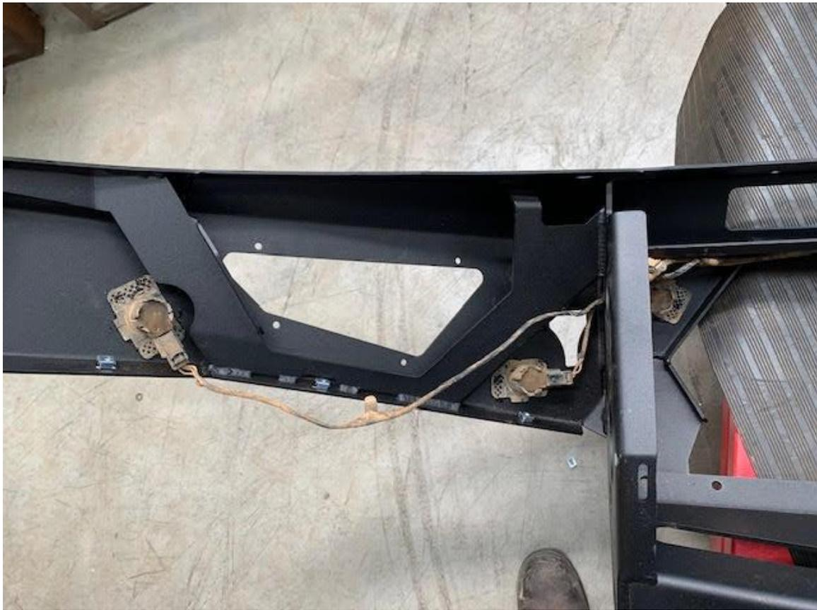
85. After at least an hour push the sensors into their housings. Make sure the housings are set, if the weather is cold you may need to wait longer.
