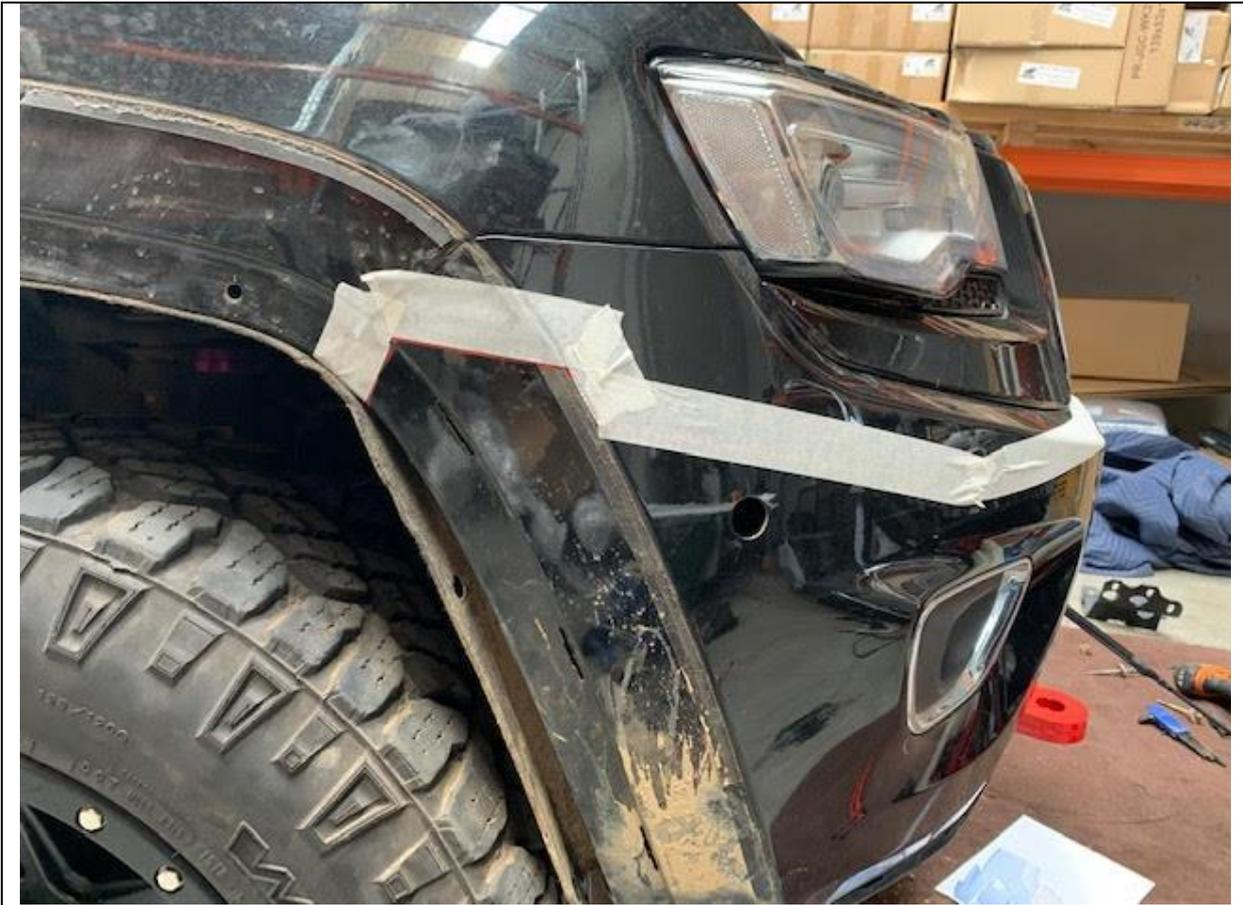
22. Use masking tape to mark out the cut lines. Put the masking tape above the cut lines to protect the portion of the bumper that will stay.
