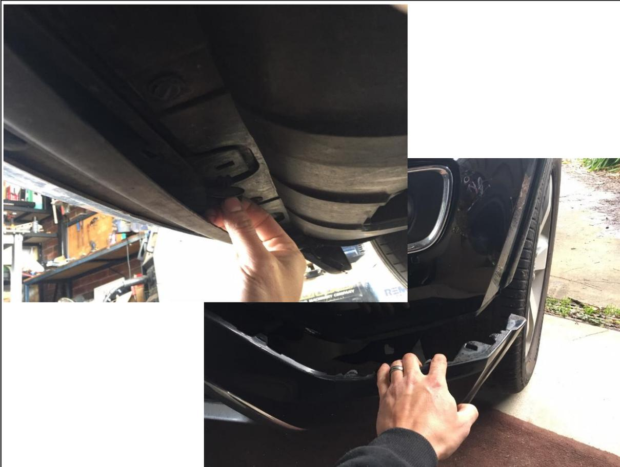
1. First step is to remove the lower air damn fascia. To do this climb under your Jeep and remove all 7 quarter turn clips by hand. Two are tucked up high in each corner and 3 in the middle
