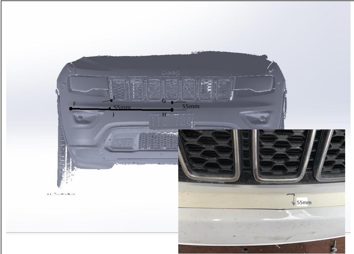
31. Point G is the centre of the bumper from left to right and the top most mold line
