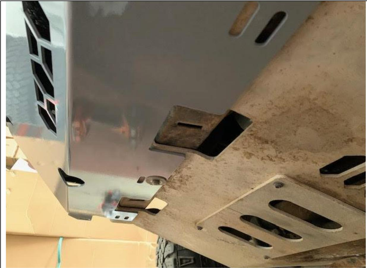
121. Fit lower factory M6 bolts through bash plate into cross member. Do not over-torque these
