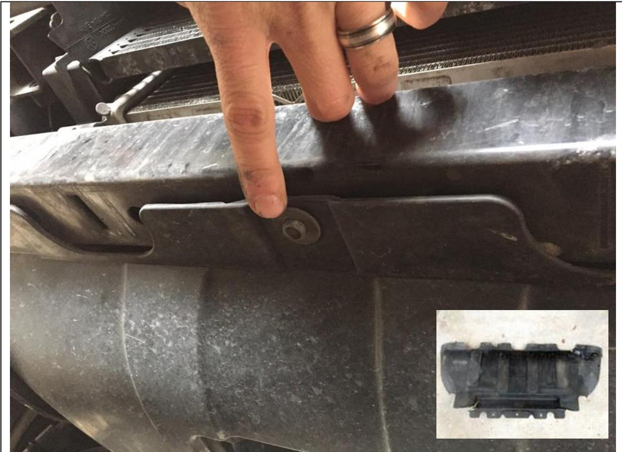
3. Remove factory Lower Radiator Cover. 3x M6 bolts on front and 2x M8 bolts on back. Use 10mm socket or spanner for front and 13mm for rear
