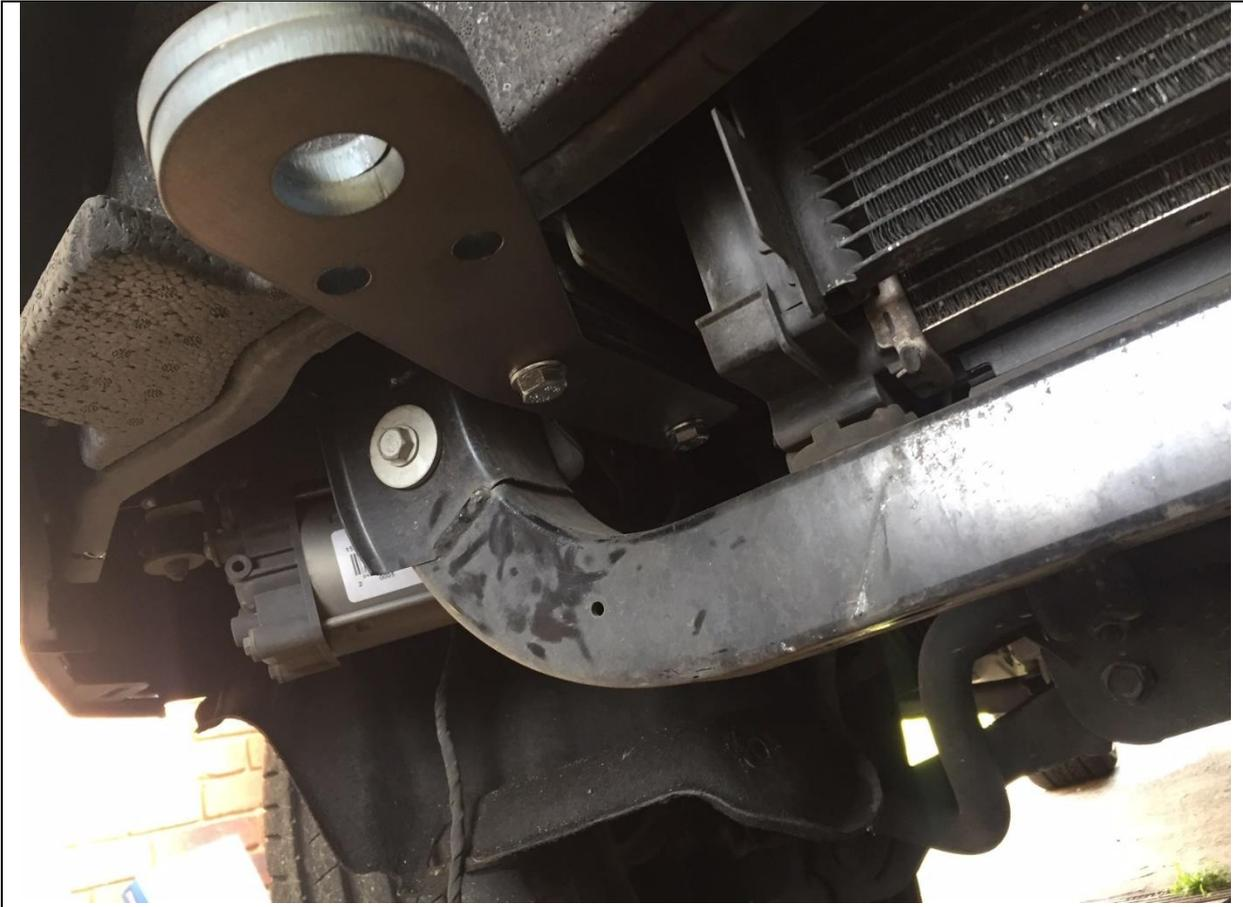
6. Fit Offroad Animal Tow points as shown on LH and RH side with M10x80 bolts directly into frame of Jeep. Torque down bolts
