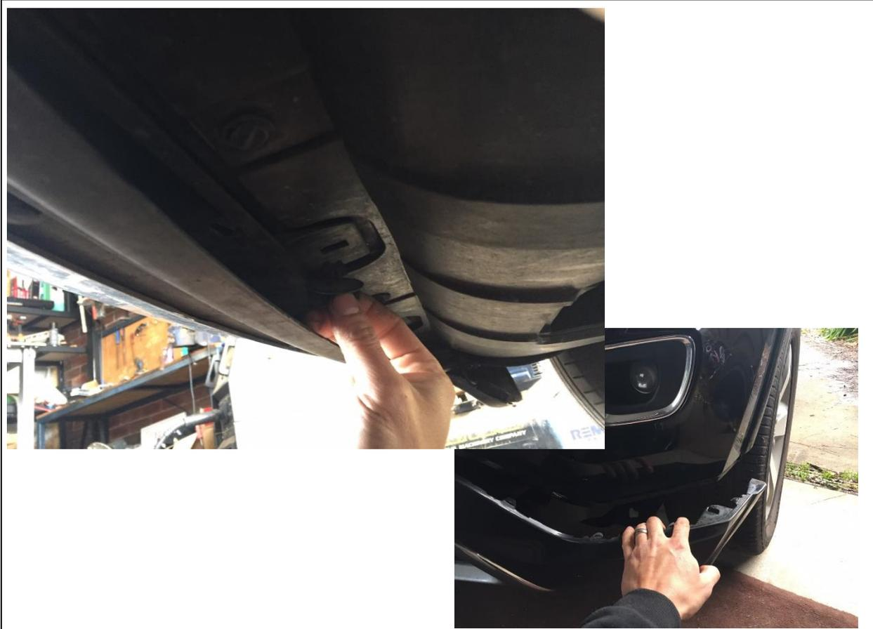
1. First step is to remove the lower air damn fascia. To do this climb under your Jeep and remove all 5 quarter turn clips by hand. Two are tucked up high in each corner and 3 in the middle
