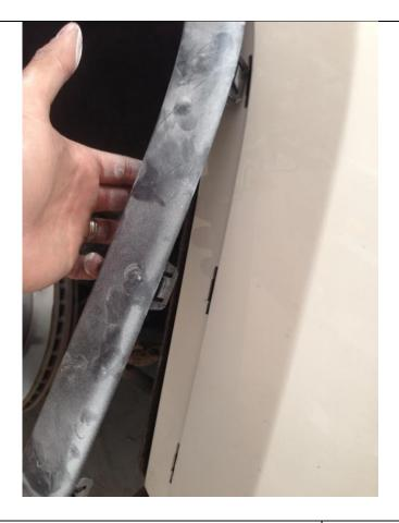
5. Pull factory flare away from bumper, using a flat head screw driver release at least 2 of the push in clips on top edge being careful not to break them as you pull the flare away from the body
