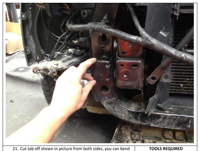
21. Cut tab off shown in picture from both sides, you can bend it back and forth a few times and remove by hand
