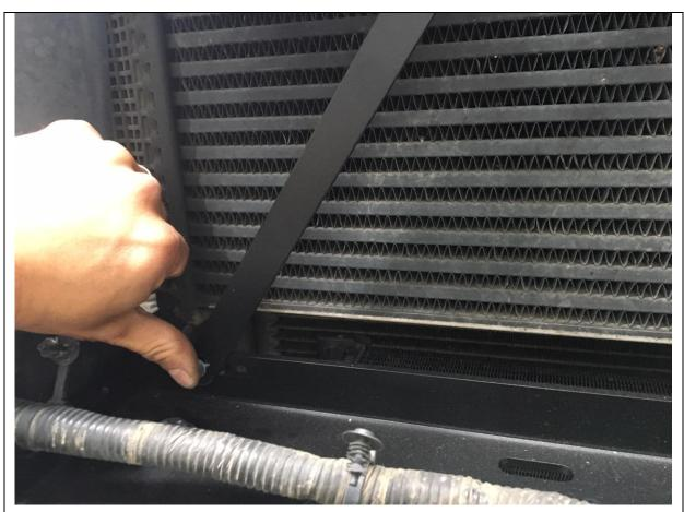
32. Fit lower end of radiator supports to winch cradle with M6 bolts, flat washers and flange nuts
