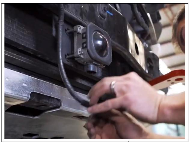
17. If Adaptive cruise control is fitted, unplug loom and pull sensor off posts
