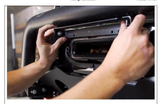
46. If purchased fit number plate flip to bumper. Drill holes and fit with M6 supplier hardware from number plate flip
