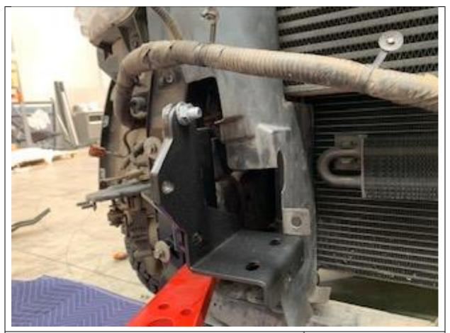
24. Fit sub support with M10 bolts, flat washer and flange nuts.
