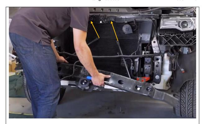
18. Remove 2x screws with 13mm tool holding round support bars from top of bonnet support then remove entire reinforcement bar.
