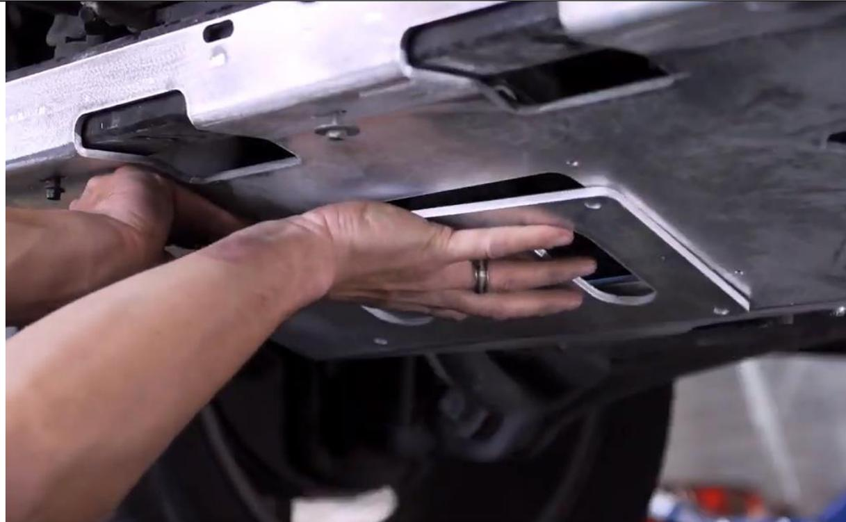
7. Fit cover panel with M6 button head cap screws and washers
