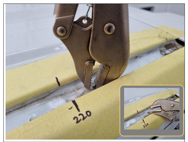
10. If there are any ball studs in the blank gutter regions, pull/twist them with a set of pliers and remove them.
