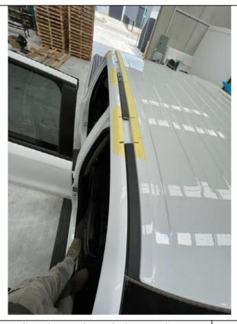
9. Refit the trim as shown leaving the marked sections bare.
