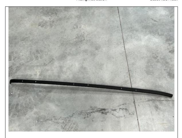
8. Using an angle grinder cut the trim piece length removing the marked sections.
