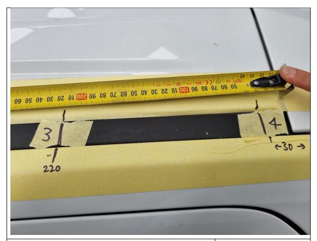
3. Mark a line at 30mm and another at 220mm. Mark on the black trim as well as the masking tape.
