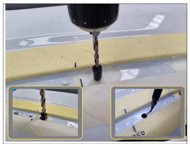
19. Drill the roof out to 11mm. Start with a pilot drill of 5mm, then move up to 8mm and finally 11mm. Ensure nutsert fits in each hole.
