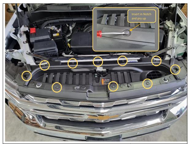
3. Remove 10x plastic push rivets securing the radiator grille cover, by levering centre section upwards using flat bladed screwdriver or trim tool, as shown.
