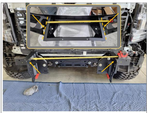
41. Measure the distance between the outside faces of uprights on bar using tape measure. Write distance below for reference if required.
