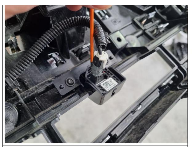
53. If equipped, the front camera can be optionally relocated for a clearer unobstructed view. This is especially recommended if running optional driving lights or top tubes.
