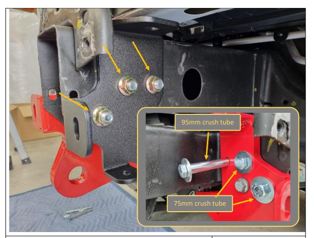
29. Fit the RH chassis mount brace bracket to the inside of the RH chassis rail and secure with 3x M12x120 hex bolt, 3x flat washer, 2x 75mm crush tube, 1x 95mm crush tube and 3x flange nut.
