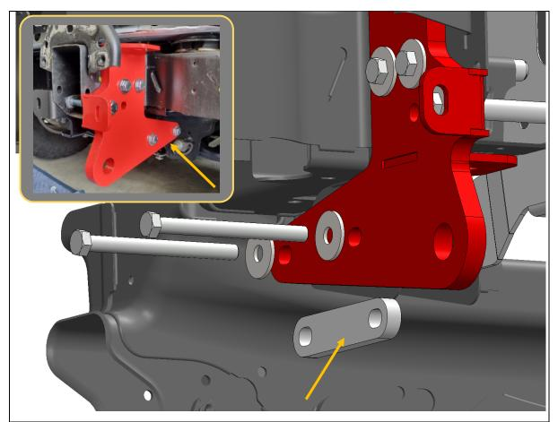
33. Insert the rear tow point spacer plate between the tow point and chassis at the rear, then loosely secure with 2x M12x130 hex bolts, flat washers and flange nuts.
