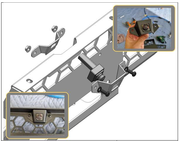
110. If relocating the front camera, sandwich the camera between the camera mount and backing plate, then attach to the mesh fairlead mount using 2x M16x16 black button head bolts, black flat washers and flange nuts.
