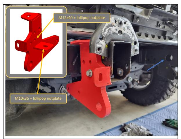
26. Fit the RH tow point to the vehicle using the retained factory M12x40 hex bolt (from Step 23) + M12 nutplate on the side and factory M10x35 hex bolt (from Step 11) + M10 nutplate on the bottom.
