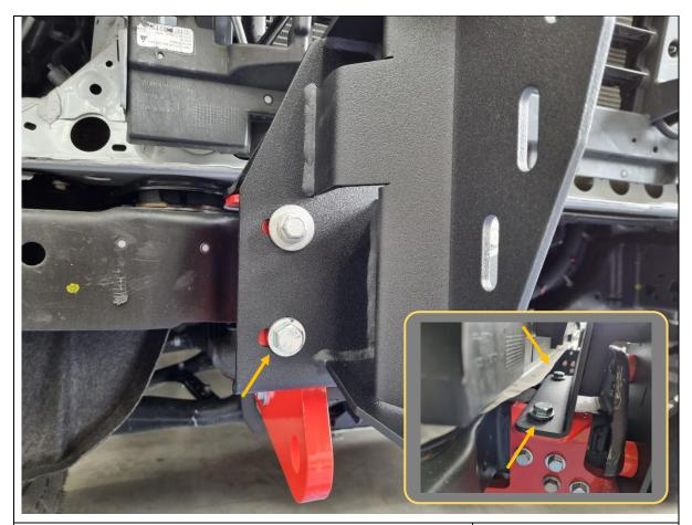
44. Fit remaining 4x M12x30 hex bolts, flat washers and flange nuts for the RH impact assembly.
