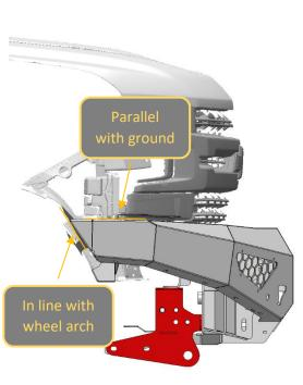
88. With assistance, from another person, align the bar with the edges of the vehicle. The bar should sit symmetric left/right on the vehicle.
