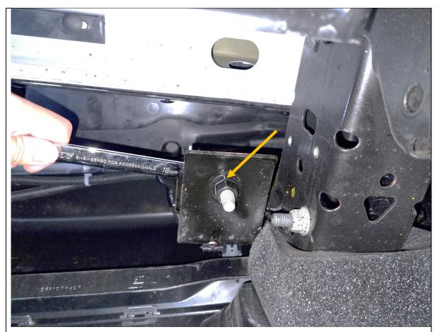
14. Above the middle bumper support bracket on the inside face of the chassis rail will be an 18mm hex bolt.
