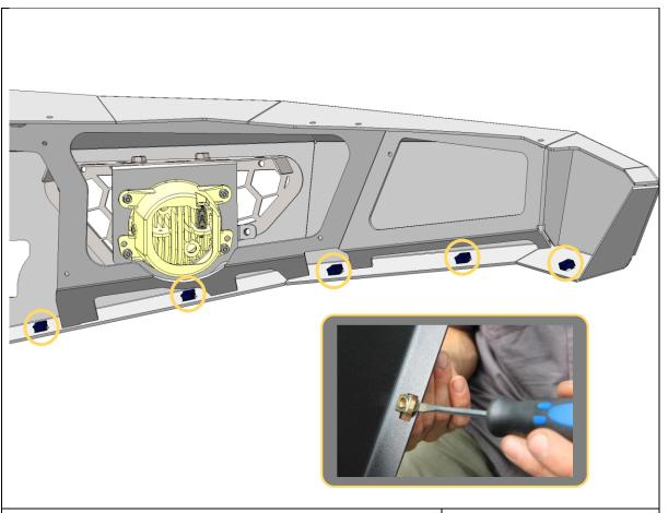
71. Fit 5x M6 cage nuts into the rectangular slots on the bottom of the bar wing.
