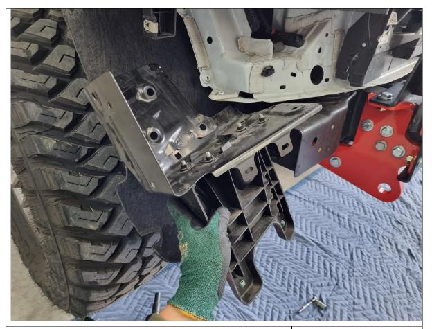
49. Using a 10mm socket, remove all the bolts securing the wheel guard bracket to the vehicle. Retain these fasteners for re-use.
