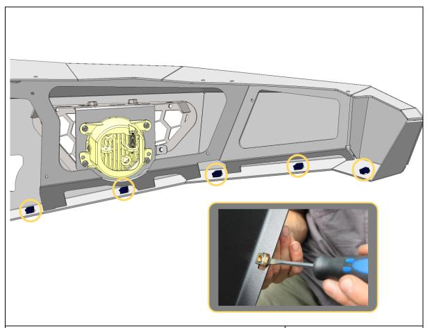
95. Fit 5x M6 cage nuts into the rectangular slots on the bottom of the bar wing.
