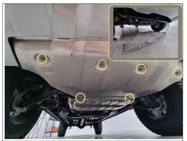
12. Remove 6x M8 bolts securing the bash plate to the vehicle, then remove and discard bash plate.
