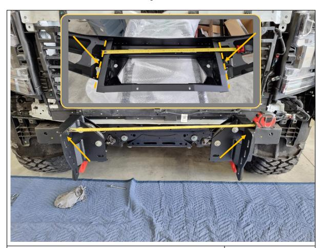
43. Measure the distance between the outside faces of uprights on bar using tape measure. Write distance below for reference if required.
