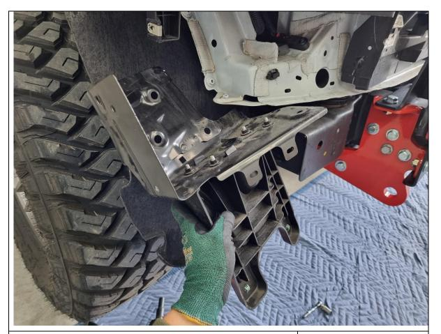
73. Using a 10mm socket, remove all the bolts securing the wheel guard bracket to the vehicle and headlight. Retain these fasteners for re-use.
