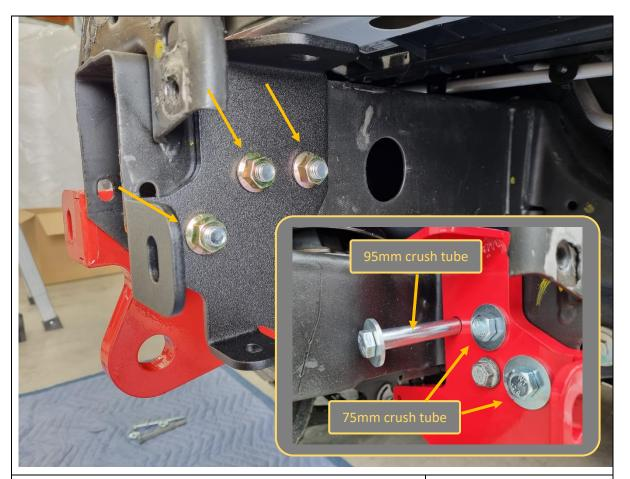
31. Fit the RH chassis mount brace bracket to the inside of the RH chassis rail and secure with 3x M12x120 hex bolt, 3x flat washer, 2x 75mm crush tube, 1x 95mm crush tube and 3x flange nut.
