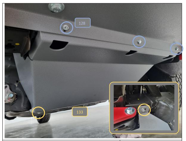
127. Fit the lower bash plate to the vehicle by re-using the 4x 13mm hex bolts from Step 12.
