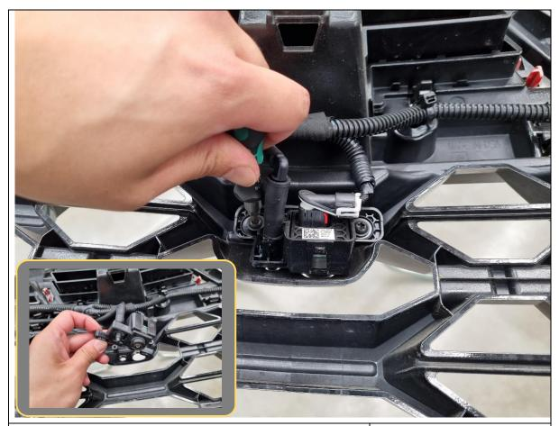
48. The front camera can be optionally relocated from the grille into the bar for a clearer unobstructed view. This is especially recommended if running optional driving lights or top tubes.
