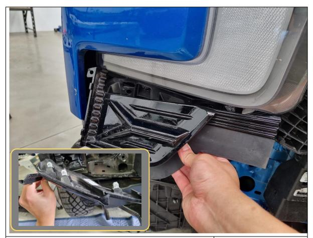
55. Pull and release the clips securing the plastic trim below the headlight. Discard this piece.
