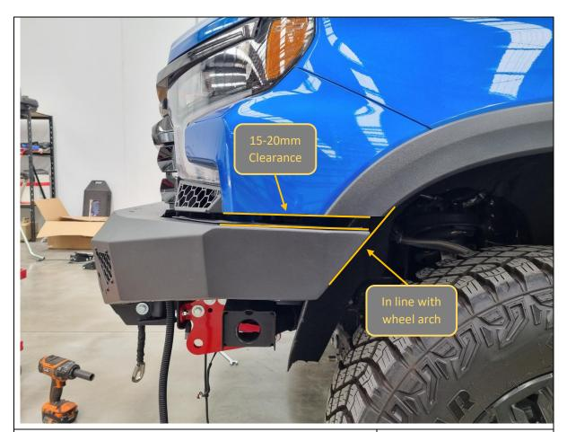
105. With assistance, from another person, align the bar with the edges of the vehicle. The bar should sit symmetric left/right on the vehicle.
