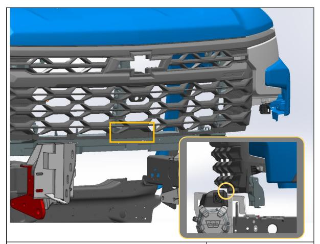
54. If fitting a WARN Zeon or a winch with a similar size, a small portion of the grille may need to cut to provide adequate clearance to the control box. It is best to do this before the bar is fully installed onto the vehicle.
