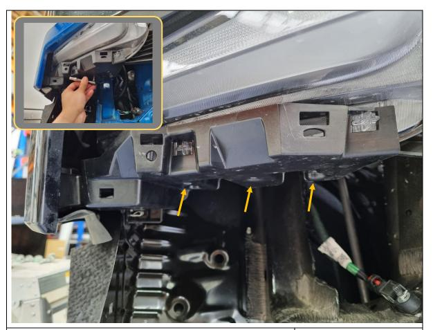
56. Remove the bumper clip underneath the headlight by loosening 3x T15 Torx screws. Do not discard the fasteners.
