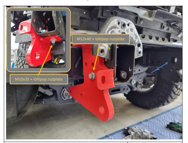
28. Fit the RH tow point to the vehicle using the retained factory M12x40 hex bolt (from Step 23) + M12 nutplate on the side and factory M10x35 hex bolt (from Step 13) + M10 nutplate on the bottom.
