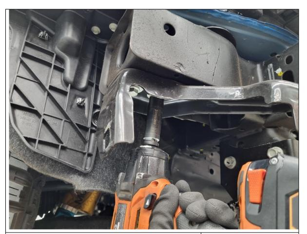
26. Remove the 2x 15mm hex bolts securing the bumper support bracket to the chassis. Retain bolts for re-use.
