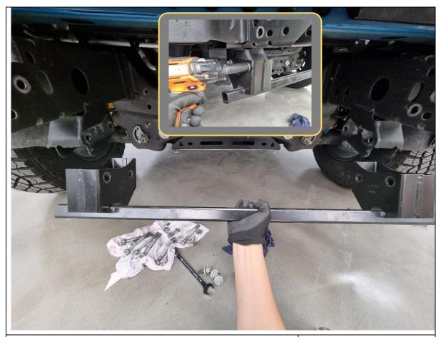
25. Remove the 4x 18mm hex bolts (2x per side) securing the bash place reinforcement member to the chassis.
