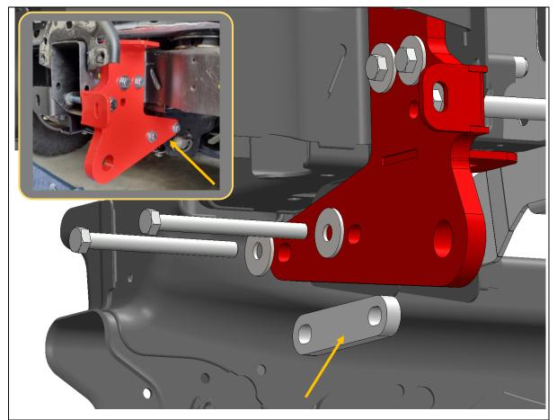
35. Insert the rear tow point spacer plate between the tow point and chassis at the rear, then loosely secure with 2x M12x130 hex bolts, flat washers and flange nuts.
