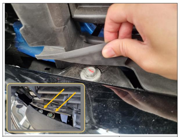
17. On the top lip of the bumper, there are 2x hex bolts hidden behind a rubber cover panel, above where the inner bolts were from the previous step.
