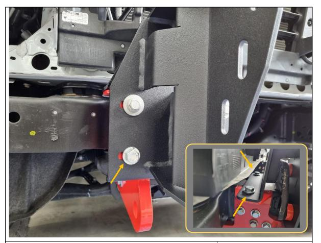
46. Fit remaining 4x M12x30 hex bolts, flat washers and flange nuts for the RH impact assembly.
