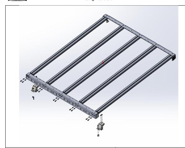
1. Assemble the rack as shown above with M8 hardware.
