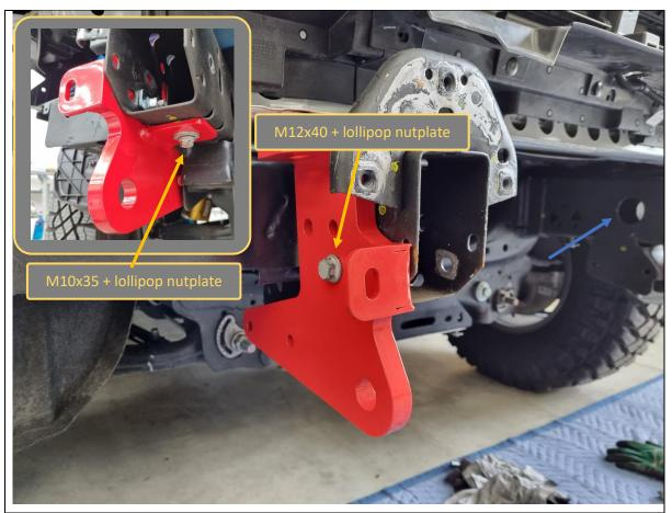
35. Fit the RH tow point to the vehicle using the retained factory M12x40 hex bolt (from Step 32) + M12 nutplate on the side and factory M10x35 hex bolt (from Step 24) + M10 nutplate on the bottom.
