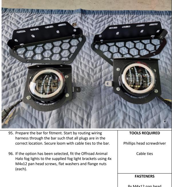
8x M4x12 pan head 8x M4 flat washer 8x M4 flange nut
