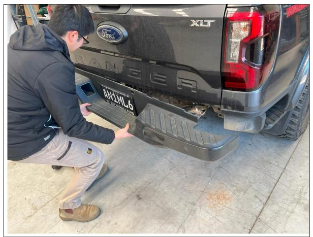
6. With all fasteners removed and the factory bumper assembly free, remove the bumper from the vehicle in a rearward direction
