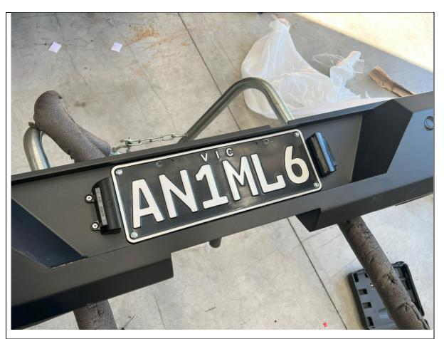
33. Re-Fit number plate to the bar, using supplied M5 Fasteners.
