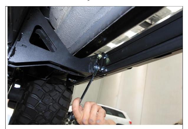
52. Tighten all mount to slider M10 flange nuts using 15mm spanner. A ratcheting spanner makes this process easier
