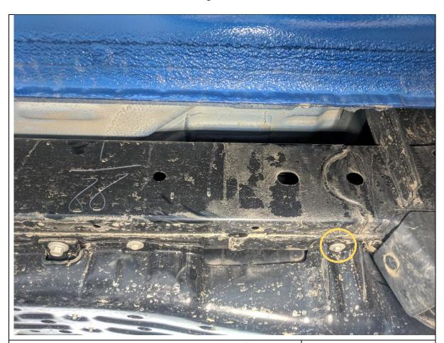
18. Locate and remove the rear most 10mm head factory bolt securing the plastic fuel tank guard to the chassis.
