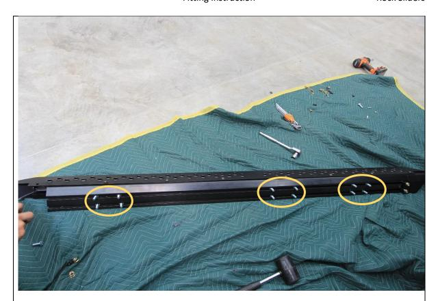
38. Slide the 12x M10x25 Hex bolts into the T slots on back side of extrusion. 6 bolts per slot.
