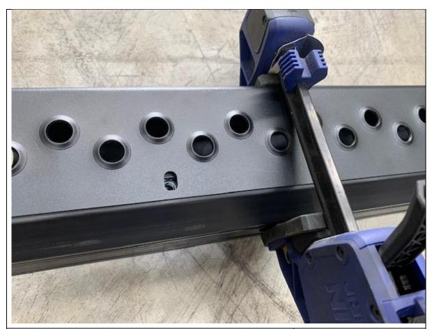
33. Using long tool feed nuts in to centre first and thread in with black M8 button head cap screws and washers
