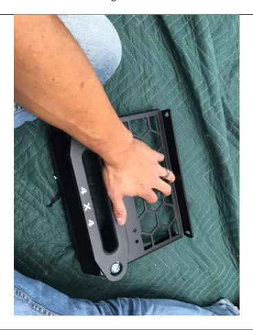
48. If fitting a winch fit fairlead to centre mesh panel with winch supplied hardware
