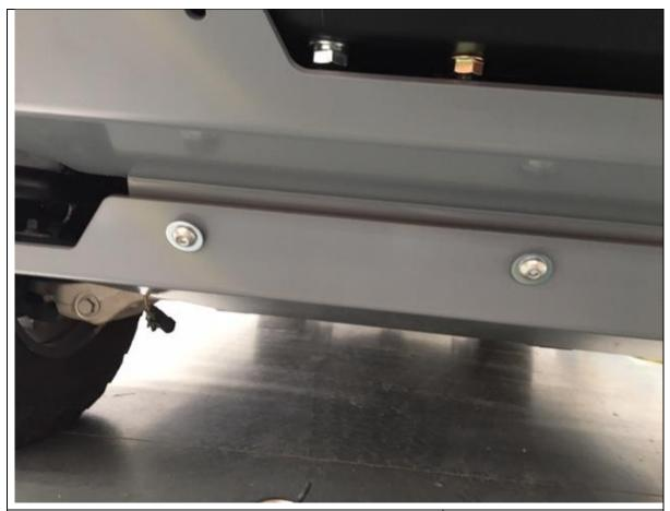
63. M10 button head cap screws tying in both bash plates shown
