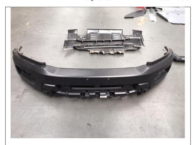
22. Shown is front bumper, bash plate and fascia panels that are no longer required.
