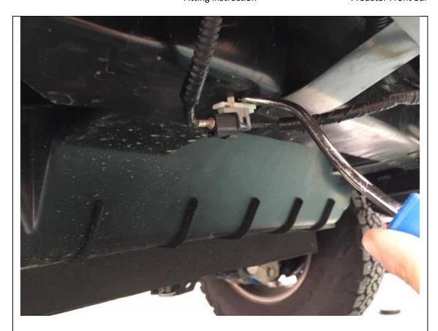
12. Pry out connector and retainers for fog light loom as shown
