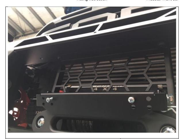
50. Fit centre mesh panel to bar with M8 x 16 black button head cap screw through the top and M8 x 20 black button head cap screws through bottom. Use washers and flange nuts
