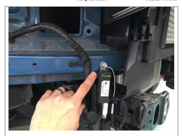
26. Relocate FM control box to tapped hole on body as shown
