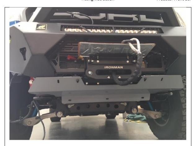
61. Fit front bash plate to lower section of bar. Insert part P-0072 shim plate between bar and bash plate. Use M8 x 30 button head cap screws, flat washers and flange nuts. Leave bolts loose
