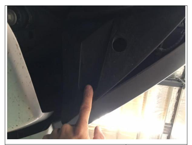
2. Remove one screw from underside (1 per side)
