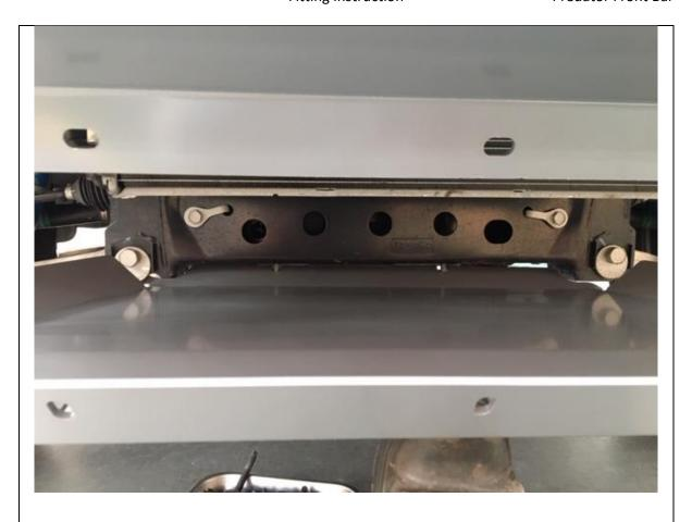
62. Time to fit new lower bash plate, with factory bolts started into threads at the back you can use them to hold up the back of the bash plate while you lift up the front and feed in M10 x 25 button head cap screws and washers.
