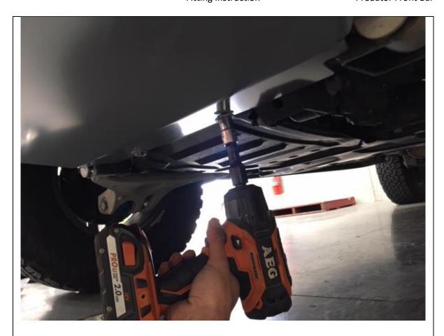
65. Don't forget to torque up bottom factory bolts
