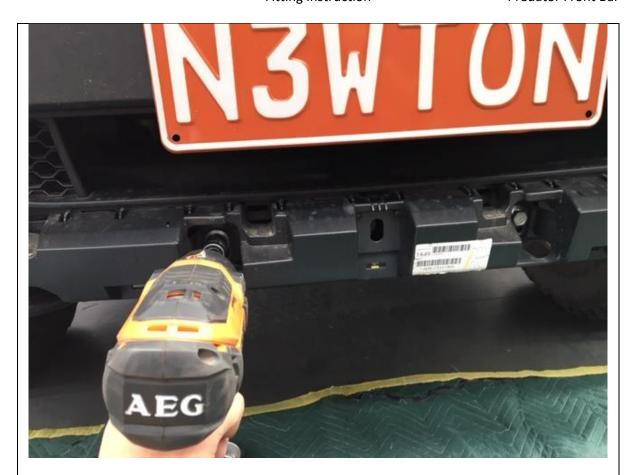
10. Remove 2 x M8 bolts from front as shown
