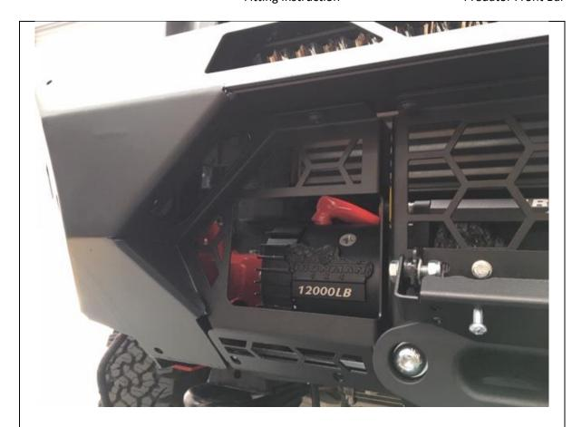
51. Fit RH mesh panels with M8 x 16 button head cap screw wash and flange nut from above as shown
