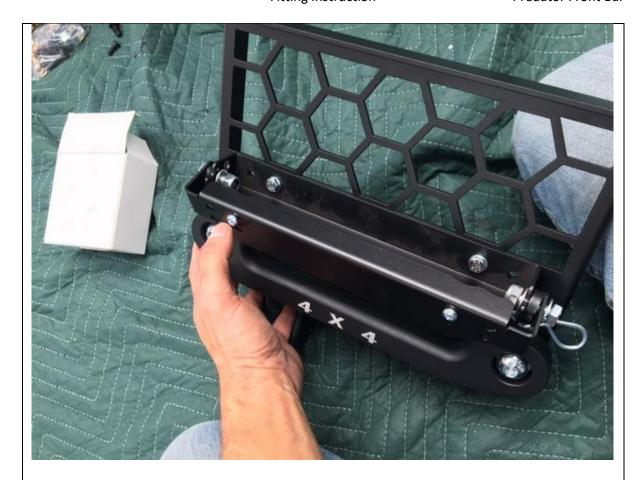
49. Fit Number plate flip bracket to centre panel with M6 hardware
