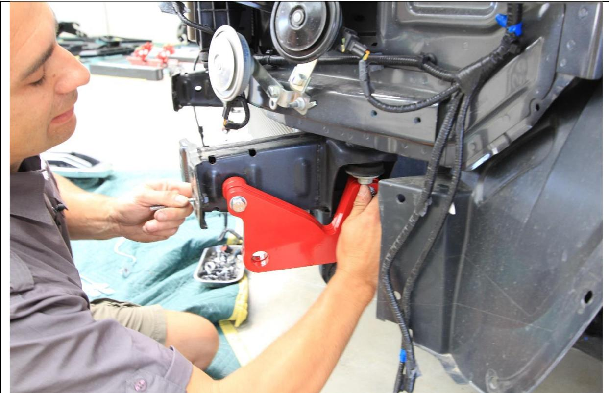
6. Secure using M12 nut plates, inserted from the front of the chassis. Once both bolts are secured tighten using 18MM spanner / Socket.
