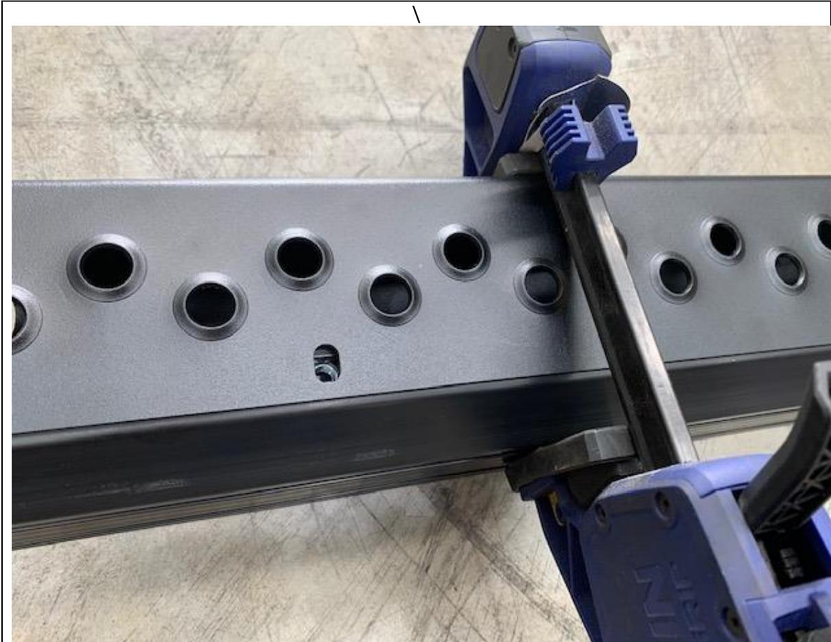
28. Using long tool feed nuts in to centre first and thread in with black M8 button head cap screws and washers
