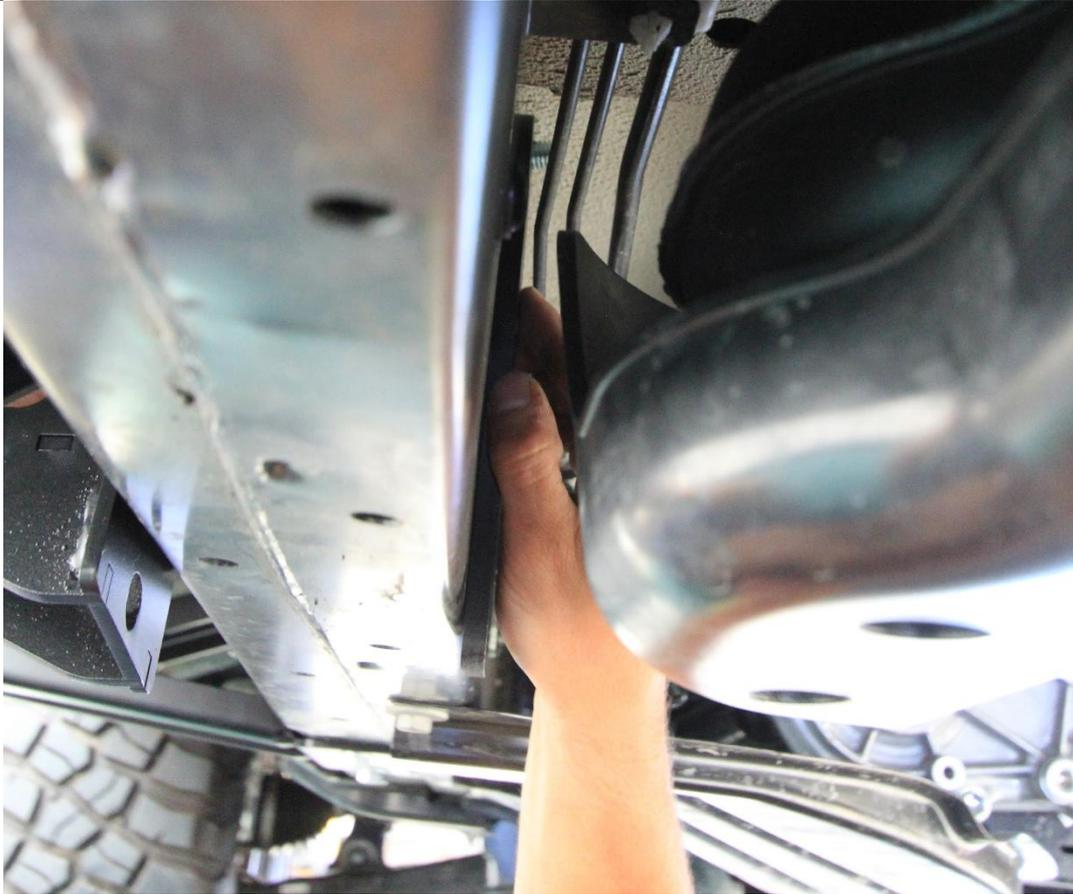
11. Install the mid / rear mount backing plate, by sliding up against back side of chassis and secure through top bolt from mount.
