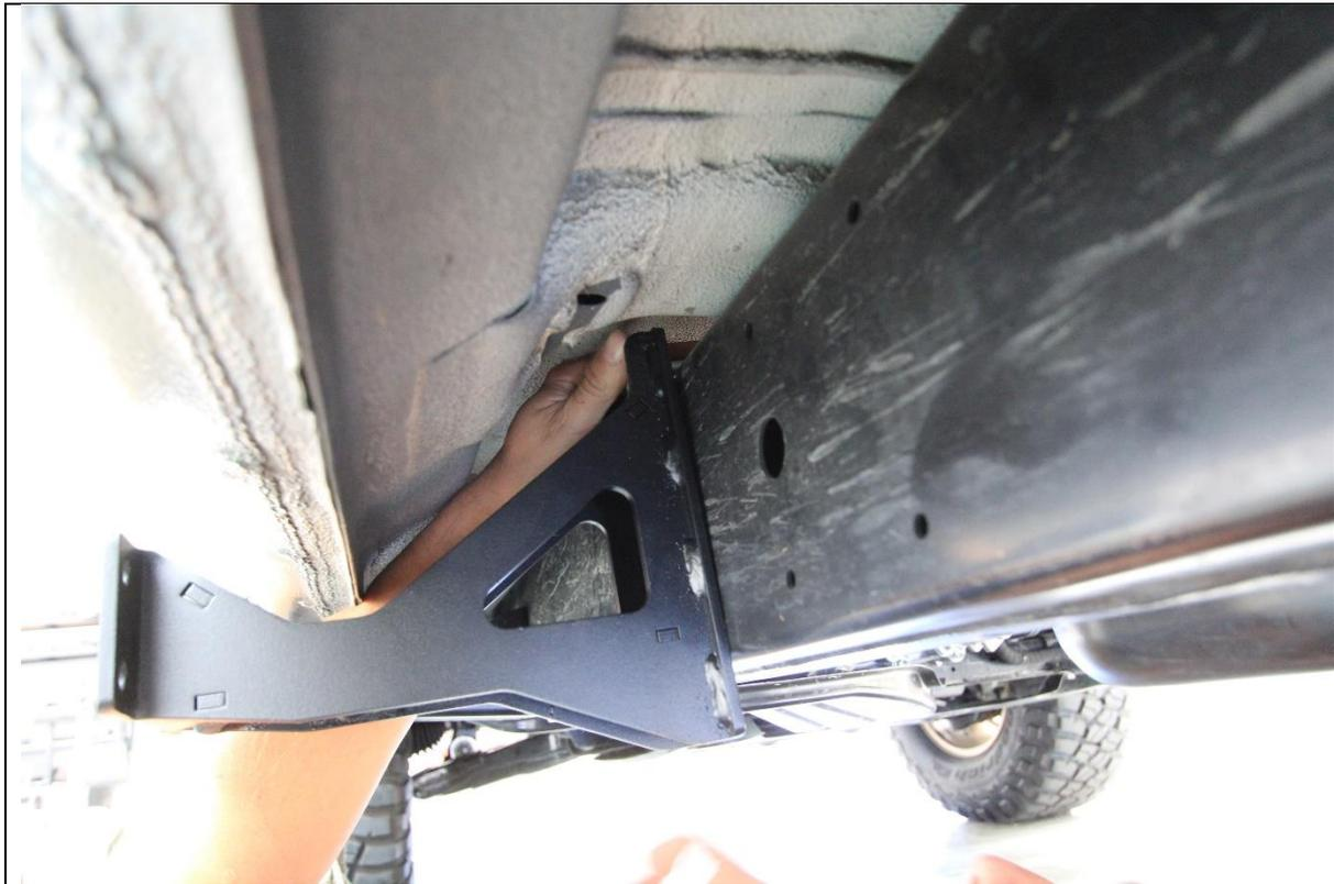
9. Prepare mid and rear mounts by pre-inserting the M12x125 Bolt, with flat washer, part way through the top mounting hole.
