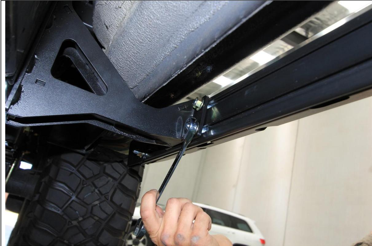
46. Tighten all mount to slider M10 flange nuts using 15mm spanner. A ratcheting spanner makes this process easier
