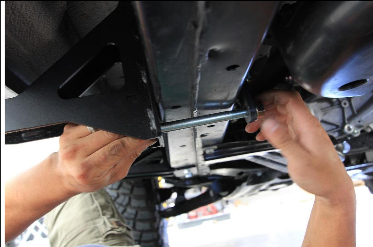
14. Insert the lower M12x125 Bolt and M12 flat washer through both the mount and backing plate
