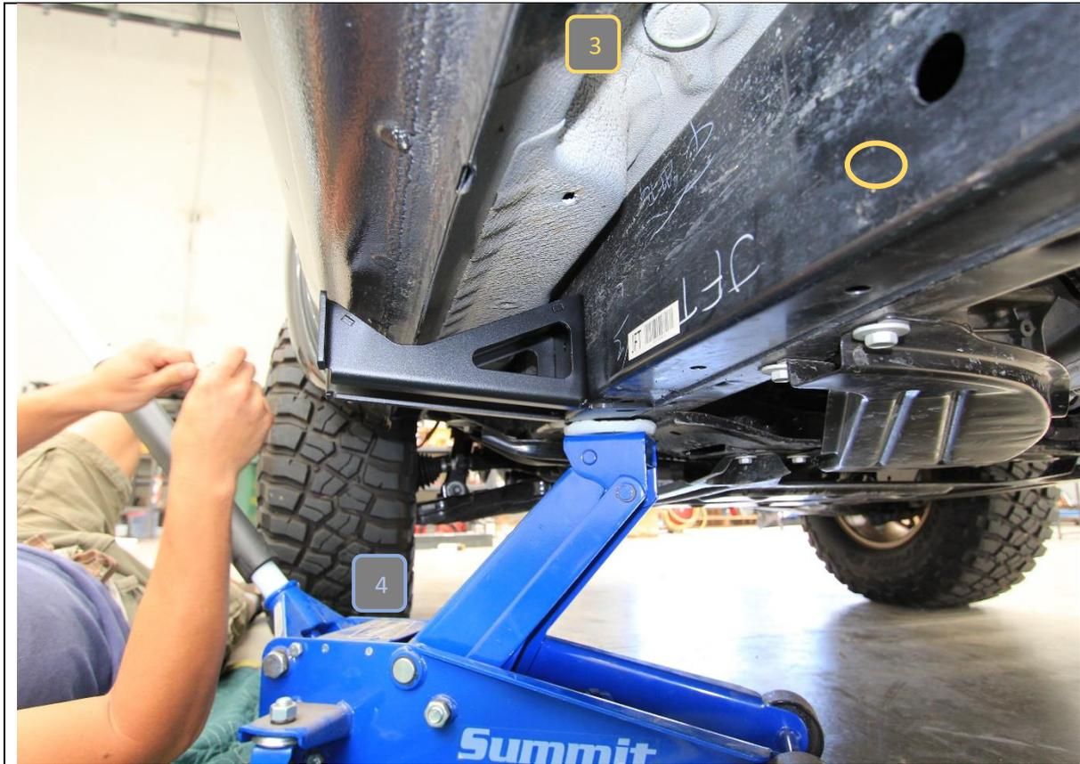
3. Locate features that front mount mounts to. The easiest way to do so is locate the rectangular slot on forward part of chassis closest to the seam weld.
