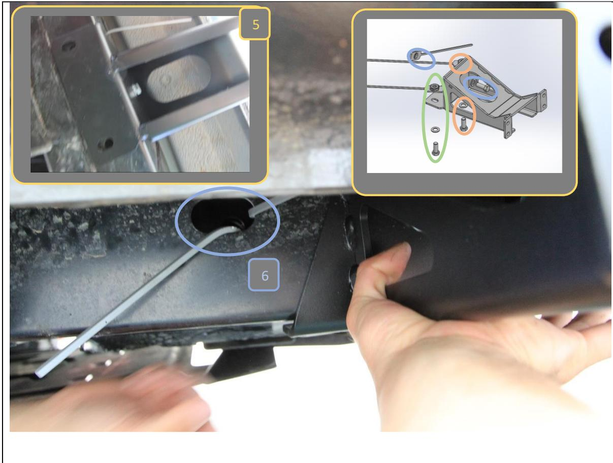
5. Check to ensure that slots on mount are aligned with holes in chassis rail. Adjust position of mount if required
