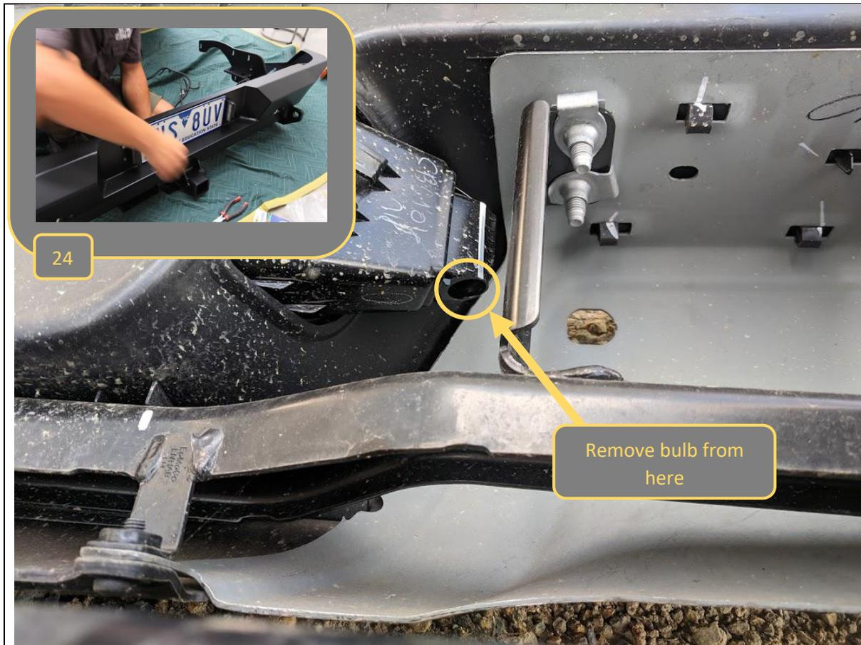
9. Remove Bulbs from Number plate lamps. Bulbs are secured with spring loaded bayonet type attachment, Push and turn to release.
