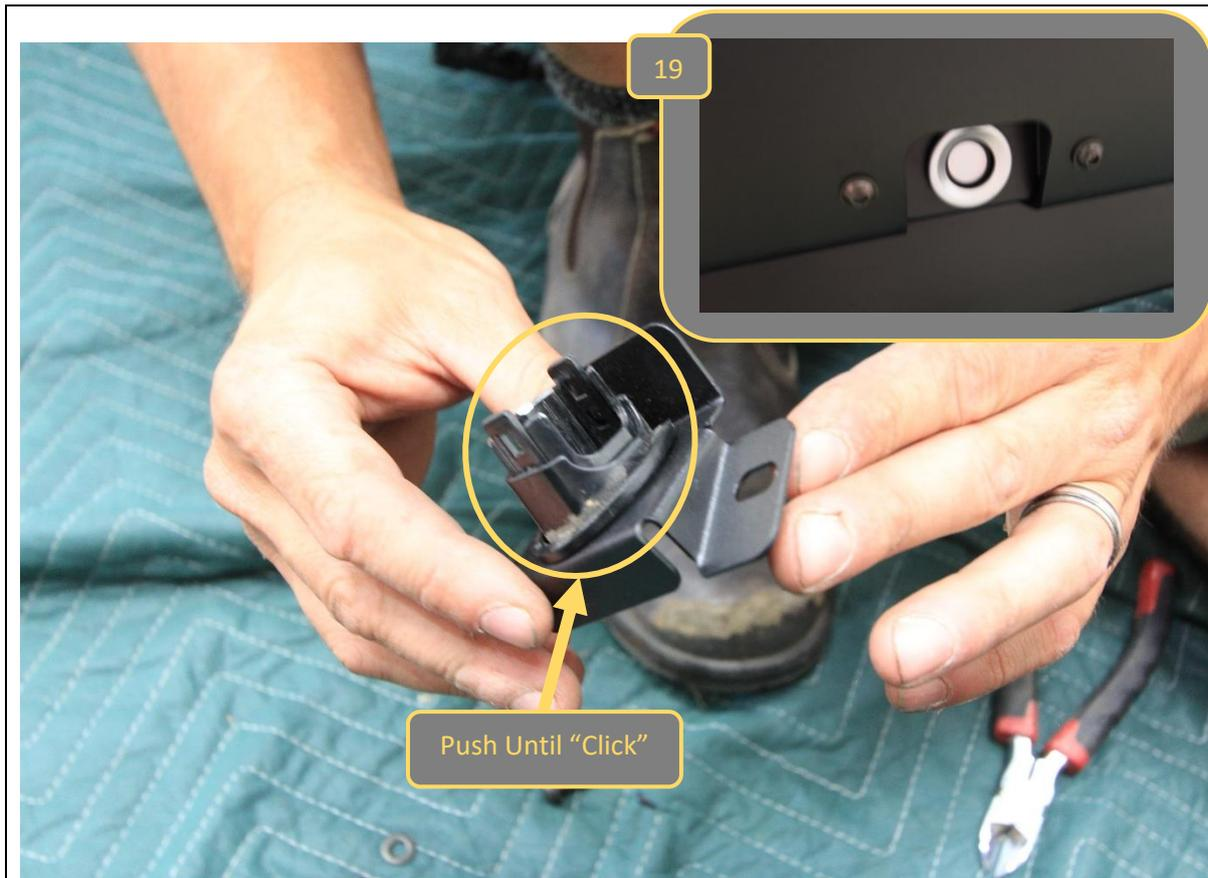
20. Fit the center housings into the sensor brackets. Insert outer housing from outside then replace inner bracket and press until an audible "Click" is heard.
