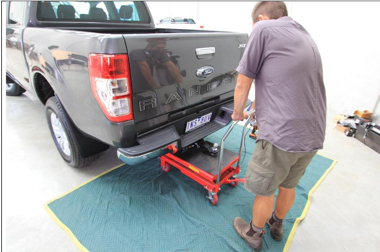
7. With all fasteners removed and the factory bar/ bumper assembly free, carefully lower, then remove from vehicle towards the back once clear of the lower tub panels
