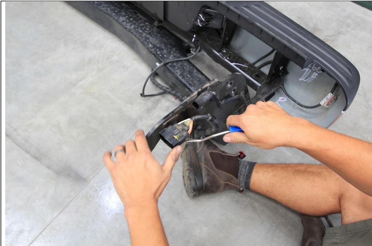
8. Remove the trailer wiring harness, by releasing all the clips securing it to the factory bar with a trim tool. Set aside for refitment to Offroad Animal bar.
