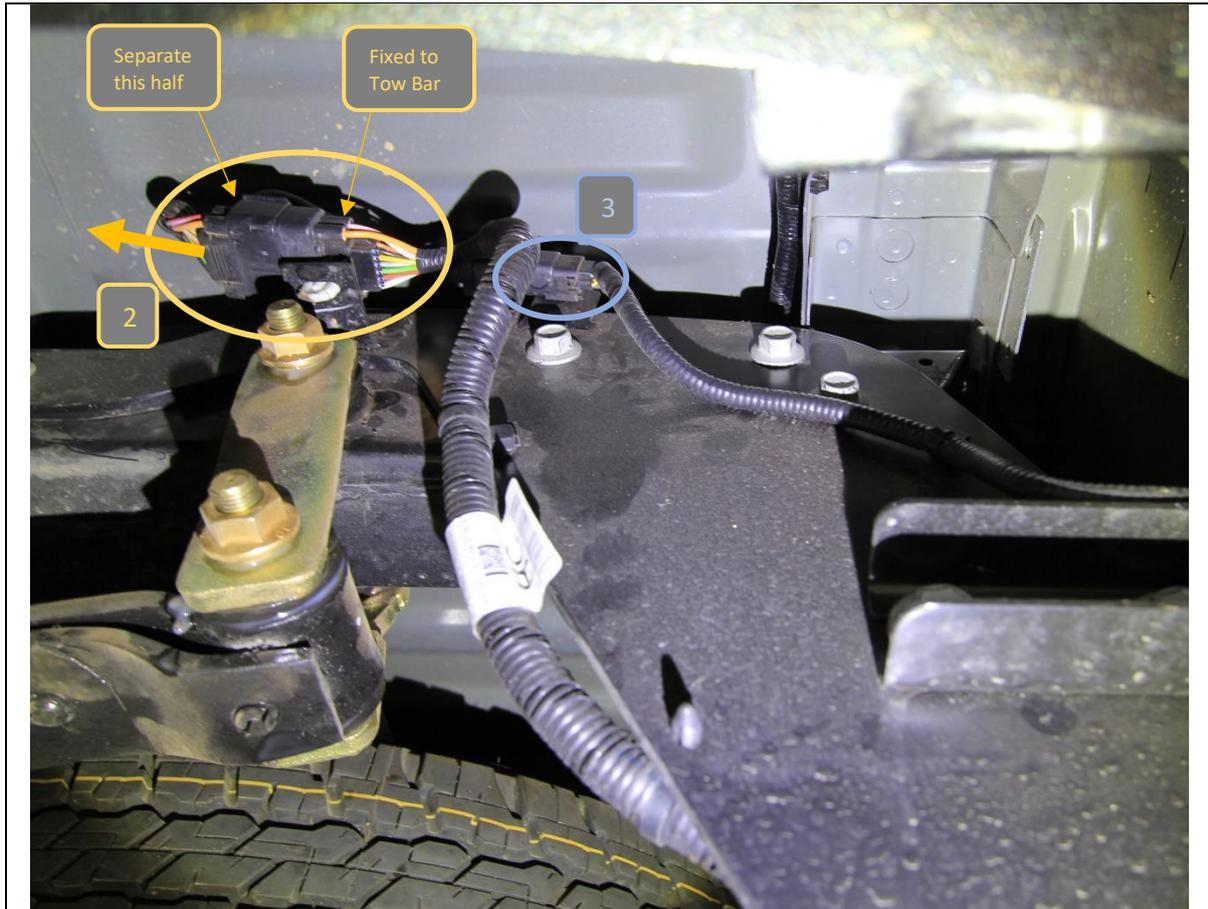
2. Disconnect the trailer wiring harness by depressing the tab on the connector and separating the half connected to the vehicle away from the fixed connector.
