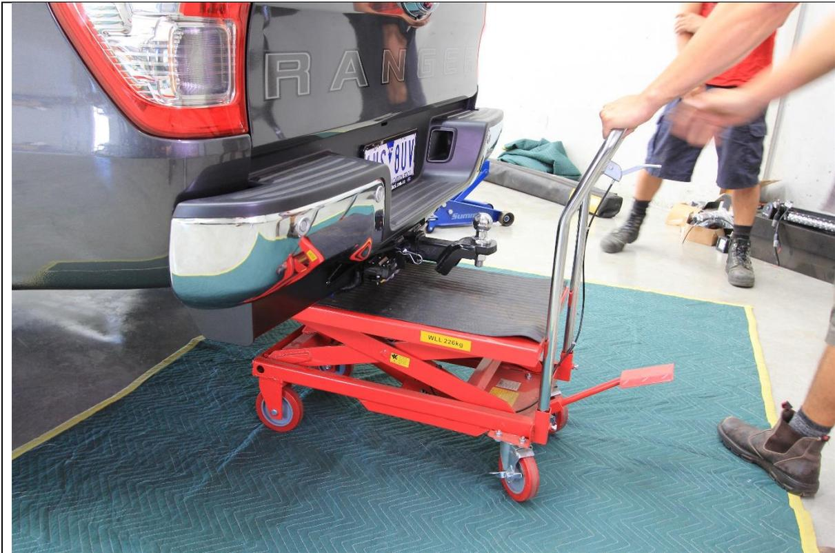
1. Before beginning work, support the factory rear bar / tow bar using lift trolley or jack.
