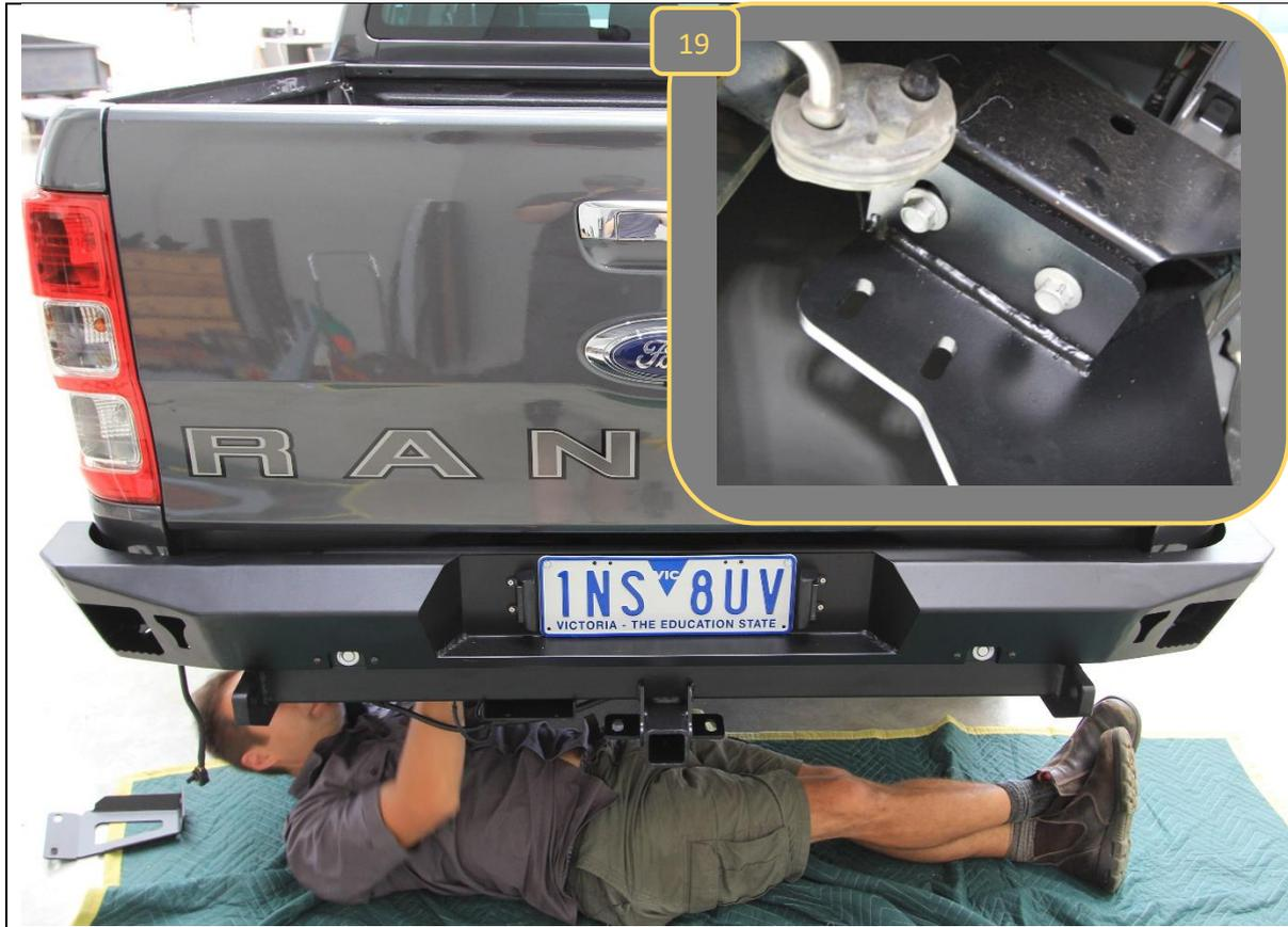
31. With assistance, from a lift trolley or another person, lift the rear bar onto the car. Tilting the bar to clear the spring hangers whilst lifting will be required.
