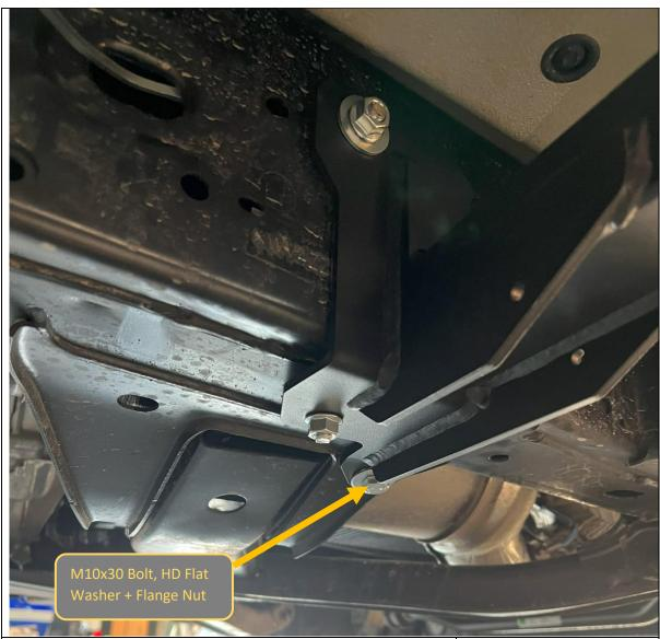
16. Once secure, finish front mount installation securing final mounting point with M10x30 Bolt, HD Flat Washer, and Flange Nut.
