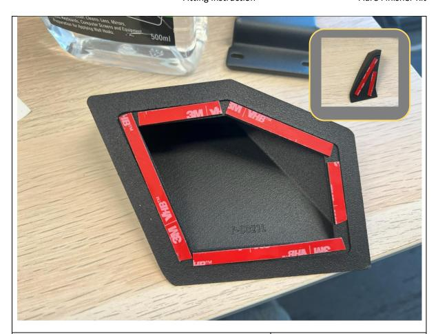
10. Using Supplied Strips of 3M VHB tape, cut and apply to the recessed bonding areas on the wing and flare finisher parts as shown.
