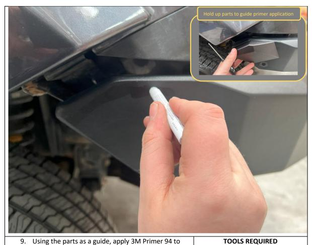
9. Using the parts as a guide, apply 3M Primer 94 to the bonding area on the end of the flare and the bulbar wing
