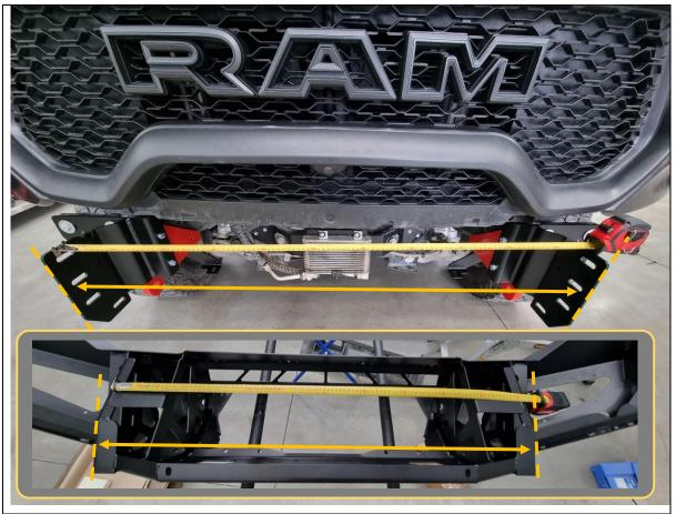
29. Measure the distance between the outside faces of uprights on bar using tape measure. Write distance below for reference if required.
