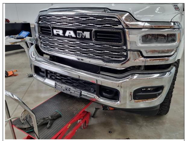
8. Pull the bumper off the vehicle and set aside in a safe place.
