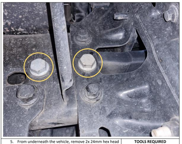
5. From underneath the vehicle, remove 2x 24mm hex head bolts securing the front tow hooks to the chassis, per side.
