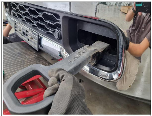
6. Pull out the loosened tow hooks through the opening in the front of the bumper.
