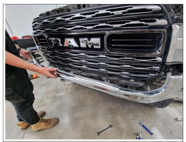
23. Remove the bottom chrome trim by pulling forwards and away from the vehicle. Set aside for reassembly.
