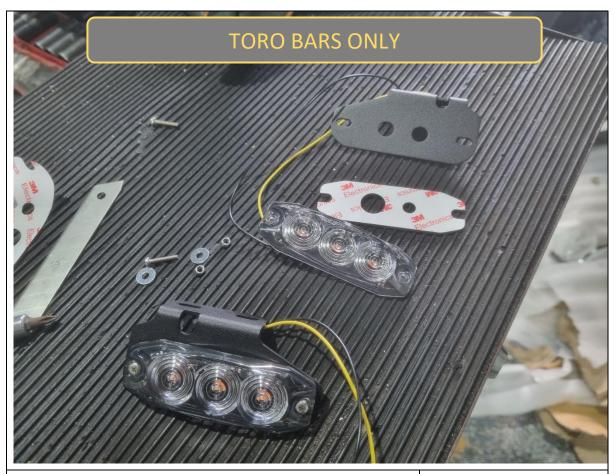
56. Fit the indicator repeater lamps to the indicator brackets, using M3 Phillips head Screws and the adhesive backing included with the lamp module.
