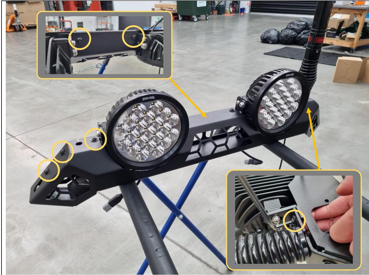
13. Loosely secure the remaining holes across the top faces with 8x M6x16 black button head bolts, flat washers and flange nuts.
