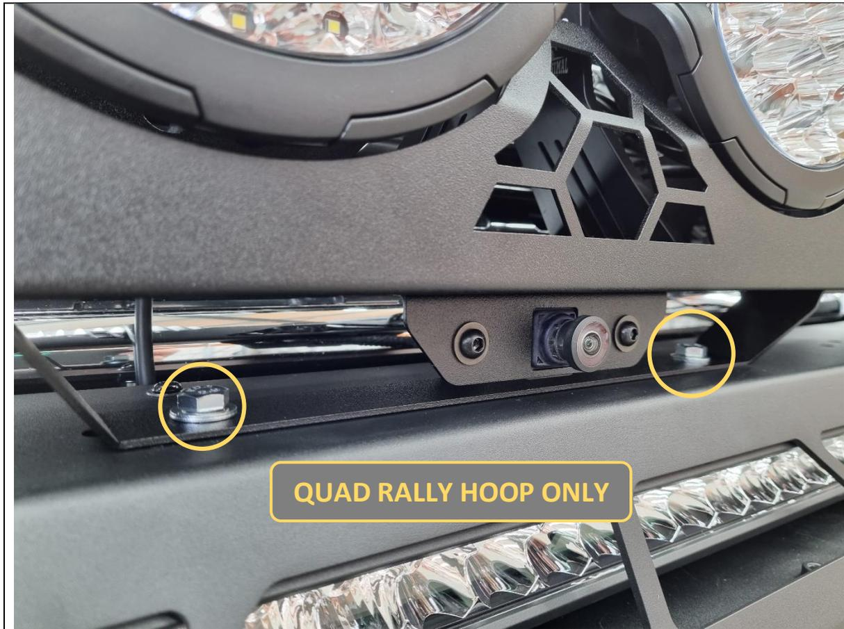
24. **Quad Rally Hoop only.** Secure the centre support to the bullbar with 2x M8x20 hex bolts, flat washers and flange nuts.
