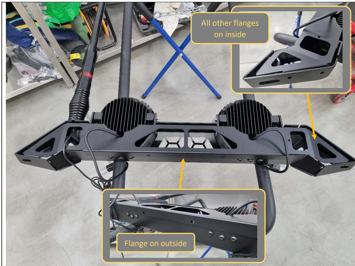
6. Insert the rear section of the rally hoop onto the back of the front section. Due to manufacturing variances, you may need to bend the flanges a little bit to get it to fit.
