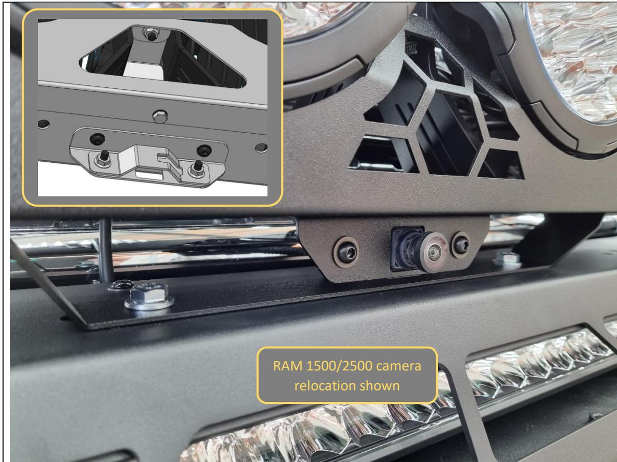
17. On some rally hoops/vehicles, there is the option to relocate the front camera onto the rally hoop, so that the view is not obstructed.
