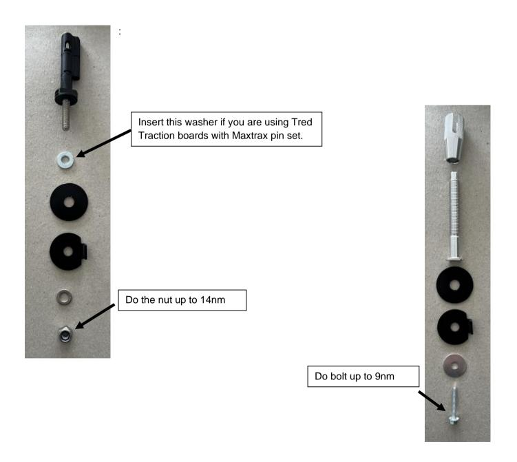
Tred mounting pins exploded view:
