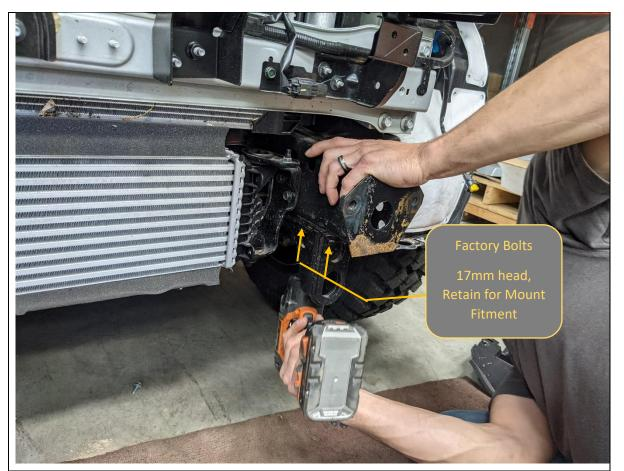
32. Remove factory tie down point from the LHS chassis rail. Retain the 17mm head factory bolts for re-fitment to bulbar mounts.
