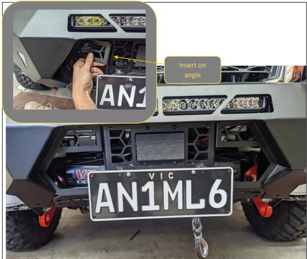
83. Fit Mesh Infill Panels. Use M8x16 Button head bolt, M8 flat washer into the captive thread in the bull bar.
