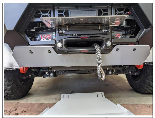
86. Fit Bash plate to the front of the bar as shown with M8 x 30 BHCS washers and flange nuts. Let hang from these fasteners at this stage.
