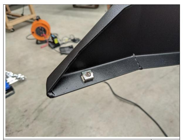
43. Fit cage nuts to bull bar by squeezing them in from above or using a flat head screwdriver to push them in
