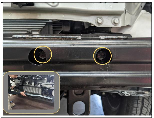
30. Remove all 4 bolts securing crash beam, then remove the impact beam.
