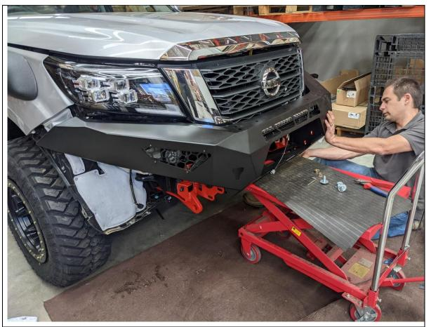
63. With the aid of a lifting table or a friend, lift bar onto vehicle
