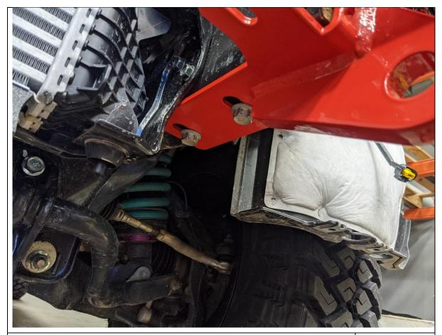
36. On LHS secure bottom of mount to nuts in chassis rail using 17mm head factory bolts removed from tie down point.
