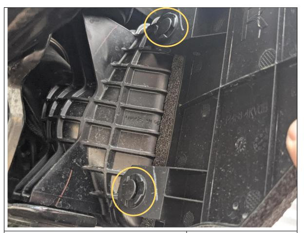
31. Remove the lower intercooler air guides by removing the 2x clips (each side) that secure them to the intercooler housing.
