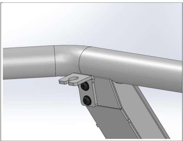
99. TORO bars ONLY. – If fitting an antenna, fit the antenna brackets to the upright using Supplied M8x20 Button head bolts and M8 Black Flat Washers
