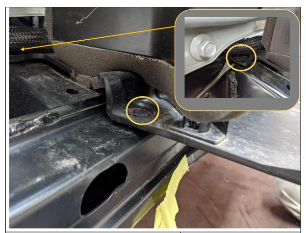
27. Remove lower air guide by removing 4 clips; 2 front (Main Image) and 2 rear (Inset image).
