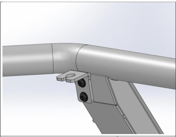
101. TORO bars ONLY. – If fitting an antenna, fit the antenna brackets to the upright using Supplied M8x20 Button head bolts and M8 Black Flat Washers
