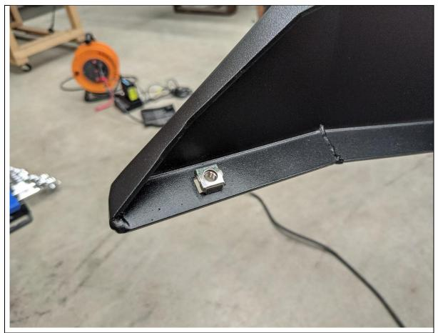
43. Fit cage nuts to bull bar by squeezing them in from above or using a flat head screwdriver to push them in
