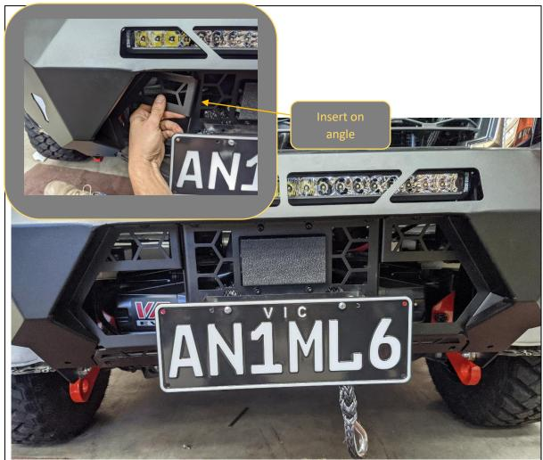
85. Fit Mesh Infill Panels. Use M8x16 Button head bolt, M8 flat washer into the captive thread in the bull bar.
