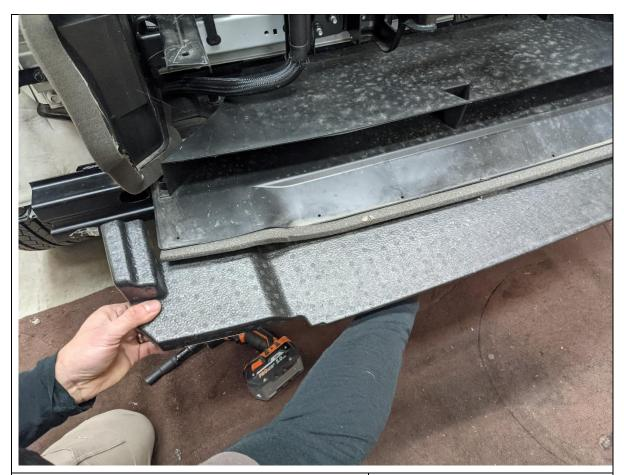
21. Remove and discard foam impact absorber from the front of the impact beam. Just pull off.
