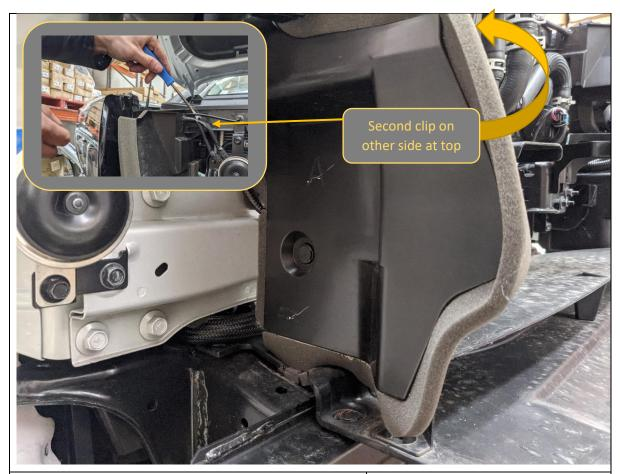
22. Remove and retain upper air guides. These are secured with 2x clips. These will be modified and refitted.
