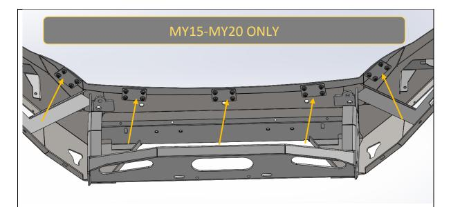
54. Fit the Infill panel to the back top edge of the bar, using the suppled M6x16 Back Button head Screws, Flat washers and Flange nuts.
