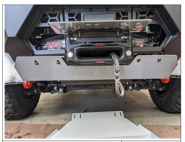
88. Fit Bash plate to the front of the bar as shown with M8 x 30 BHCS washers and flange nuts. Let hang from these fasteners at this stage.
