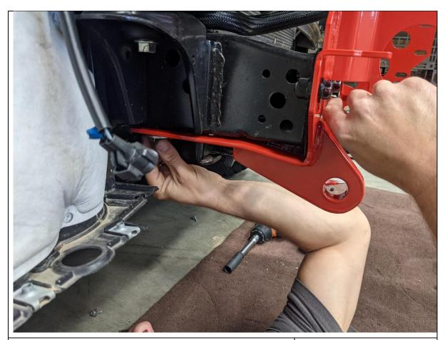
37. On RHS, secure mount to bottom of chassis rail using M12x30 Hex bolts, Flat washers and M12 Nut Plates inserted through front of chassis rail.
