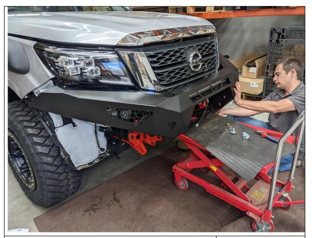
64. With the aid of a lifting table or a friend, lift bar onto vehicle
