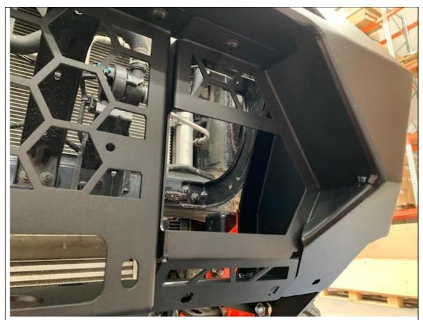
34. Fit side panels as shown with M8 button head cap screw washer and flange nut. Leave bottom holes open at the moment
