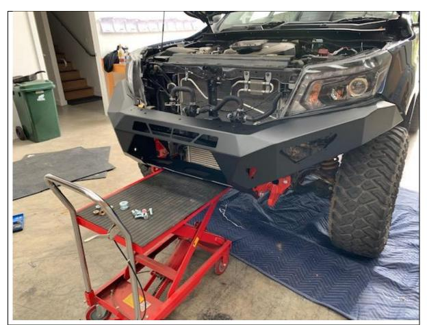
28. With the aid of a lifting table or a friend, lift bar onto
