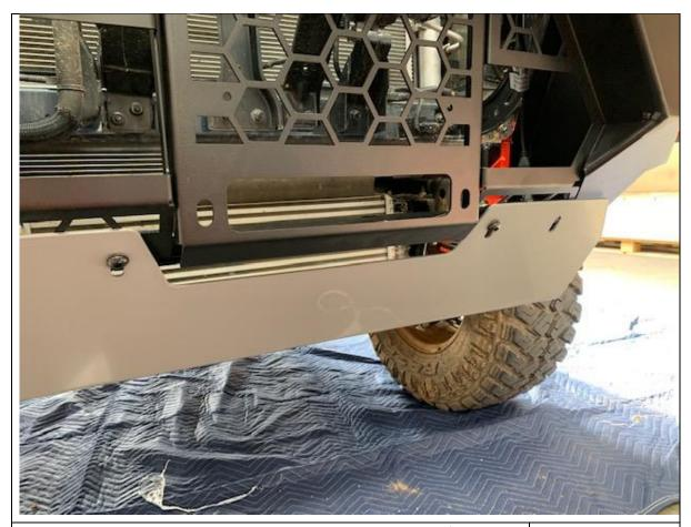
56. Fit Bash plate as shown with M8 x 30 BHCS washers and flange nuts. Leave off bottom bolts
