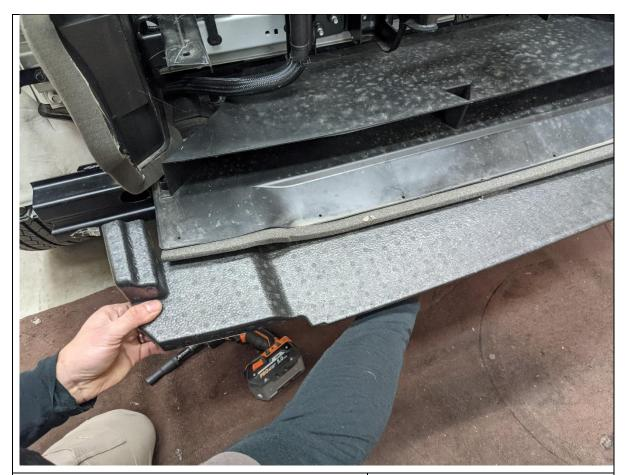
21. Remove and discard foam impact absorber from the front of the impact beam. Just pull off.
