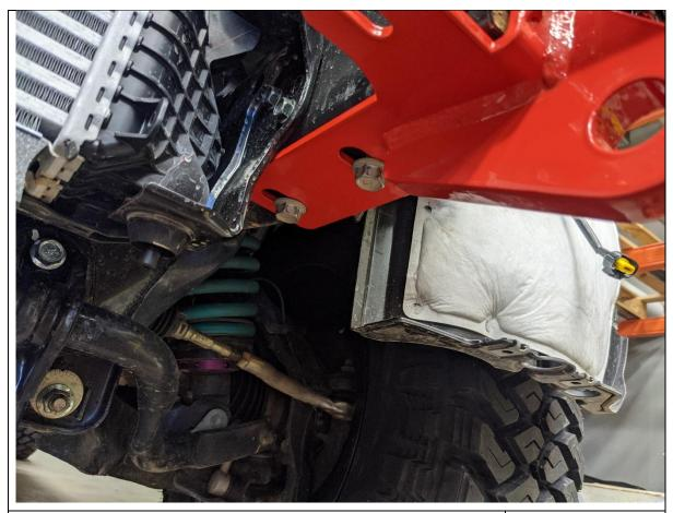
36. On LHS secure bottom of mount to nuts in chassis rail using 17mm head factory bolts removed from tie down point.
