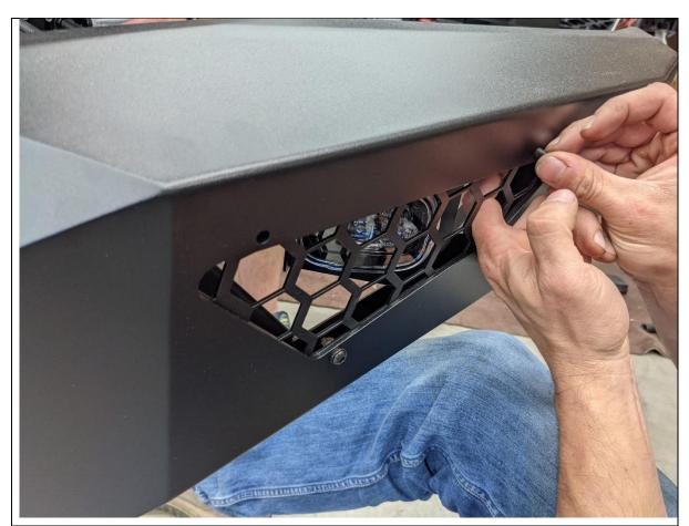
48. Fit Mesh light covers to the bar, using supplied M6x16 Black button head screws, Flat washers, and Flange nuts.
