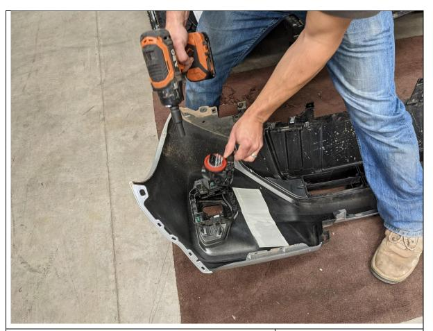
44. Remove fog lights from bumper by removing the 4x Phillips head screws securing them.
