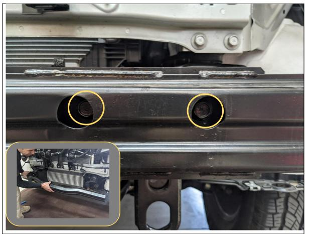
30. Remove all 4 bolts securing crash beam, then remove the impact beam.
