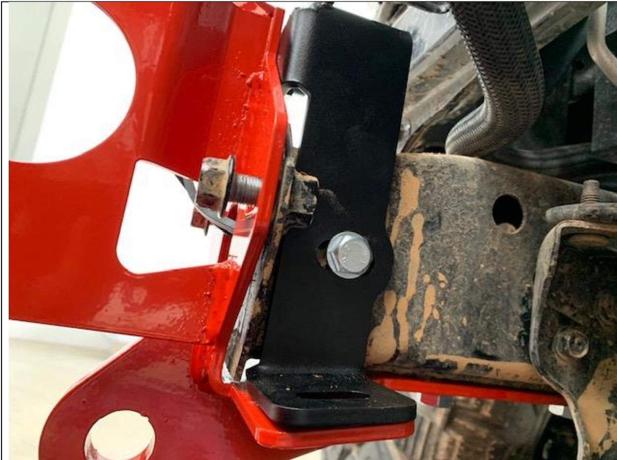
21. Fit Chassis brace as shown
