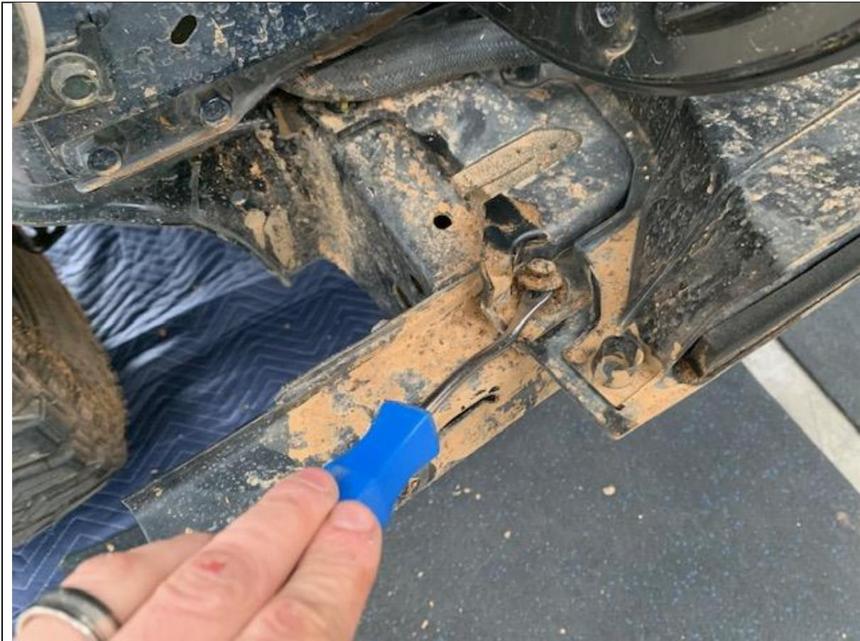
13. Remove lower air guide by removing 4 clips; 2 front (above) and 2 rear(below)
