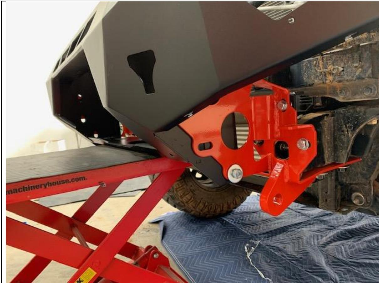
29. Place at least 2 bolts in mounts to secure bar and check fitment left to right of bar on vehicle. Once happy torque down all chassis mount bolts. Use flange nuts for these and do up finger tight
