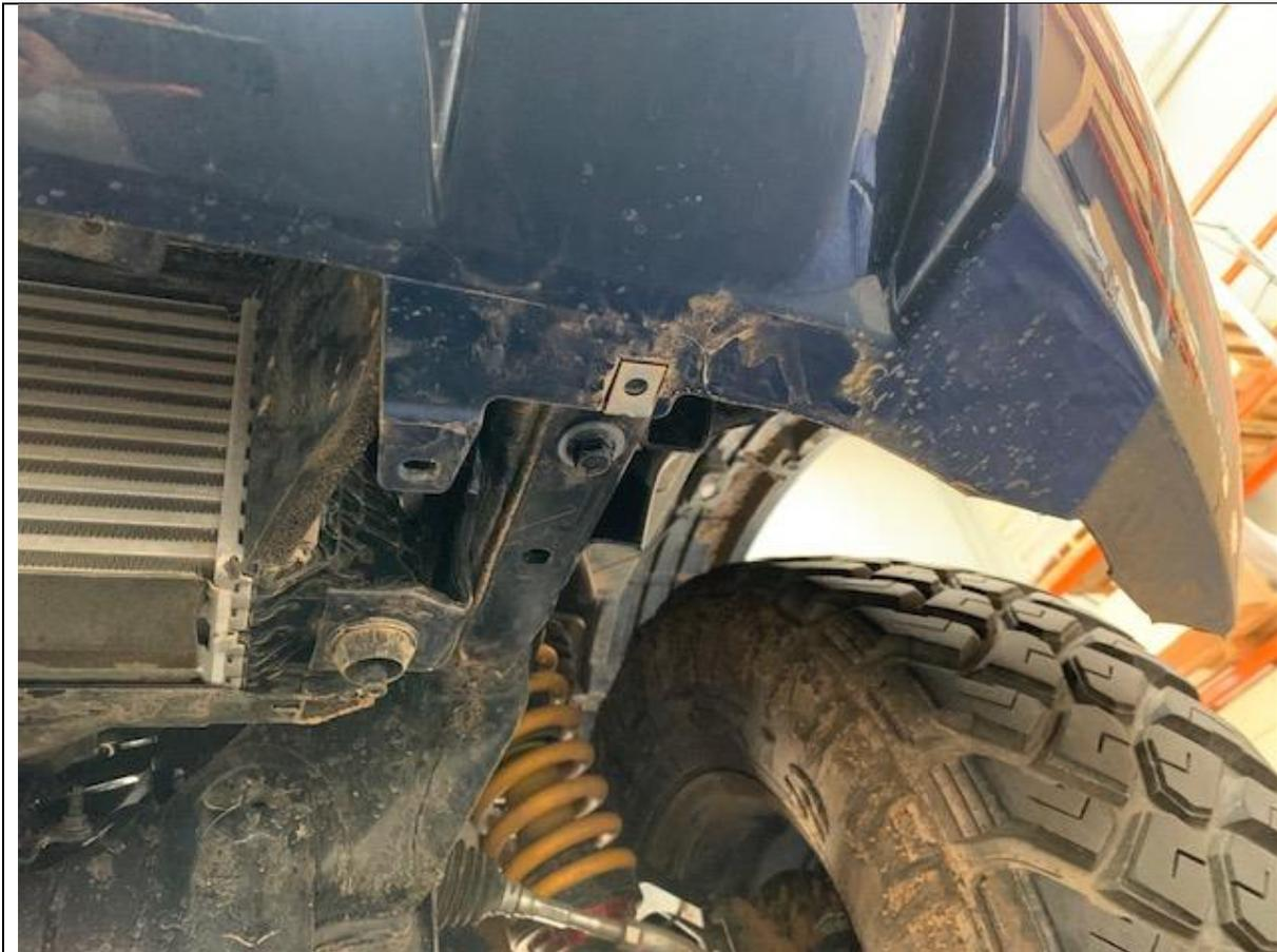
5. Remove factory bash plate and lower panels under bumper
