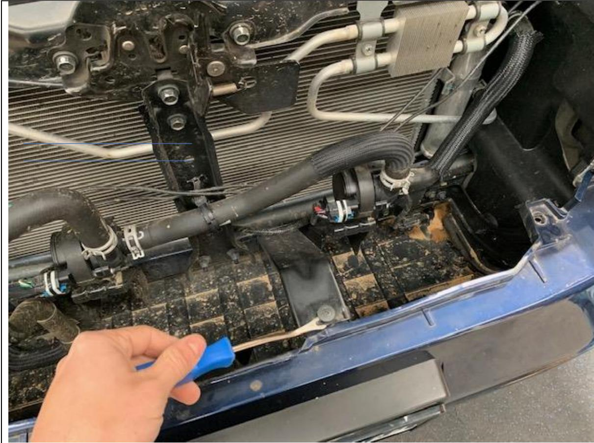
7. Remove all clips securing centre of bumper to vehicle
