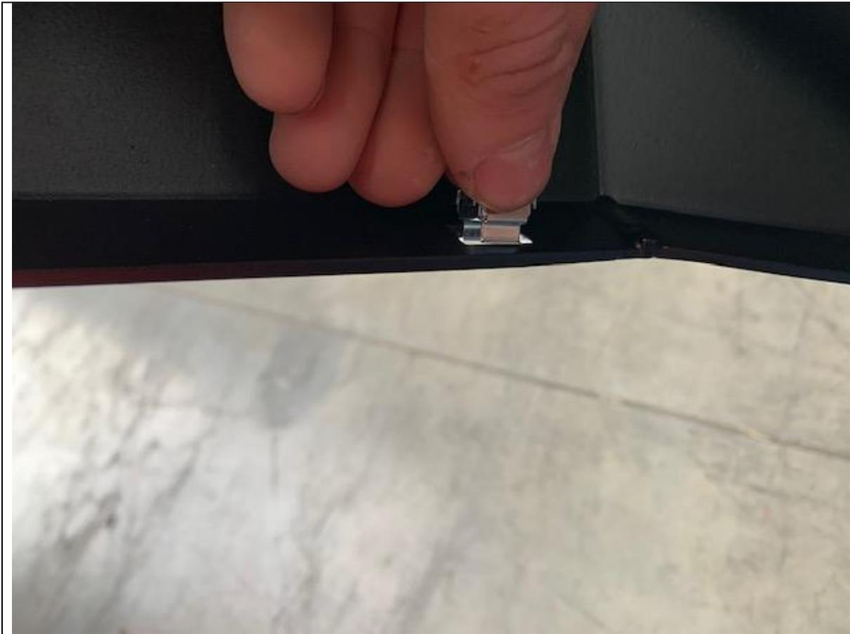
25. Fit cage nuts to bull bar by squeezing them in from above or using a flat head screwdriver to push them in
