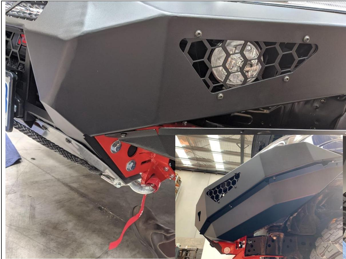
51. Fit mesh panels M-0002R/L to bar with fog light with M6 Hardware. If no fog lights used simply fit Mesh panel to bar with M6 hardware
