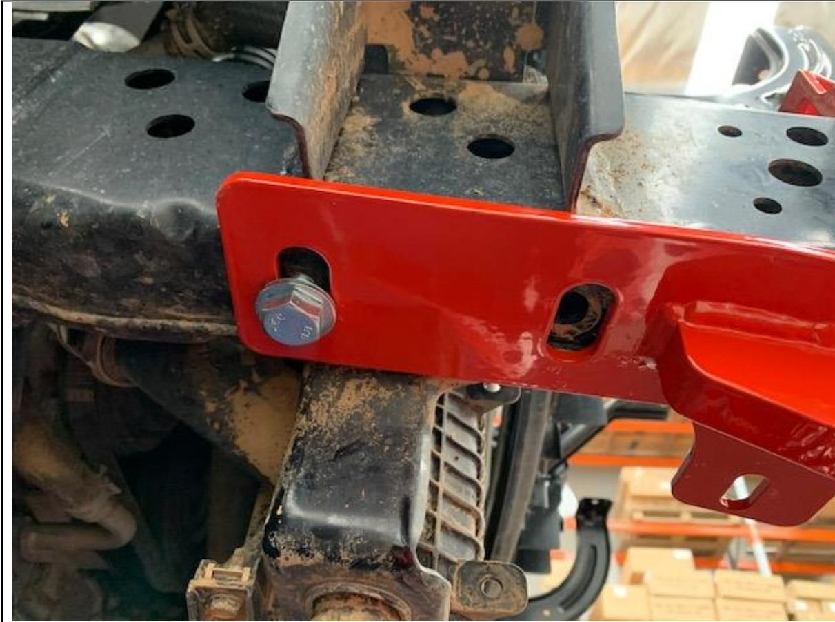
19. On Right hand side you will need to feed nut plates through to secure with M12x40 bolts
