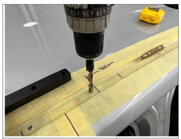
48. Before drilling, check underside of drill locations for any obstructions. Un clip wiring harnesses or similar as required to ensure breakthrough area is clear and drill will not damage anything in the roof.
