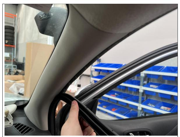
21. Release door rubbers and peel back to past the level of the beige portion of the pillar trim panels.
