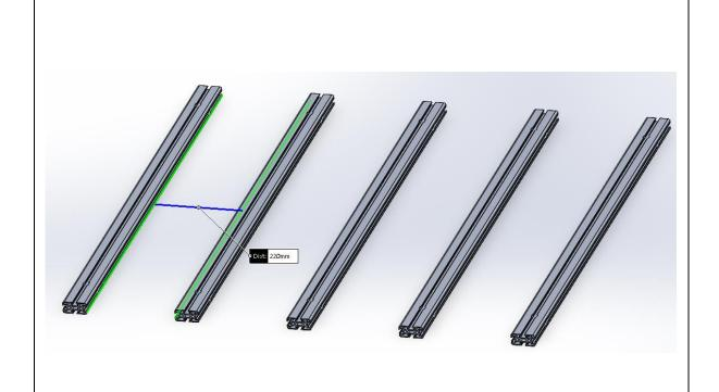
62. Next Assemble the roof rack. Start by setting out the 5 extrusions on a table. Position them so they sit approximately 220mm apart.
