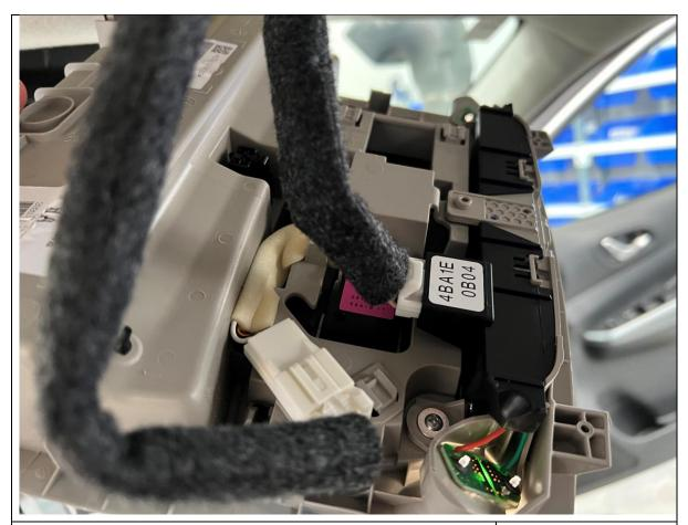
18. Disconnect the wiring harness connectors from the back side of the roof panel.
