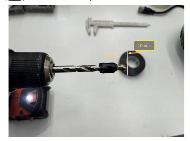
46. Insert 9mm drill into electric drill
