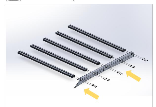
63. Fit the side rail to the extrusion,
