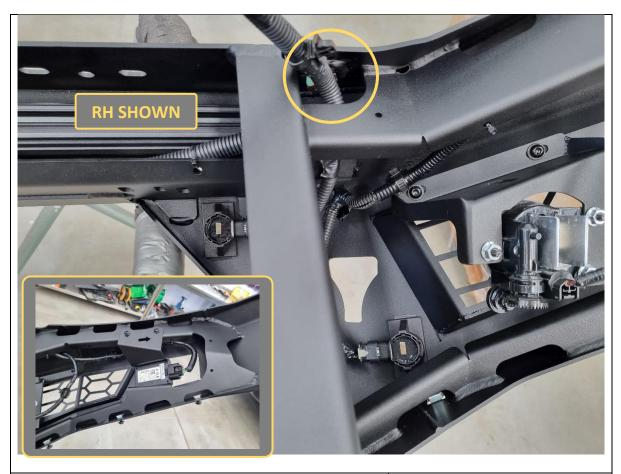
100. Remove backing film on VHB tape (easier with knife to peel off) and adhere parking sensors in position in bar. Apply pressure for at least 10 seconds after positioning for best adhesion.
