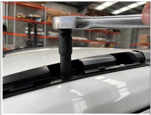
11. Remove the front and rear track bolts, using 12mm socket or spanner.
