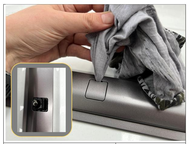
9. Using a Rag covered flat screwdriver to prevent marking of roof rail, unclip the plastic access covers at for the two center roof rail mounts, uncovering the forward center rail bolts
