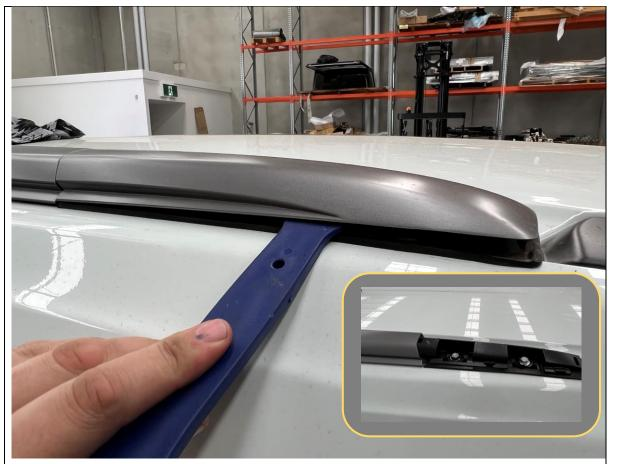
10. Using a plastic trim tool to prevent marking of roof, unclip the plastic cover at the rear end of the roof rail, uncovering the back roof rail bolts
