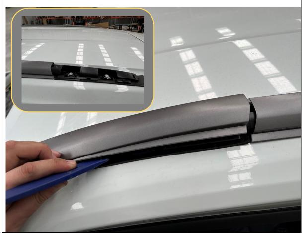
8. Using a plastic trim tool to prevent marking of roof, unclip the plastic cover at the front end of the roof rail, uncovering the forward roof rail bolts
