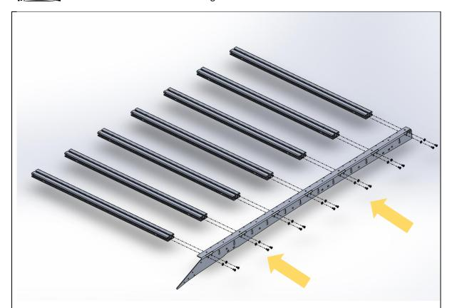
17. Fit the side rail to the extrusion,
