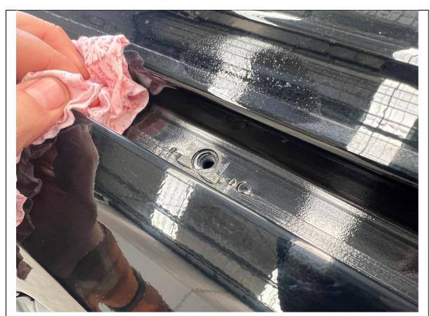
33. Clean the area around all of the mounting points with isopropyl alcohol or wax and grease remover solvent to ensure a good sealant bond.
