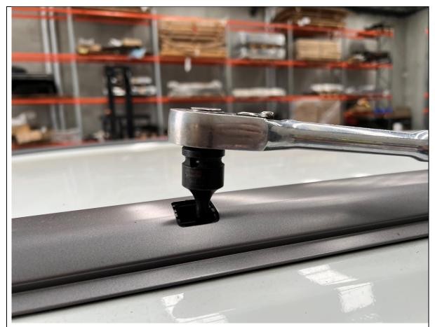
12. Remove the Center track bolts, using 5mm Hex key or hex key socket or
