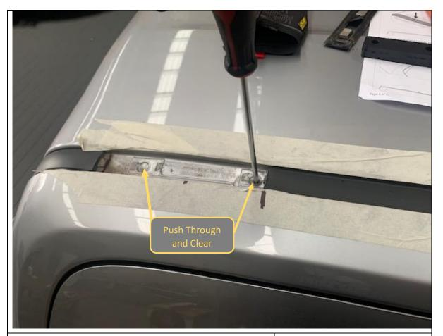
6. Using a small screwdriver or pick, push through the factory sealant patches covering the threaded mounting points in the roof.
