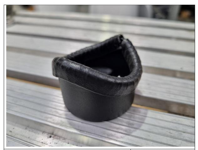
67. Fit supplied pinch weld around the curved edge of the spigot. Trim with side cutters if oversized.
