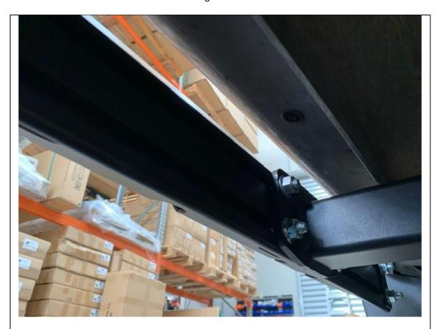
47. With the help of a friend or mate, lift step and extrusion up to brackets. Align all the bolts so they fit through the corresponding holes in the brackets.
