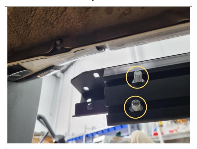
51. Slide in 2x M10x25 hex bolts into the front open end of the extrusion as shown.
