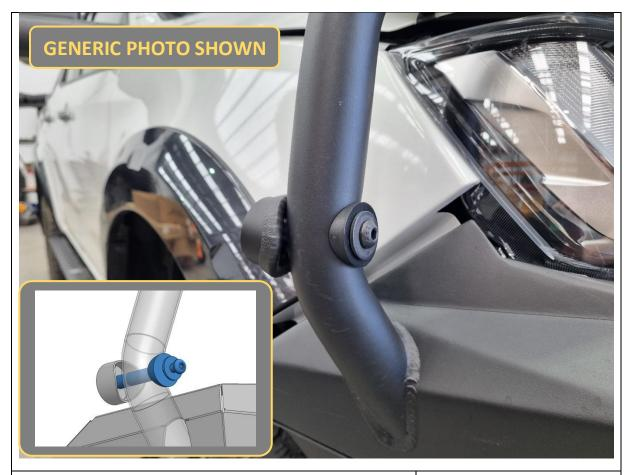
68. Loosely position the spigot with the Toro bar and hold in place with 1x M10x100 black button head, flat washer, nylon saddle washer and crush tube, through the 18mm drilled hole in the bar.
