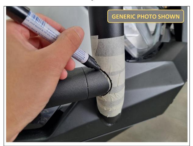
59. Using a marker pen, trace the outline of the spigot in position onto the Toro bar tube.
