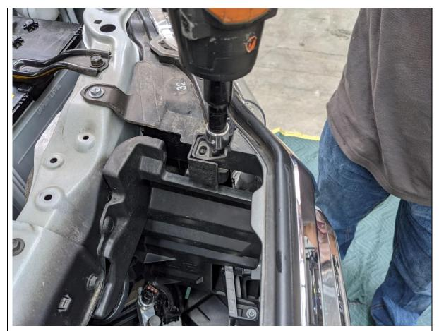
4. Remove the 2x Bolts securing top grille to body using 10mm socket.
