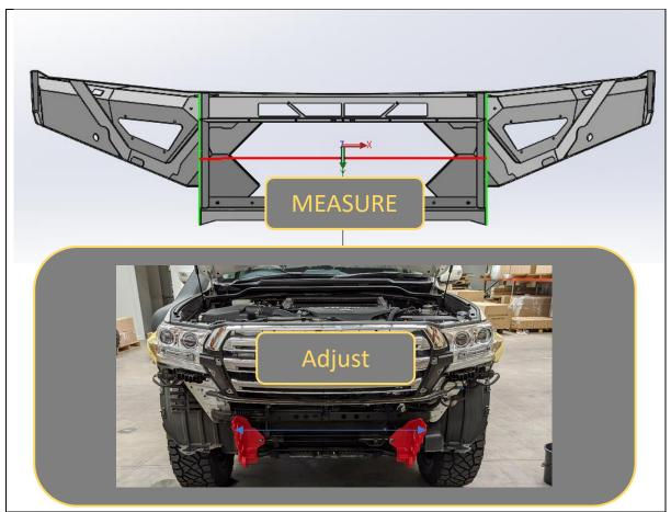
48. Measure Distance between outside edges uprights on bar using tape measure. Write distance below for reference if required.
