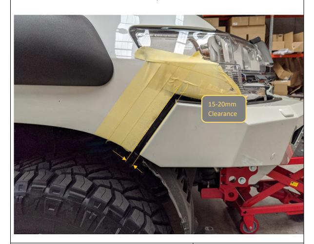
67. With assistance, from another person, Align the bar with the edges of the vehicle. Adjust such that the clearances are neat and even side to side.
