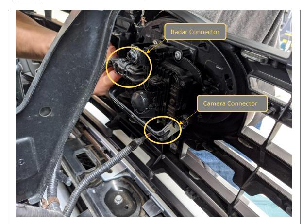
13. For Vehicles equipped with Adaptive cruise radar sensor and / or front camera, Disconnect the electrical harness connectors located on the back of the sensors.
