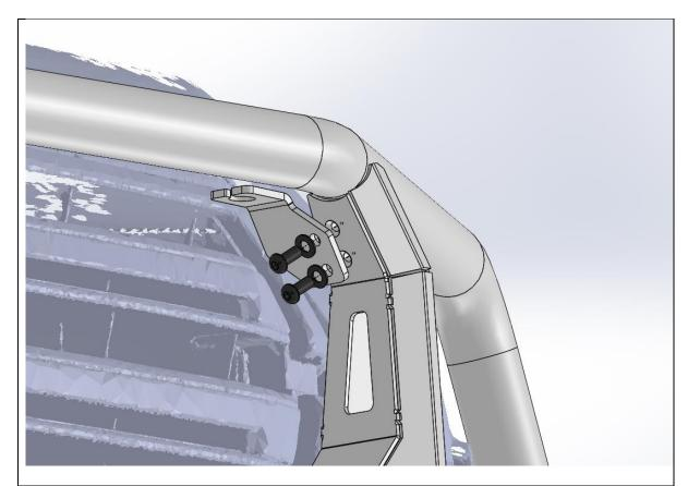
106. If fitting antenna to Torro bar, fit the antenna brackets to the M8 Threaded inserts in the uprights. Note that brackets are handed.
