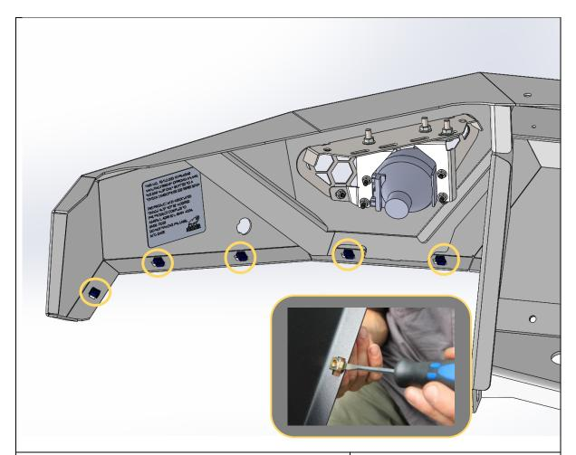
56. Fit 5x Cage nuts from small parts kit to rectangular slots in bottom of wing.
