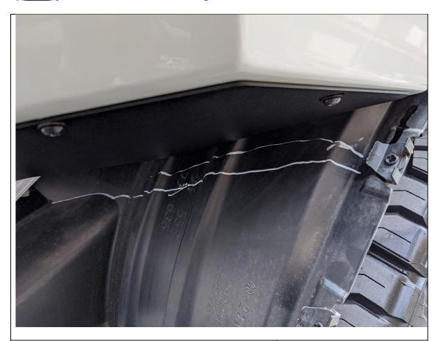
101. Using the edge of the under panel as a guide mark the wheel arch liner, approximately 15mm beyond the intersection of the under panel.
