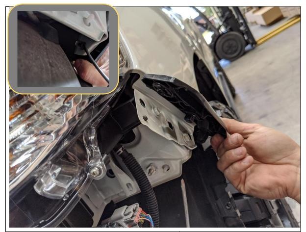
32. Remove the plastic bumper retainers by removing the Philips head screw, then prying out the large clip from behind using trim tool
