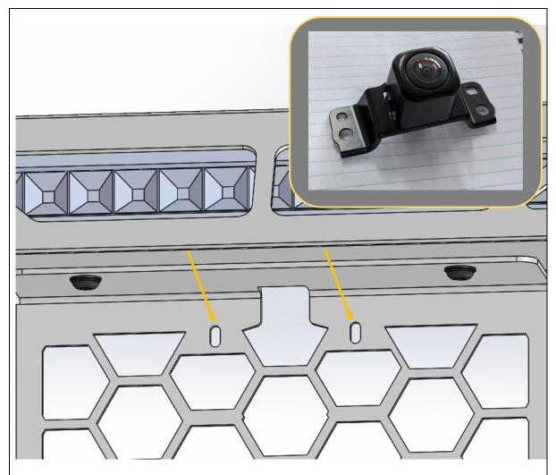
78. If vehicle is fitted with front camera, the bar will obscure bottom part of front camera image.
