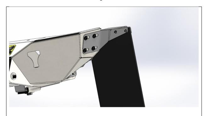
16. If fitting Optional mud flap brackets, position bracket as shown with M8 BHCS and flange nuts with washers
