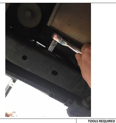
4. While still underneath remove 2 x M10 bolts as shown, and loosen M10 bolts further up on same bracket
