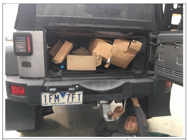
3. Climb underneath and disconnect loom for rear number plates
