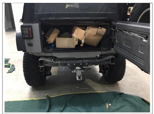
7. With bumper removed open rear door before putting new bar on
