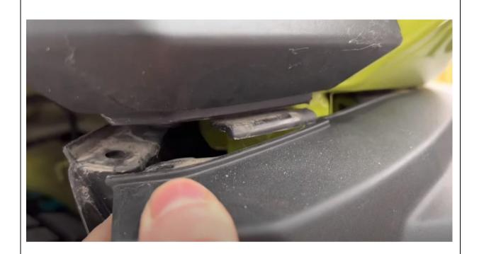
6. Peal edges of bumper just free from retaining clip at the edge under the flare.
