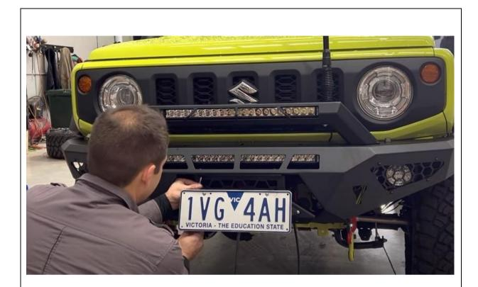
55. Install centre mesh plate with M8 x 16 BHCS blk and flat washers, x 3 in top gusset. Leave bottom bolts off for now
