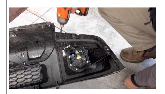
19. Remove fog lights from bumper with Phillips head screwdriver.
