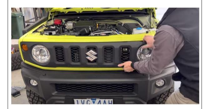
Gently pull grill away from body enough that will allow you to disconnect the indicator loom. LHS of vehicle you should be able to reach in the bonnet area to do this before grill is removed **TOOLS REQUIRED**
