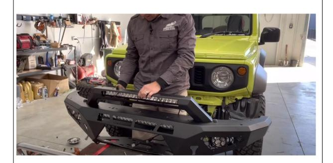
41. If fitting a top hoop do so now with provided hardware, and fit the light
