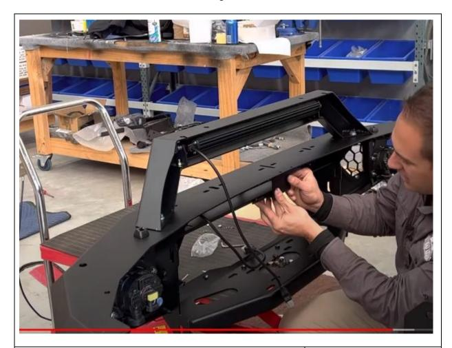
42. Fit pan brace as shown with M6 hardware, 4 of each
