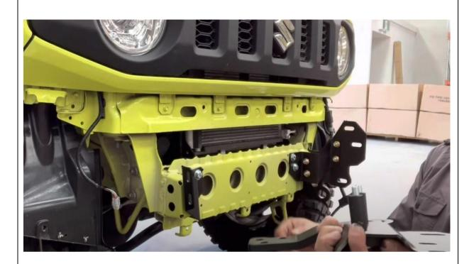
25. Fit inner chassis bracket as shown, with M10 x 30 bolts, flat washer and a flange nut inside chassis through large hole. Leave hand tight.
