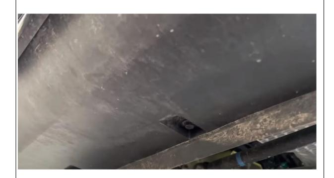
5. Underneath front, remove 3 screws holding splash guard onto chassis
