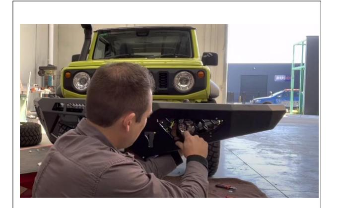
39. Fit mesh panel with lights to bar and secure with 4 x M6 x 16 BHCS BLk, M6 FW and M6 FN
