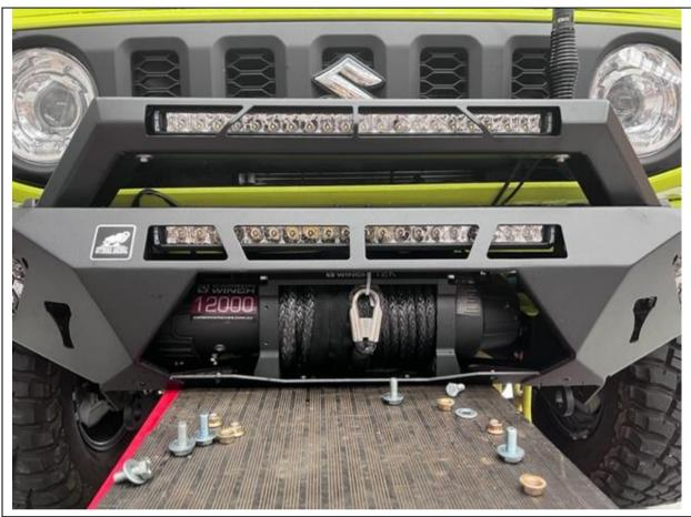
46. Using a lifting table, trolley jack or a strong mate lift the bar and winch onto the vehicle and secure with M10 x 30 bolts, flat washers and Nyloc nuts
