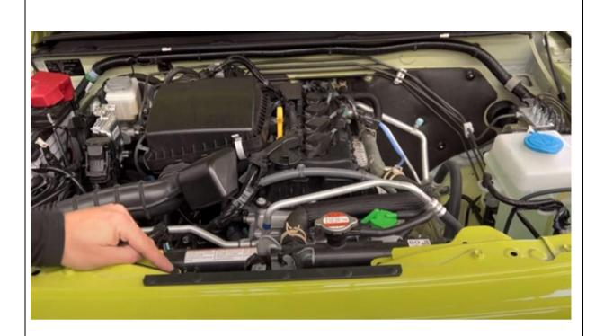
7. With bonnet open remove 3 x clips holding grill onto the body
