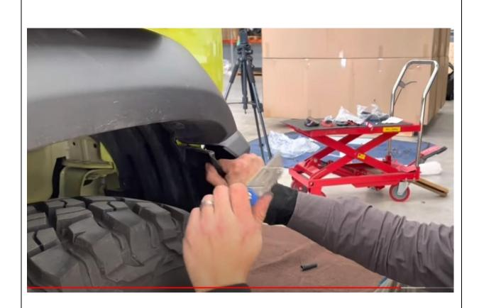
48. Using a sharp blade trim the wheel well liner to suit the bar.
