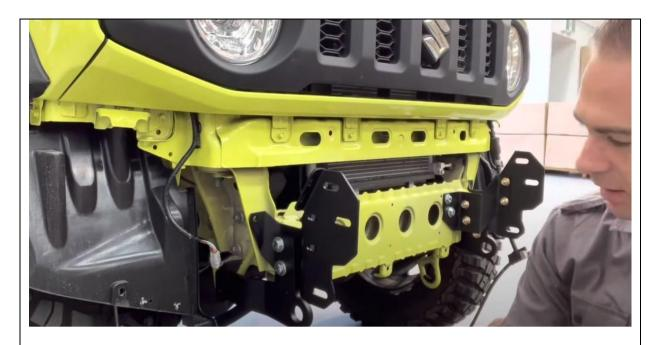
26. Doing a stack of parts, you'll take the M10 x 80 bolts, through flat washer, then tow hook, then outer chassis bracket, then crush tubes and put all of this through the large holes just drilled. Secure with flange nuts on the inside chassis bracket, and leave hand tight
