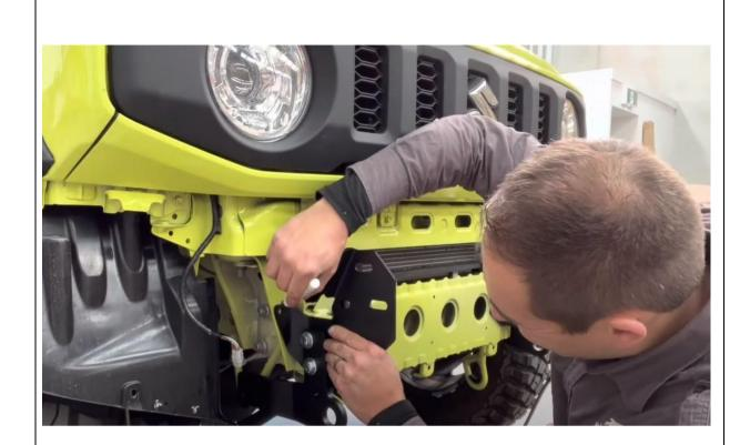
27. Put a centre hole as shown, then remove outer chassis bracket an centre punch the marked hole
