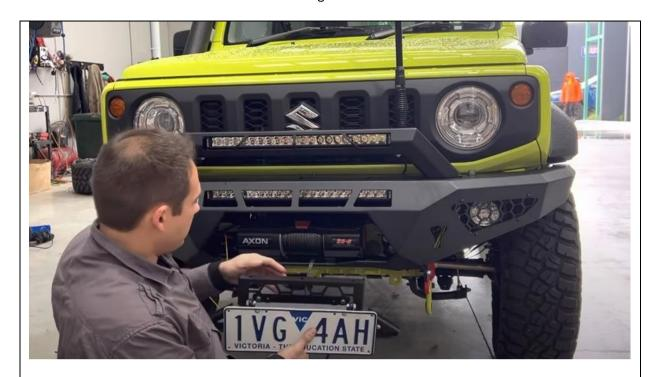
54. Remove number plate from factory bumper and fit to number plate flip
