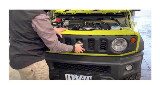
13. Refit the grill using all but the last 4 clips you just removed in step 12
