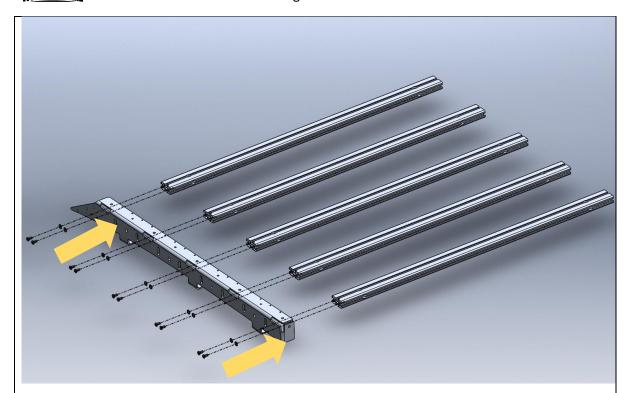
4. Fit the side rail to the extrusion,
