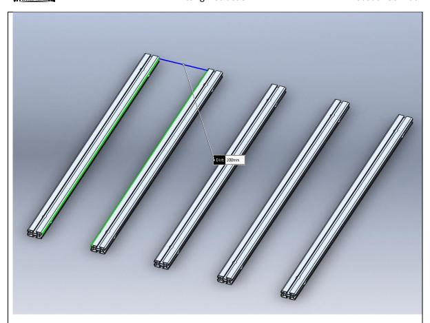
3. Next Assemble the roof rack. Start by setting out the 5 extrusions on a table. Position them so they sit approximately 200mm apart.
