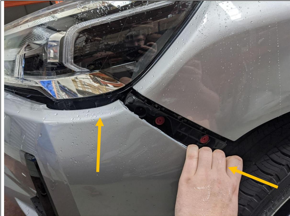
12. Remove the bumper. Start by pulling from the outside where the bumper meets the wheel arch and work towards the center from both sides.
