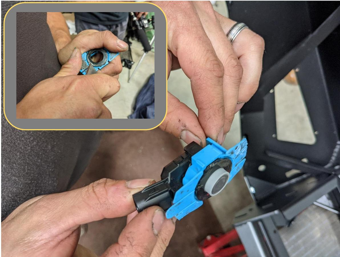
51. Remove remnant adhesive from the face of the sensor housing, using a utility knife and / or solvents.
