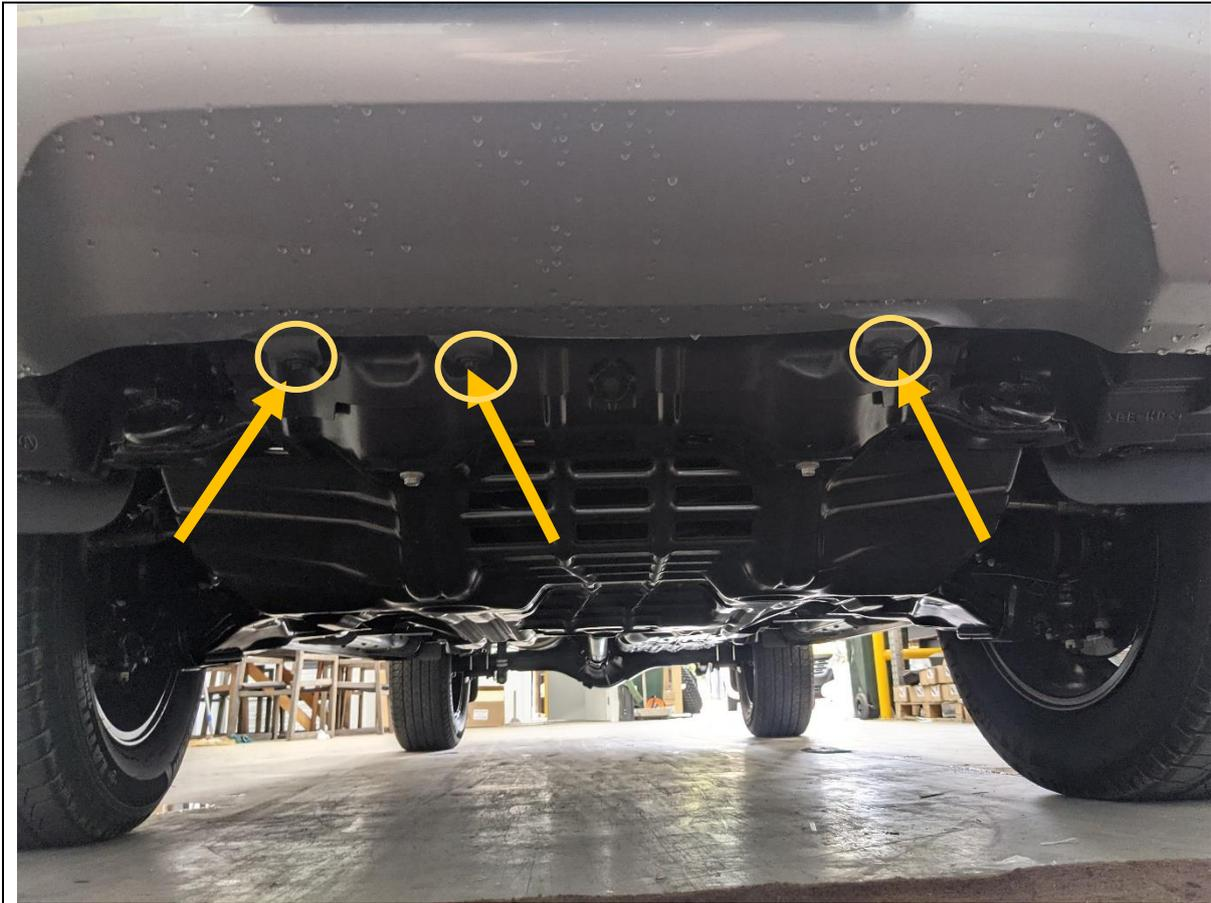
10. Remove the 3x 10mm head Screws securing bottom center section of bumper to inner wheel arch liner.
