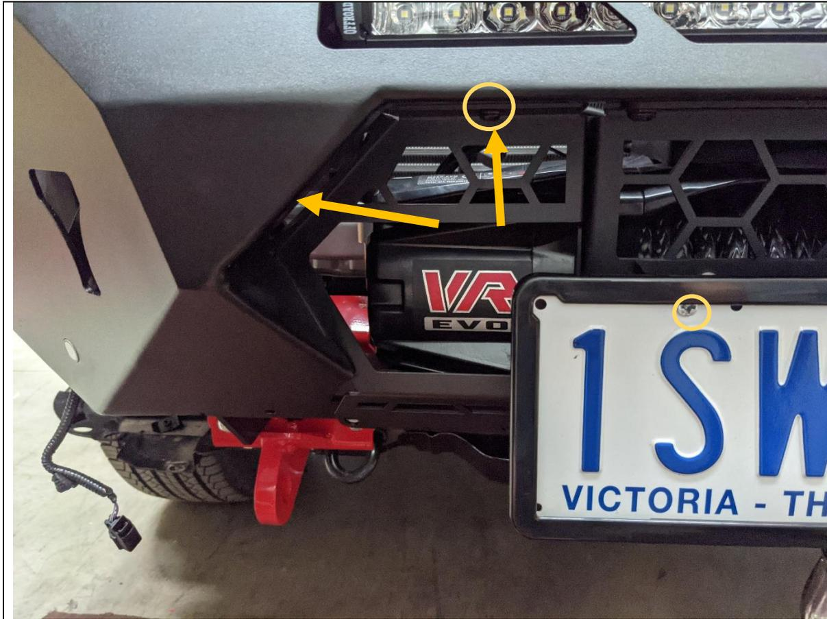
79. Fit the side mesh panel to the bar, using only the top and side points at this stage. Secure with 2x M6x16 Black Button head, bolts, Black M6 Flat washer and flange nut.
