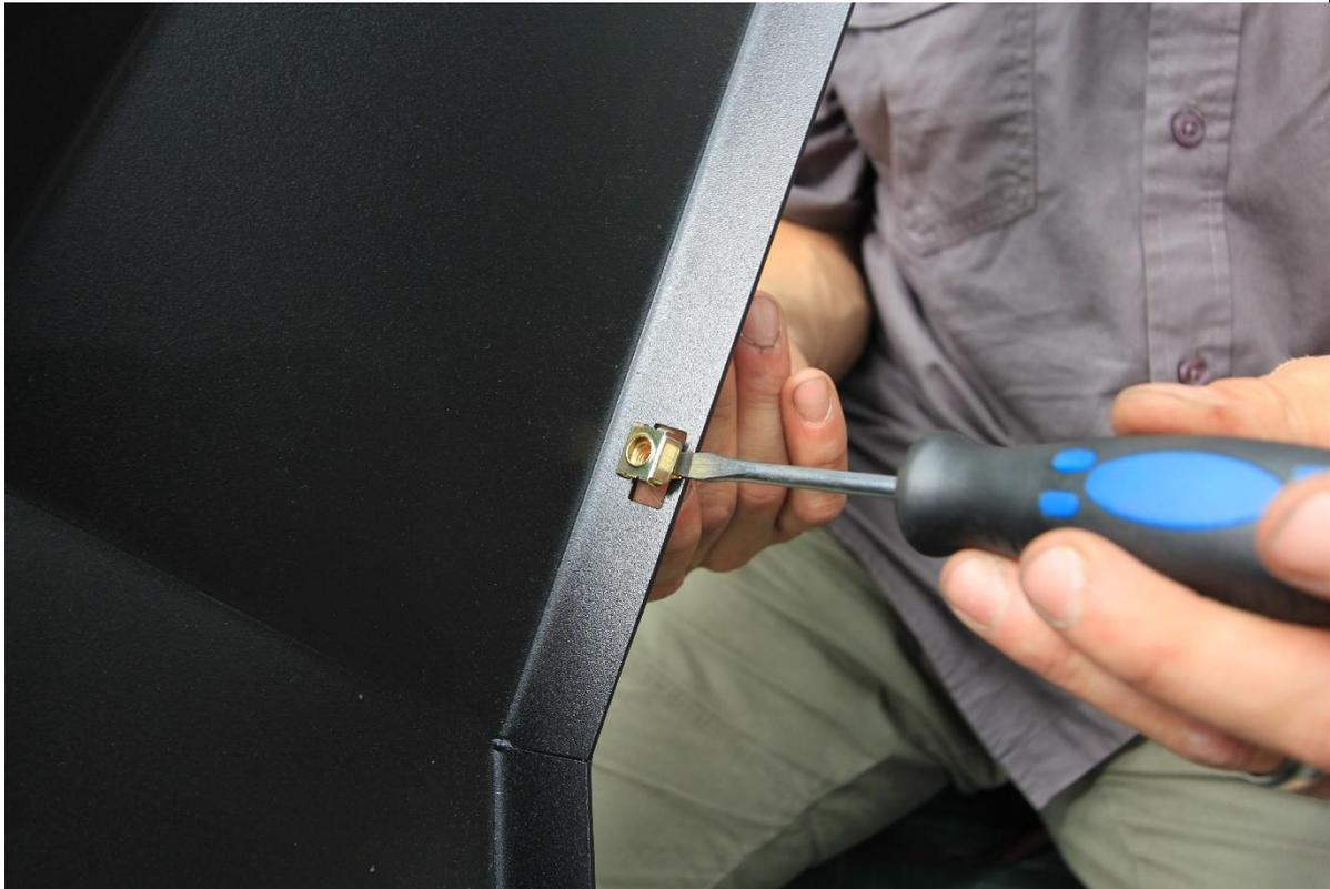
67. Insert cage nuts to square slots in bottom of wings. Seat cage nut against one edge of slot then push other edge in with flat bladed screwdriver.
