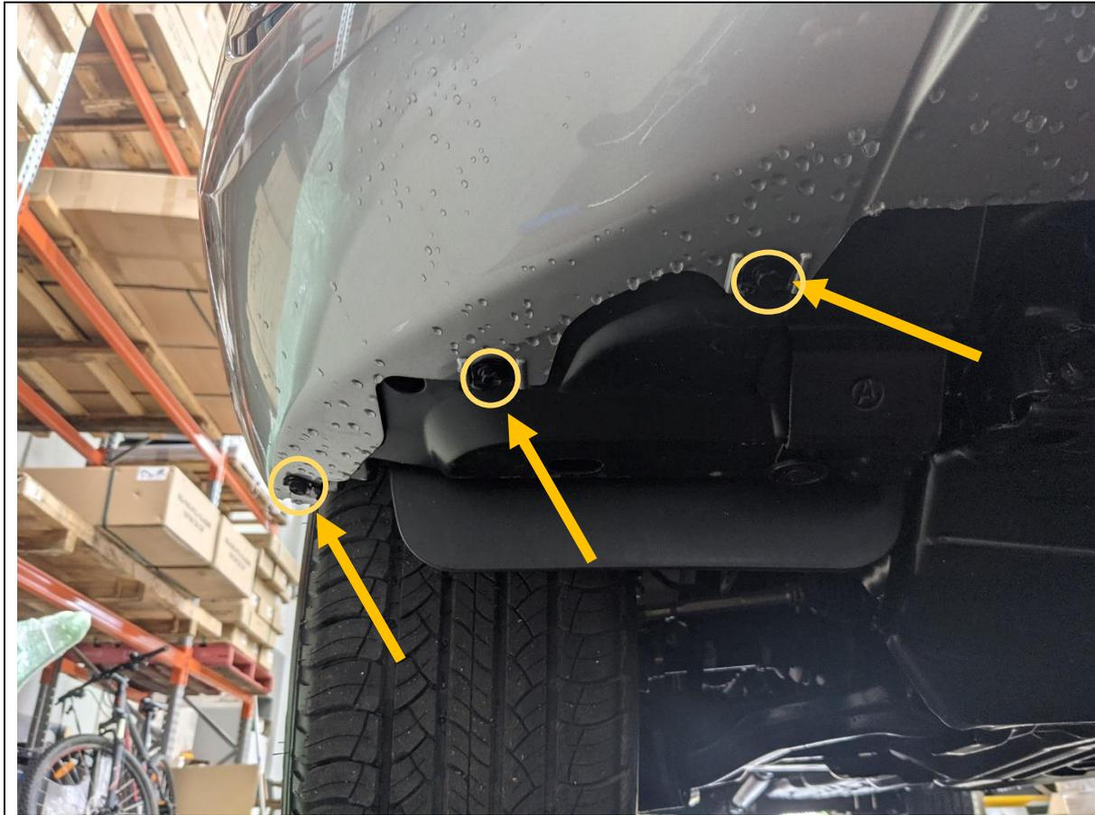
8. Remove the 3x 10mm head Screws securing bottom corner of bumper to inner wheel arch liner.
