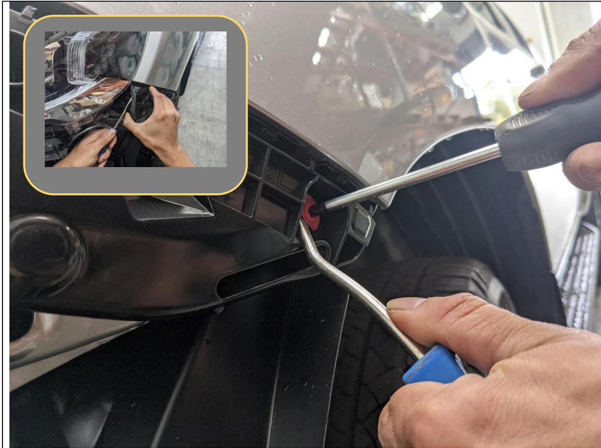
18. Remove the front bumper support plastic fasteners using trim tool and Phillips screwdriver to pry whilst loosening as shown.
