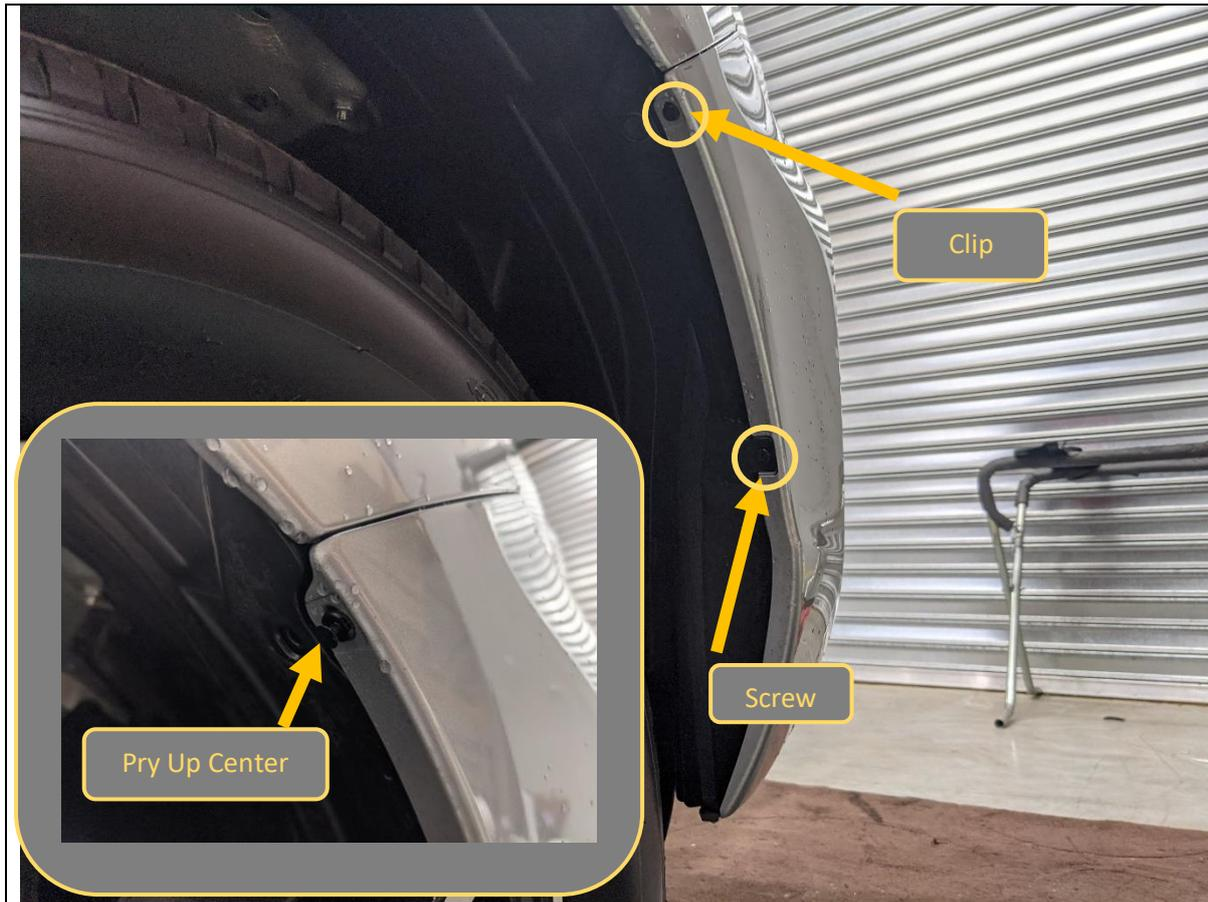
6. Remove the small screw and clip securing the bumper to the inner wheel arch liner.
