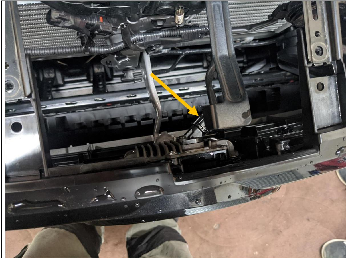
5. Unplug the radar sensor module wiring connector, located on the back of the Toyota Badge / sensor.
