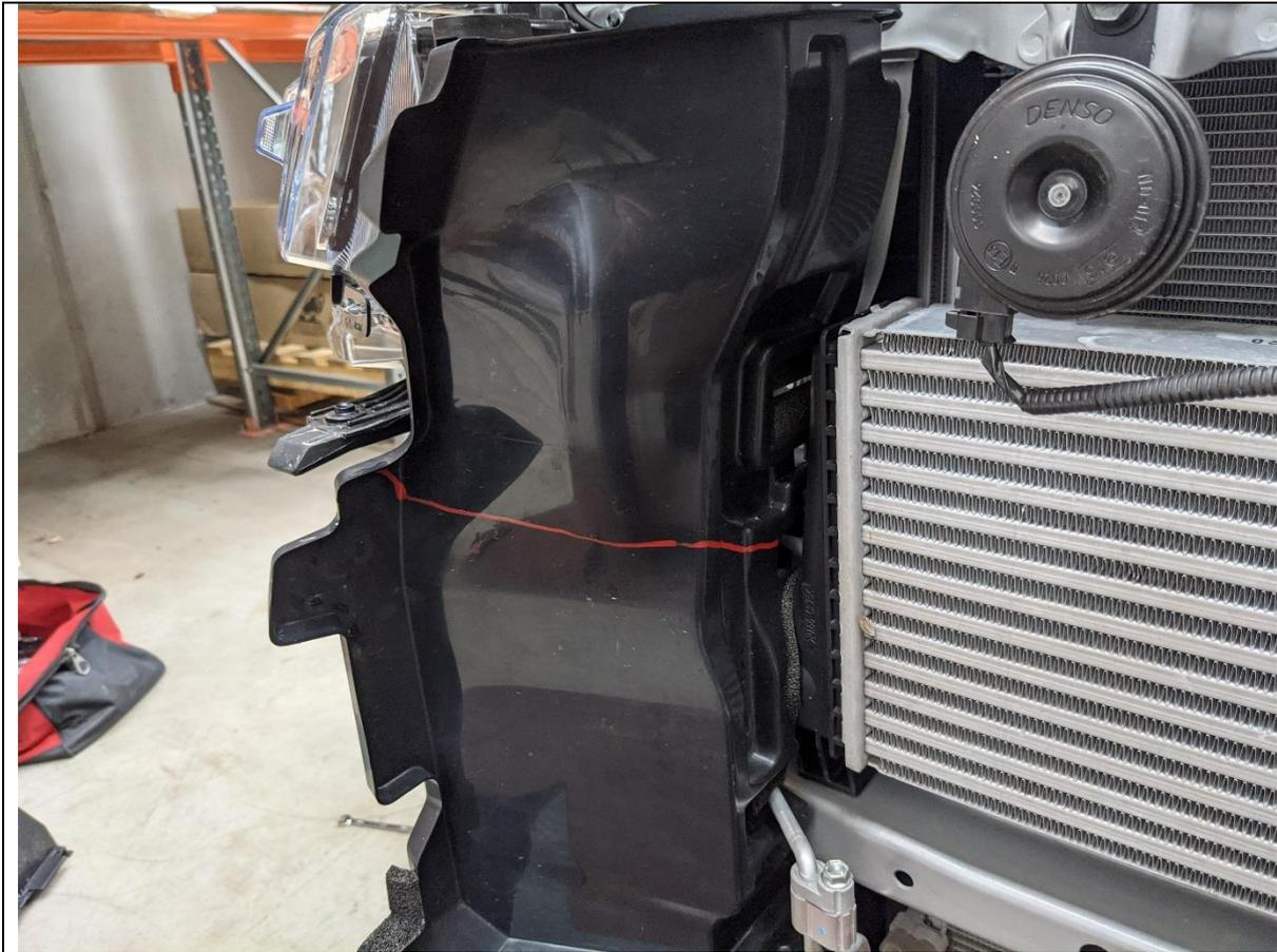
30. Mark air guide on Right hand side of vehicle as shown in the above image.
