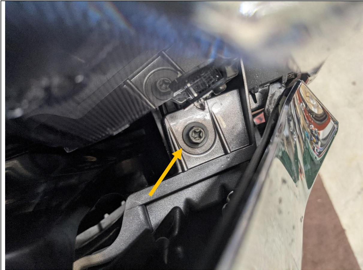
11. Remove the 2x 10mm Head/Phillips screws securing the bumper to crossmember.
