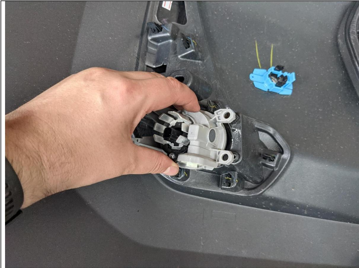
49. Remove the 3x Screws securing the fog lights to the bumper, then remove the fog light from the bumper
