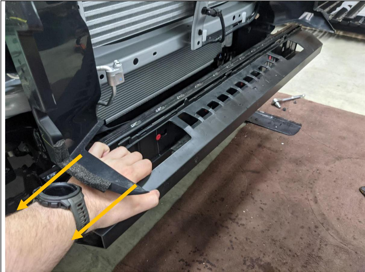
24. Remove the plastic cover from the impact beam by strongly pulling in the direction shown to release it from the clips
