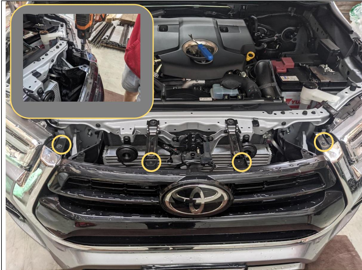
3. Remove the 4x 10mm Head screws securing the top of the grille
