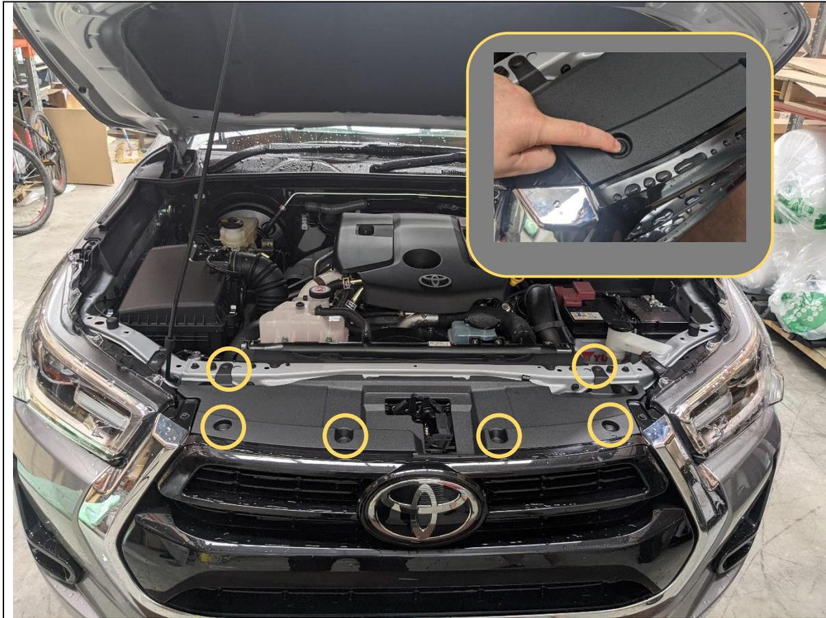
1. Remove the Radiator shroud by removing the 6x clips securing it to the grille and cross member.
