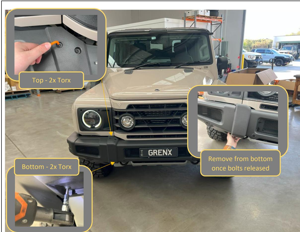
1. Park up vehicle in appropriate work location and remove the front number plate.
