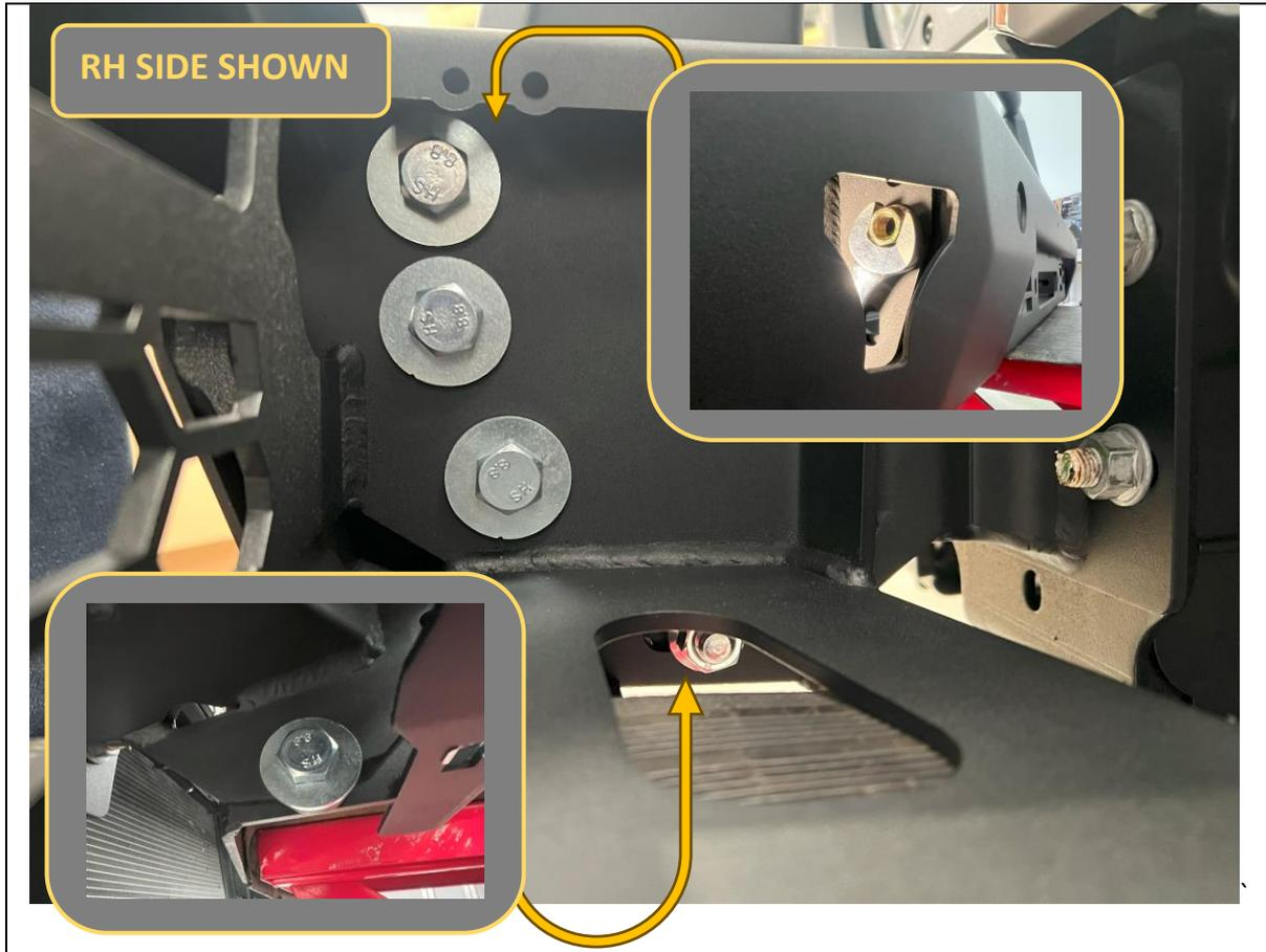
104. Secure with 4x M12x30 Bolts, Heavy Duty washers and M12 Nyloc and Flange Nuts per side, Finger tight at this stage.
