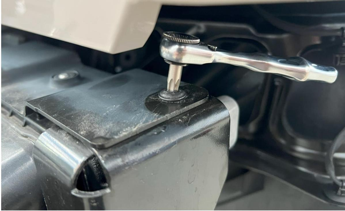
15. Once bumper panel is removed, replace the factory screw that secures the corner of the auxiliary radiator mounts.
