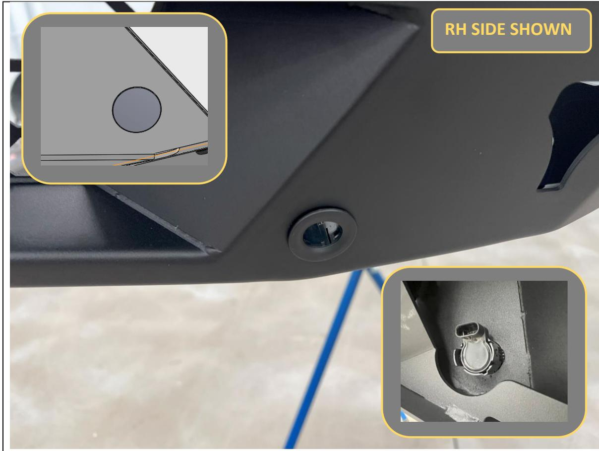
70. Re-fit the sensor housing and parking sensors to the bar.
