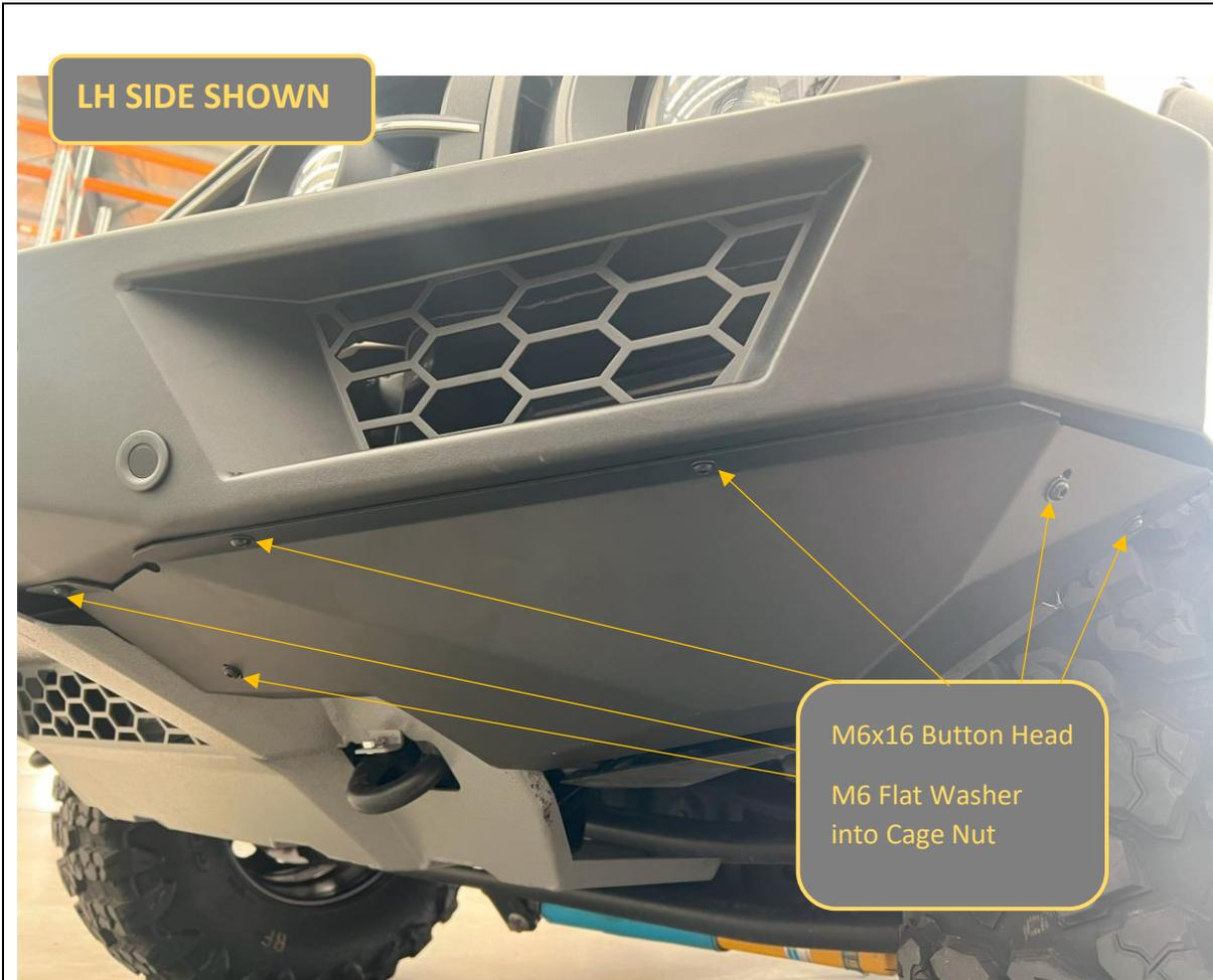
143. Fit Side Under panels using, 6x M6x16 button head and flat washer into the cage nuts placed earlier.
