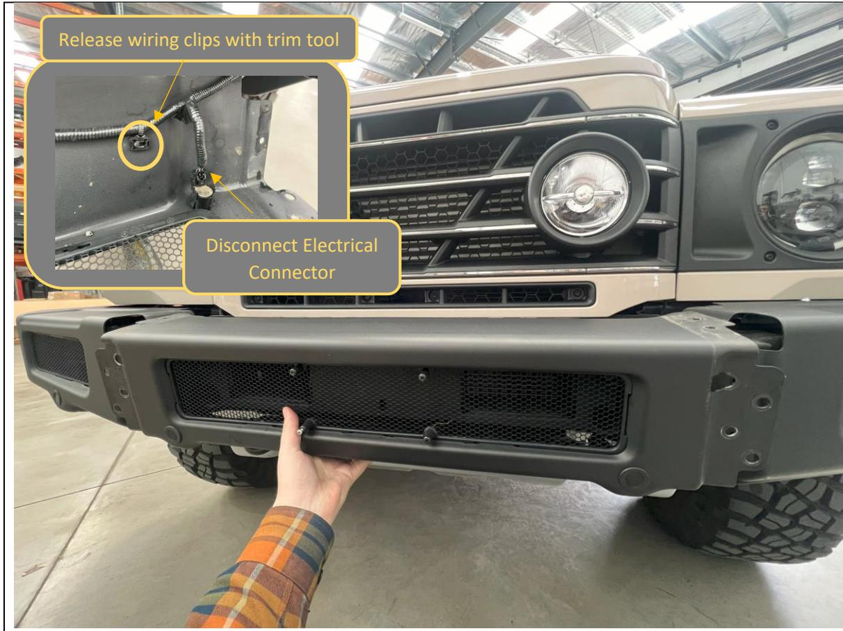
8. With all bolts removed, slide the center bumper panel forwards to remove.
