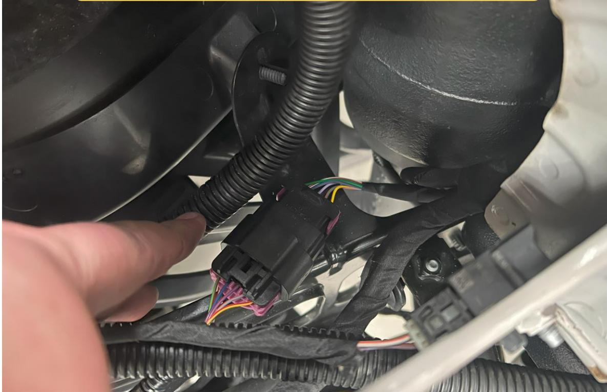
119. If Vehicle equipped with parking sensors. Re connect the main parking sensor loom behind the headlight. Remember to replace the retaining clip.
