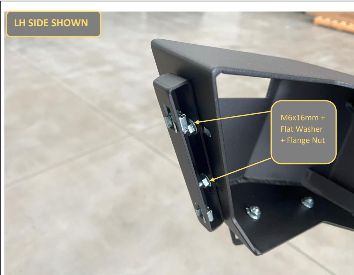
92. Fit the Inner Arch Liner Brackets to the slots in the back edge of the wing, using M6x16 Hex bolts, Flat Washers and Flange nuts. Leave finger tight at this stage
