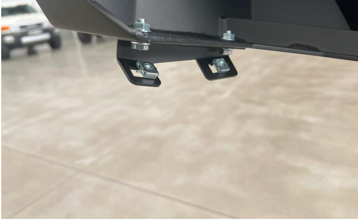
89. Fit the under-panel support brackets to the slots in the bottom edge of the wing, using M6x16 Hex bolts, Flat Washers and Flange nuts. Leave finger tight at this stage
