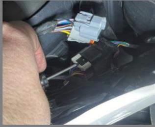
Use screwdriver to release retaining clip
