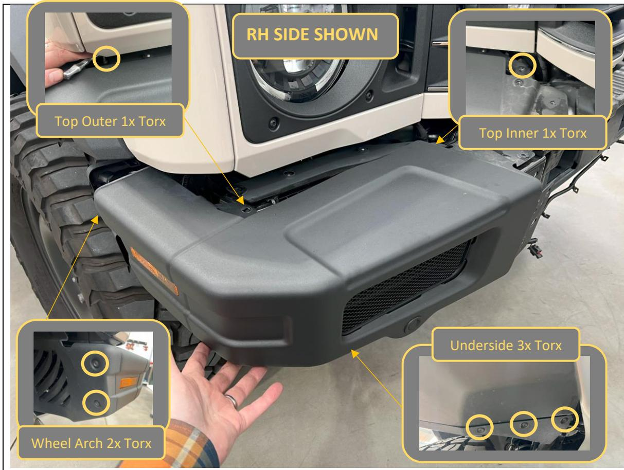
10. Remove Torx head screws retaining the outer bumper panel to the vehicle. Locations are shown in the image above.
