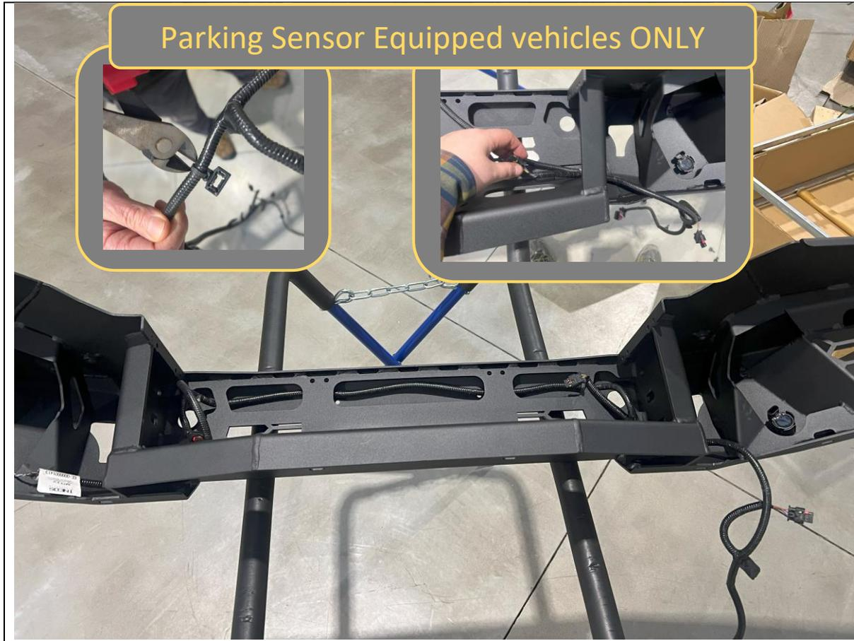
73. Before refitting the parking sensor loom, remove all the stud clips, by carefully cutting off using side cutters. This will make the loom much easier to run through the bar.
