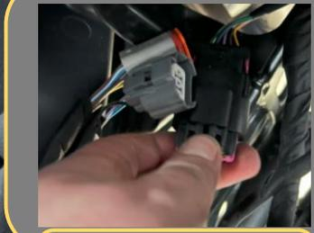
Squeeze tab and pull to disconnect
