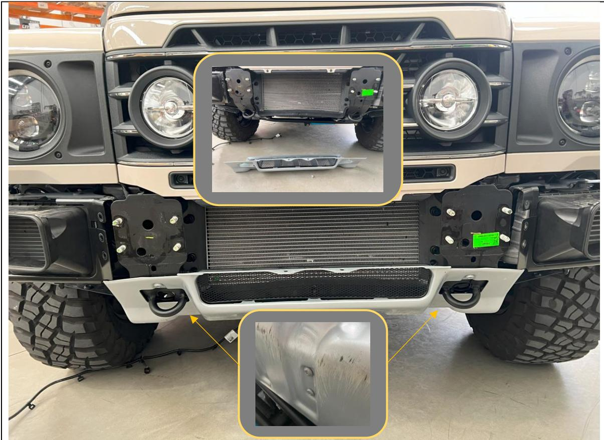
36. Remove the 2x T50 Torx screws securing the top of the bash plate to the chassis.
