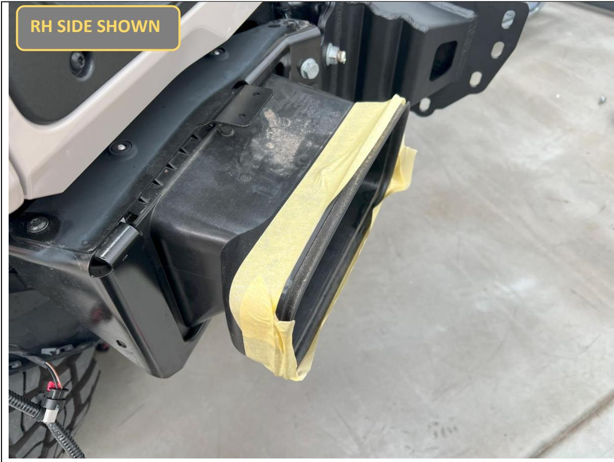
43. Cover the outer section of the plastic aux radiator air guides with masking tape, as shown.
