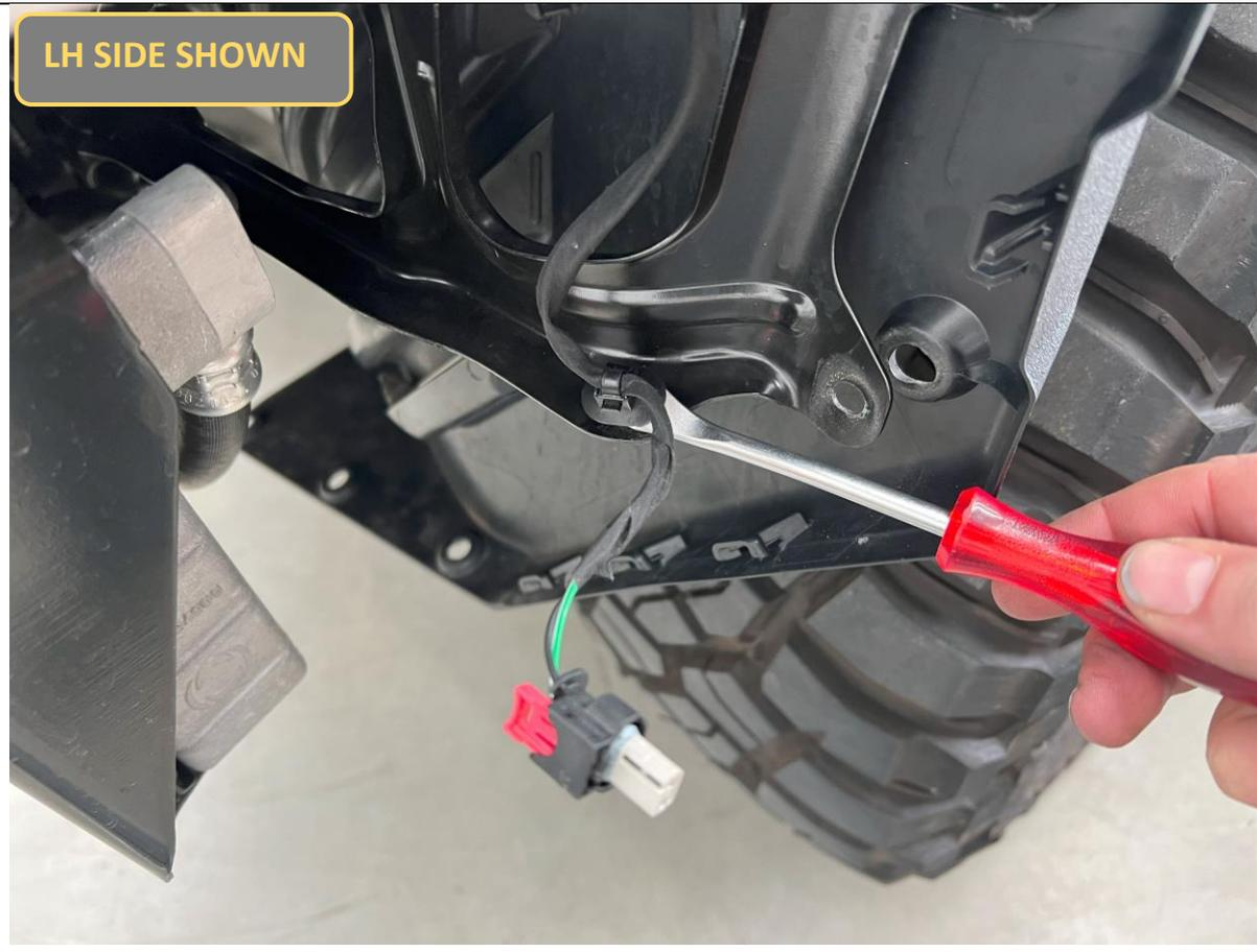
29. Unclip the clearance light harness from the wheel arch bracket.
