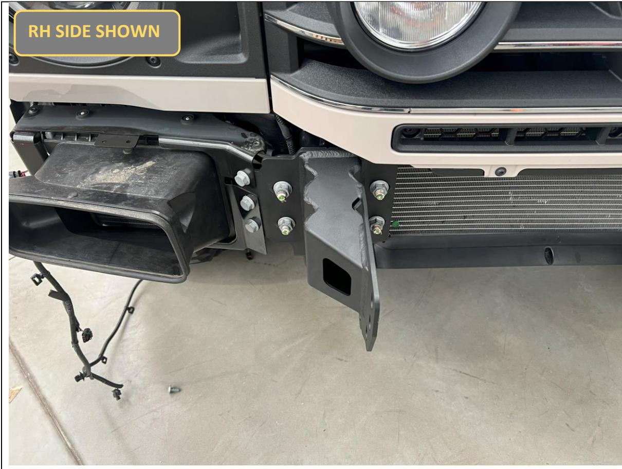
39. Secure the impact assembly to the chassis and auxiliary radiator bracket, re-using the factory bolts and flange nuts removed from the impact beam.
