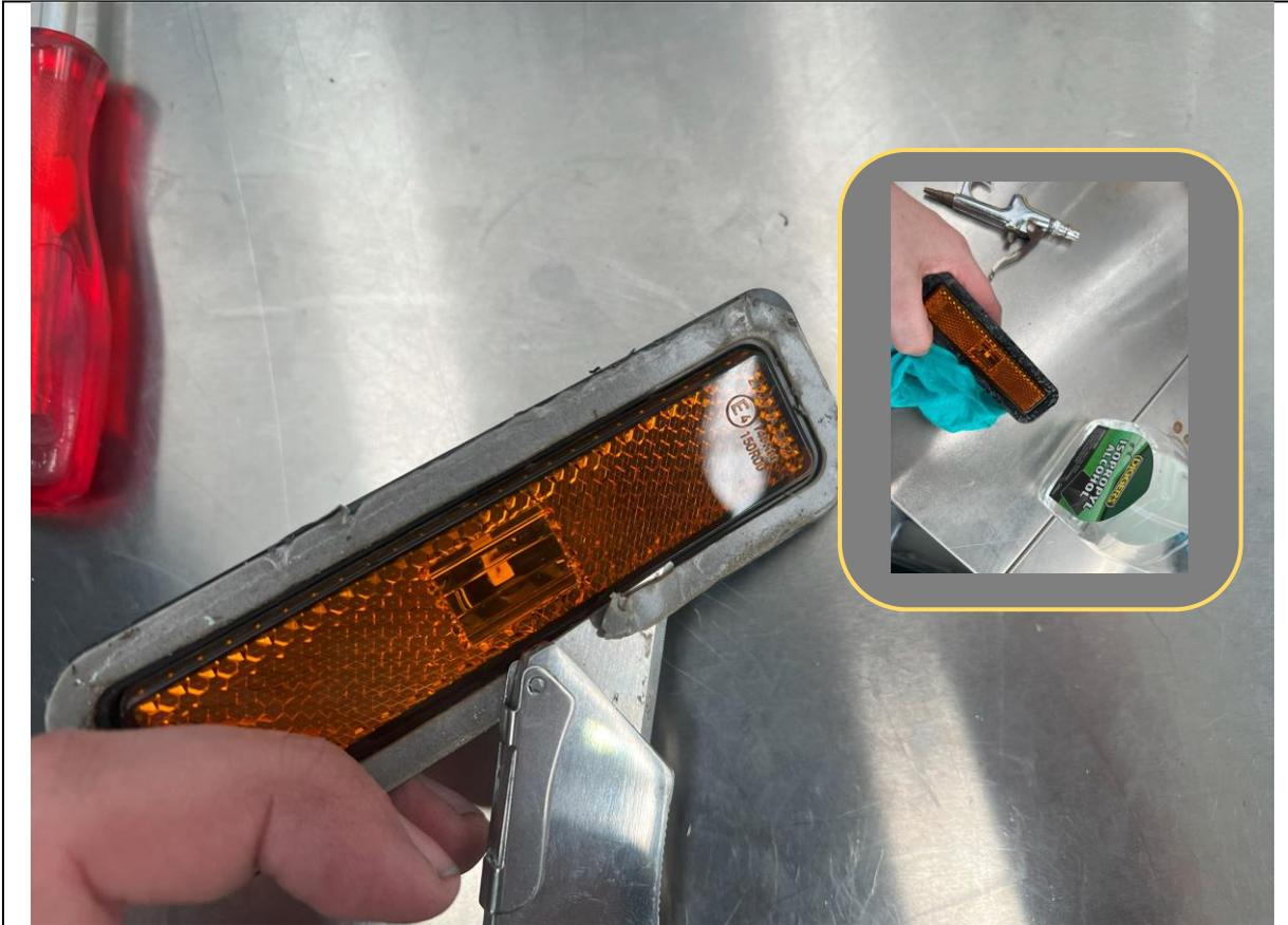
54. Remove all adhesive, and adhesive residue from the clearance lights.
