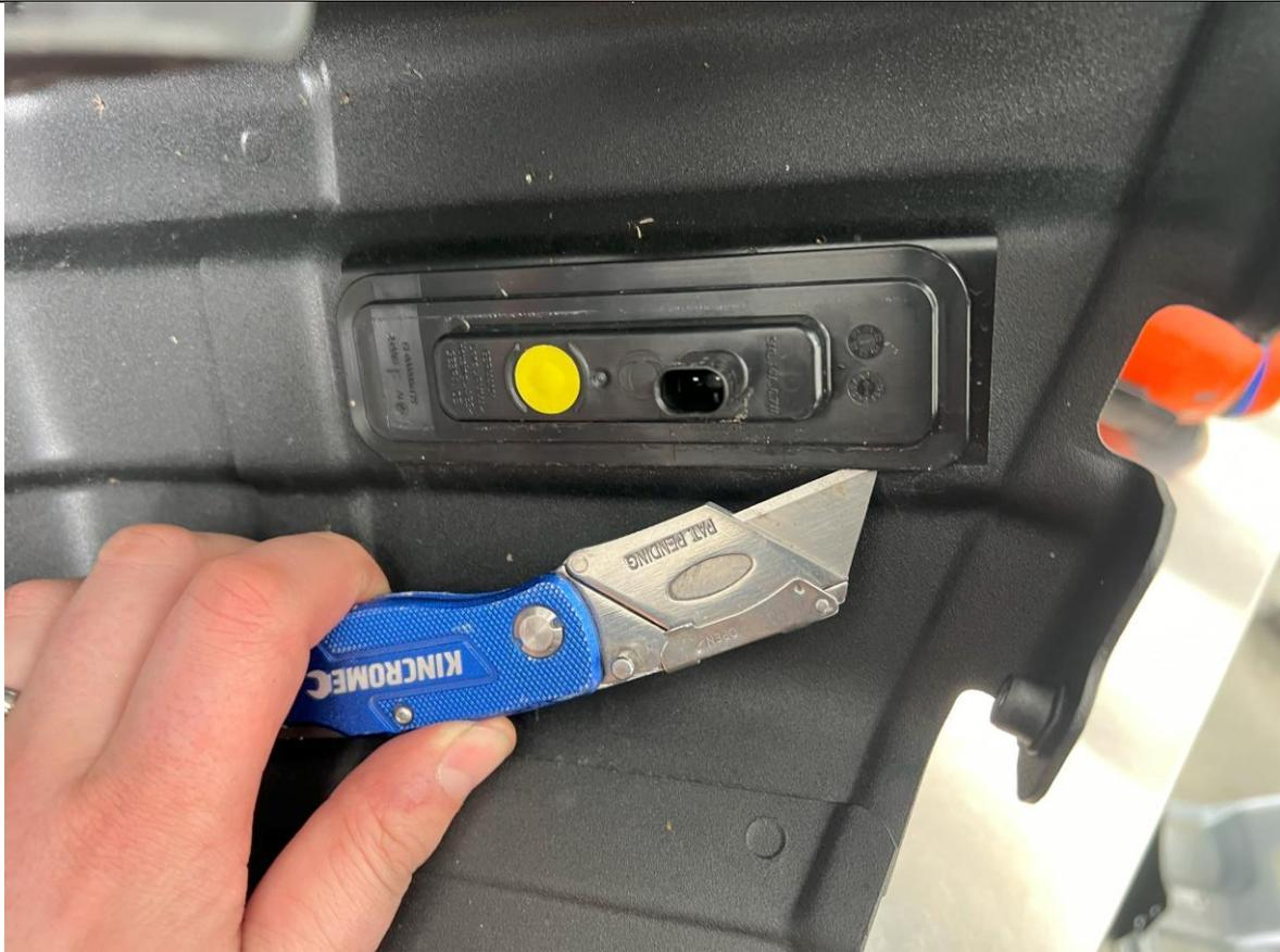
51. Remove the marker lamps from the outer bumper panels. Use a sharp utility knife to cut the tape, then gently use a trim tool to pry the light out.
